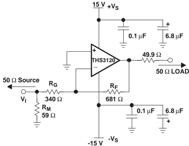
Figure 48. Wideband, Inverting Gain Configuration
