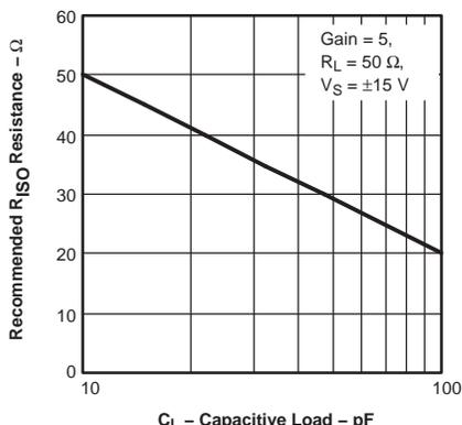
Figure 51. Recommended R<sub>ISO</sub> vs Capacitive Load
