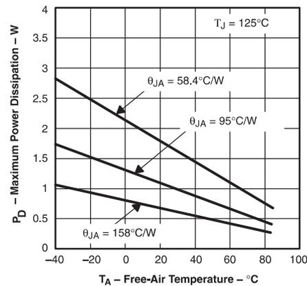
Results are With No Air Flow and PCB Size = 3 inches x 3 inches (76,2 mm x 76,2 mm)
