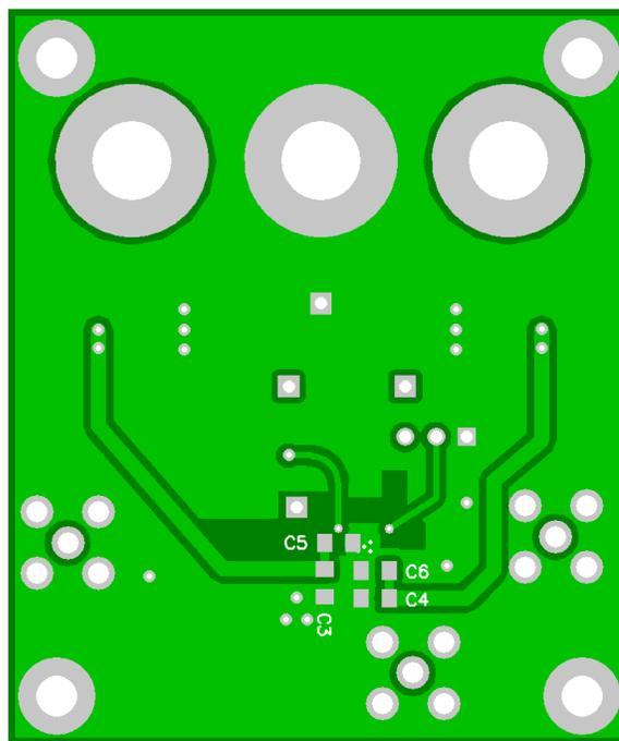
Figure 64. THS3120 EVM Board Layout (Bottom Layer)
