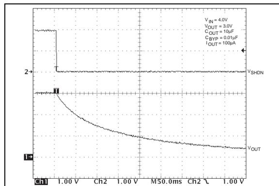
FIGURE 2-17: Shutdown Delay.
