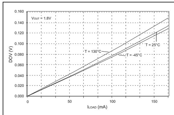
**FIGURE 2-6:** Dropout Voltage vs.  $I_{LOAD}$ .
