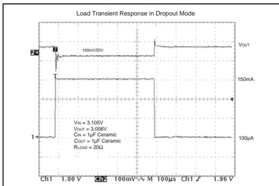
FIGURE 2-14: Load Transient Response in Dropout Mode.
