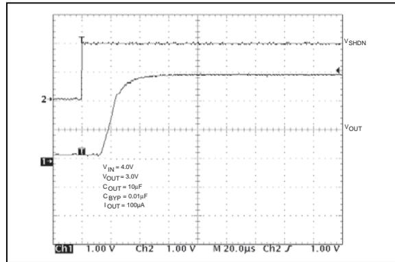
FIGURE 2-18: Shutdown Wake-up Time.
