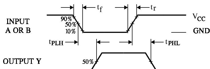
**Figure 1. Switching Waveforms**
