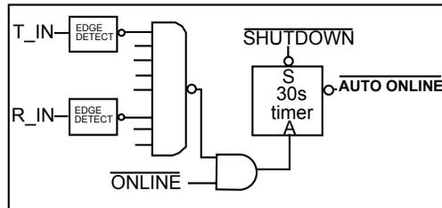
Figure 3c. Auto On-line<sup>®</sup> Plus Logic
