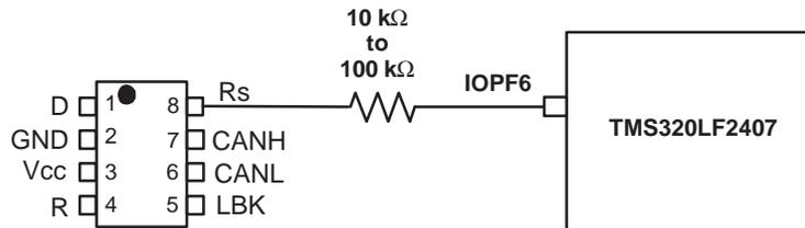
Figure 30. Slope Control/Standby Connection to a DSP
