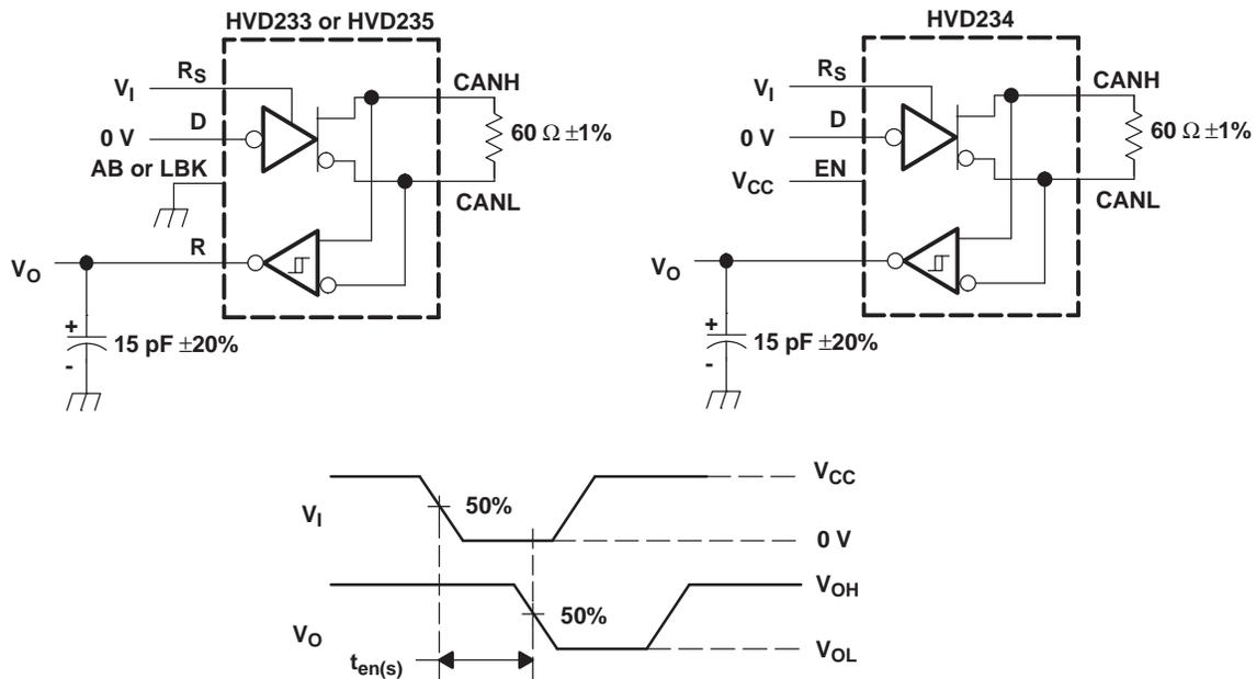
NOTE: All  $V_I$  input pulses are supplied by a generator having the following characteristics:  $t_r$  or  $t_f \leq 6$  ns, pulse repetition rate (PRR) = 125 kHz, 50% duty cycle.
