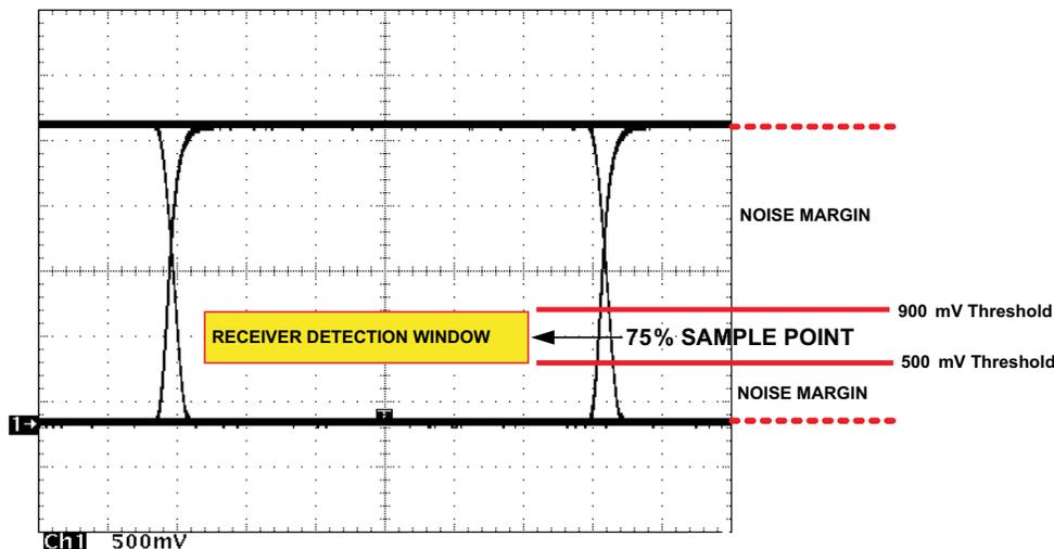
Figure 29. Typical SN65HVD230 Differential Output Voltage Waveform
