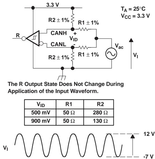
NOTE: All input pulses are supplied by a generator with  $f \leq 1.5\text{ MHz}$ .
