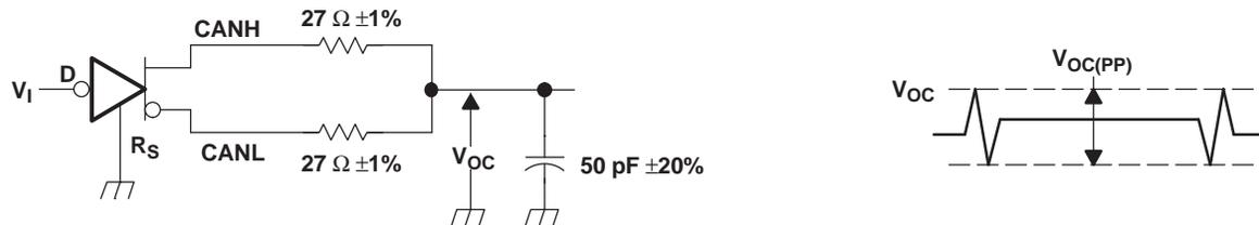
NOTE: All  $V_I$  input pulses are supplied by a generator having the following characteristics:  $t_r$  or  $t_f \leq 6$  ns, pulse repetition rate (PRR) = 125 kHz, 50% duty cycle.
