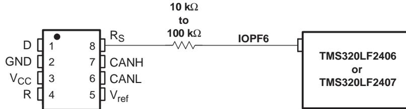
Figure 32. Slope Control/Standby Connection to a DSP
