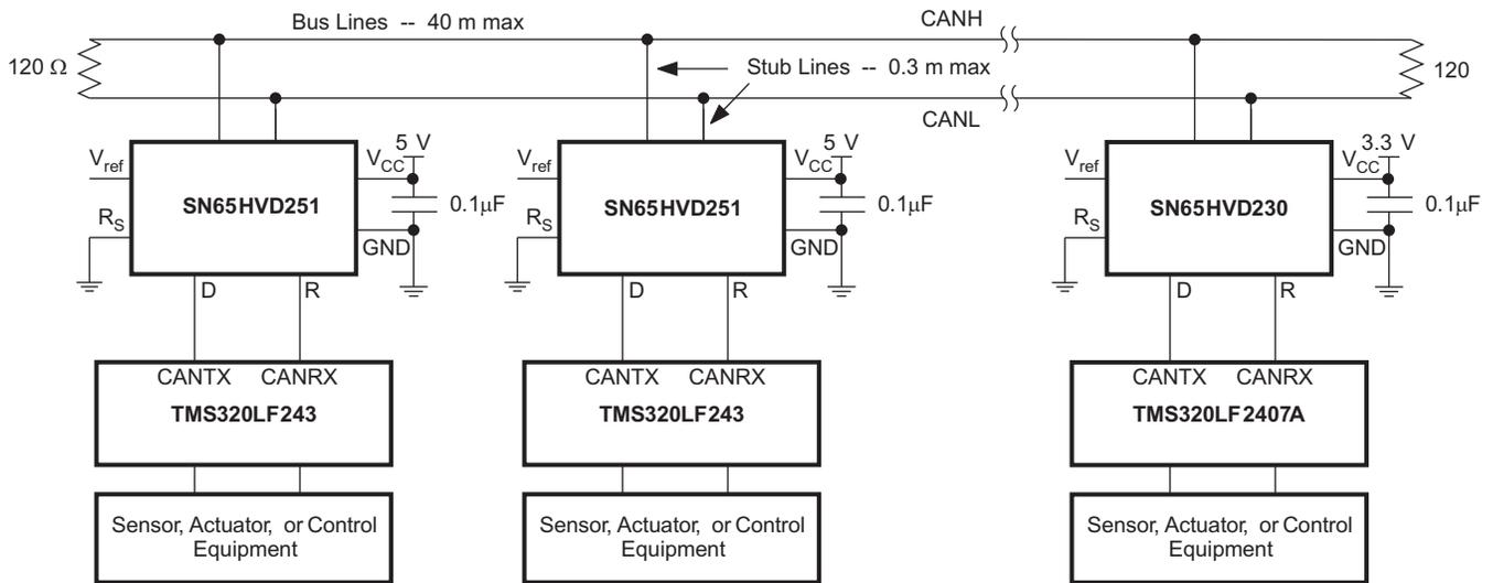
Figure 37. 3.3-V and 5-V CAN Transceiver System
