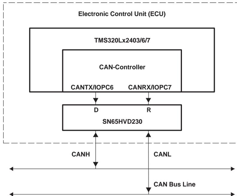
Figure 28. Details of a Typical CAN Node
