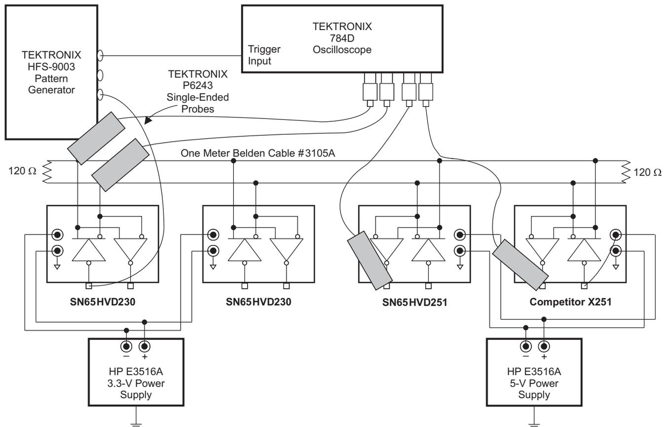
Figure 38. 3.3-V and 5-V CAN Transceiver System Testing
