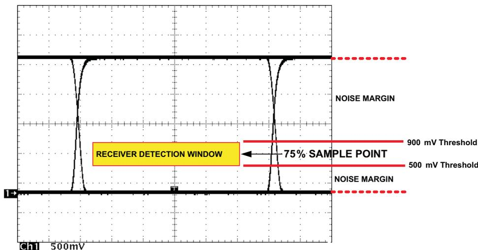
Figure 36. Typical SN65HVD230 Differential Output Voltage Waveform
