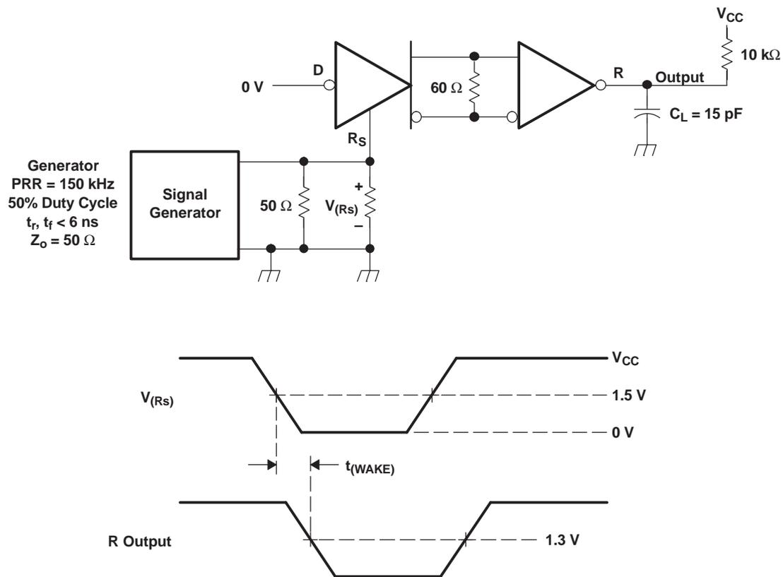
Figure 8.  $t_{(WAKE)}$  Test Circuit and Voltage Waveforms
