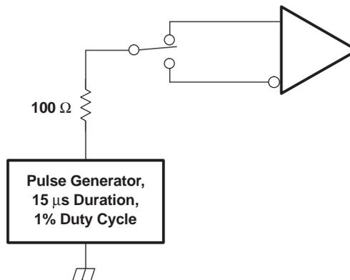
Figure 7. Overvoltage Protection
