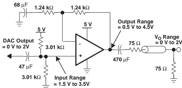
Figure 42. AC-Coupled Wide Output Swing Single-Supply Video Amplifier
