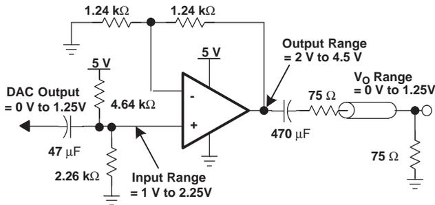
Figure 41. AC-Coupled Input and Output Single-Supply Video Amplifier
