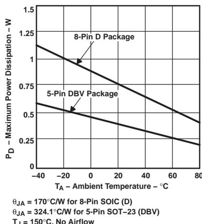
**Figure 46. Maximum Power Dissipation vs Ambient Temperature**
