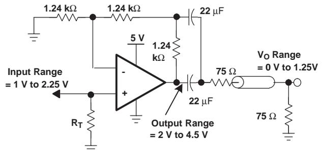
Figure 40. AC-Coupled SAG Corrected Output Single-Supply Video Amplifier
