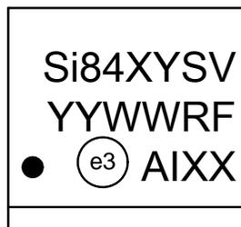
Figure 22. 8-Pin Narrow Body SOIC Top Marking
