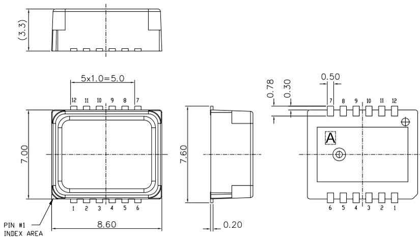
Figure 3. Housing dimensions
