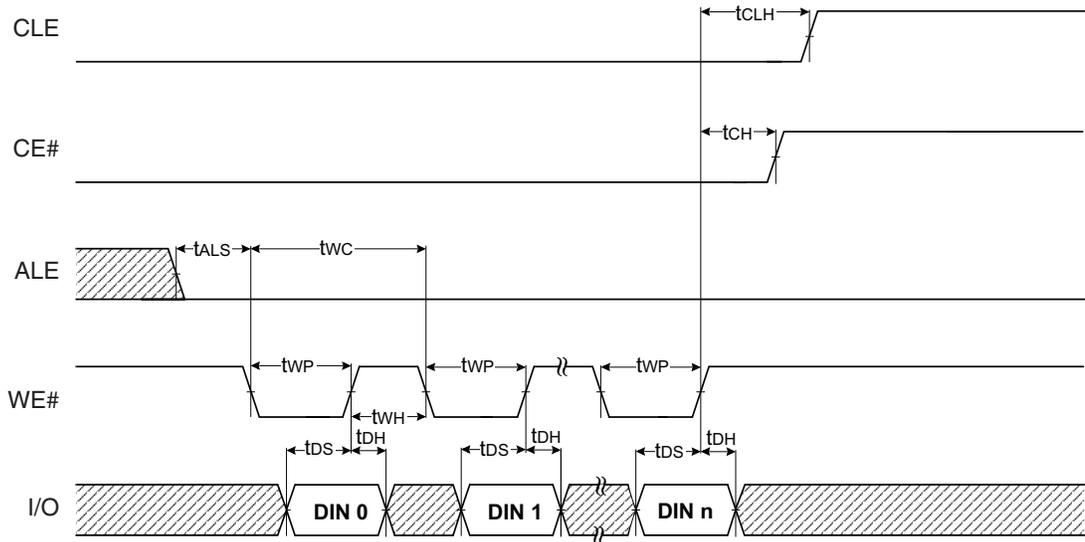
Figure 7.4 Sequential Data Out Cycle Timing Diagram (CLE = Low, ALE = Low, WE# = High)
