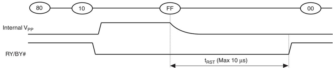
**Figure 10.10** Reset (FFh) Command Input During Erasing
