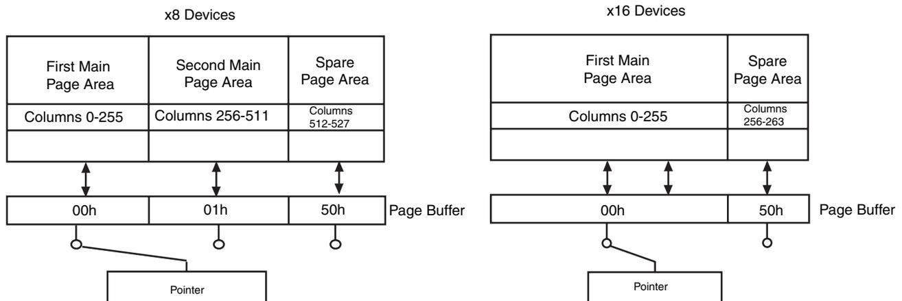
**Figure 10.2** Pointer Operations for Programming
