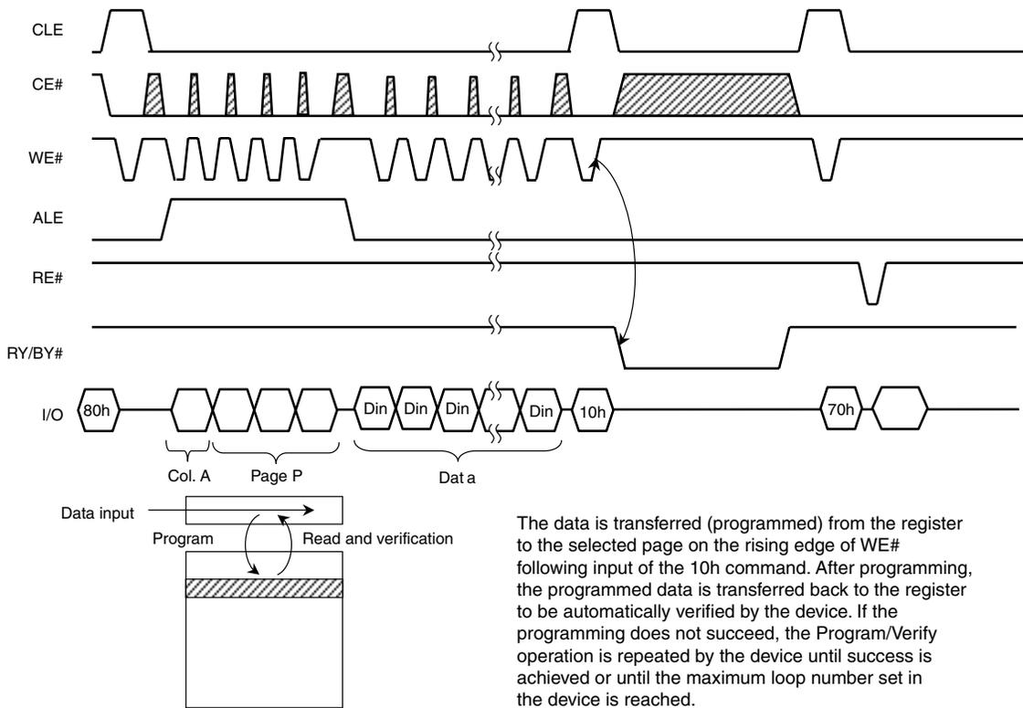
Once the serial input 80h command has been input, do not input any command other than 10h related to programming and FFh related to reset. If a command other than 10h, FFh is input into the device, the program operation will not be performed.
