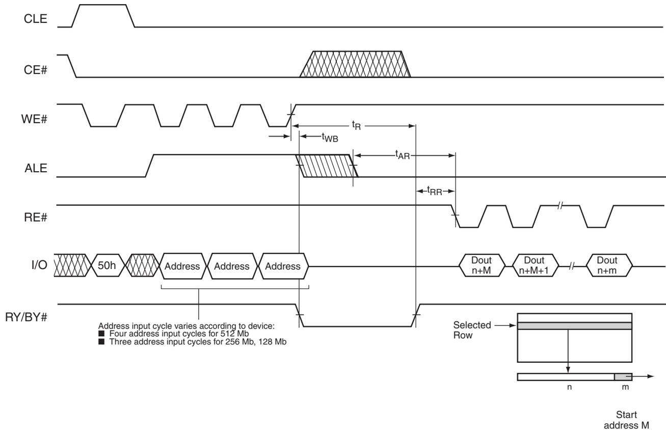
Figure 7.8 Page Program Timing Diagram
