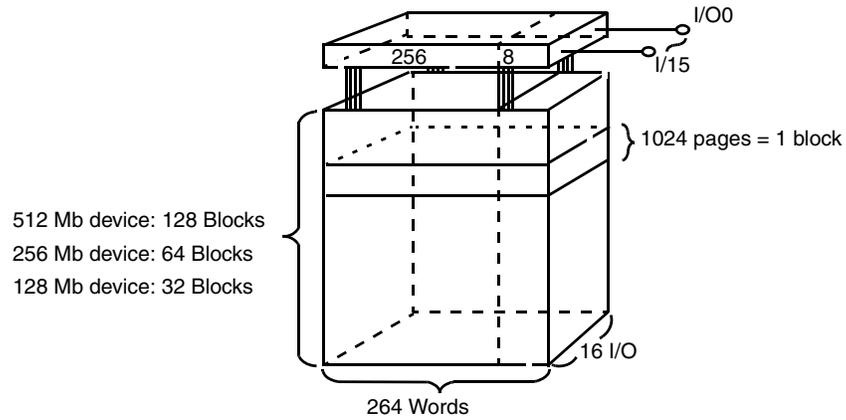
A page consists of 264 Words in which 256 Words are used for main memory storage and 8 Words are reserved for redundancy or other usage.
