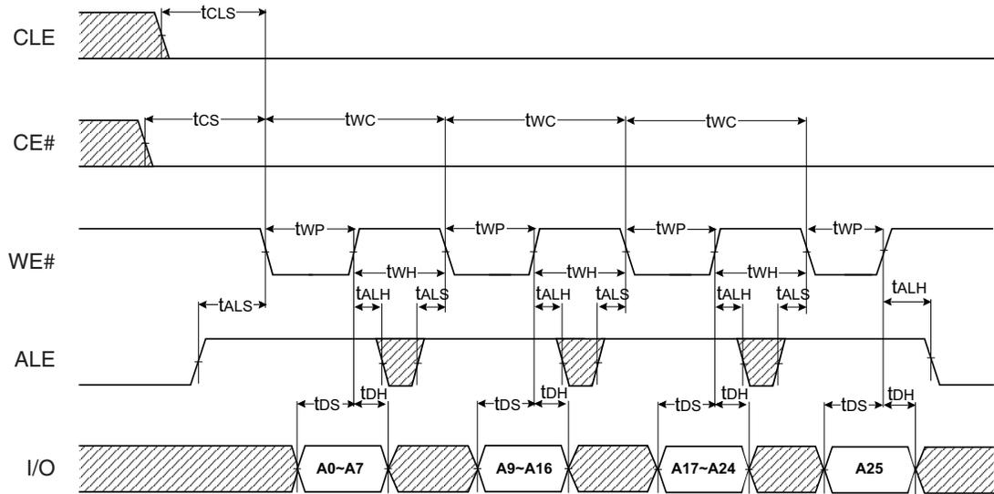
Figure 7.3 Input Data Latch Cycle Timing Diagram
