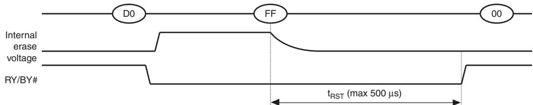
**Figure 10.11** Reset (FFh) Command Input During a Read Operation
