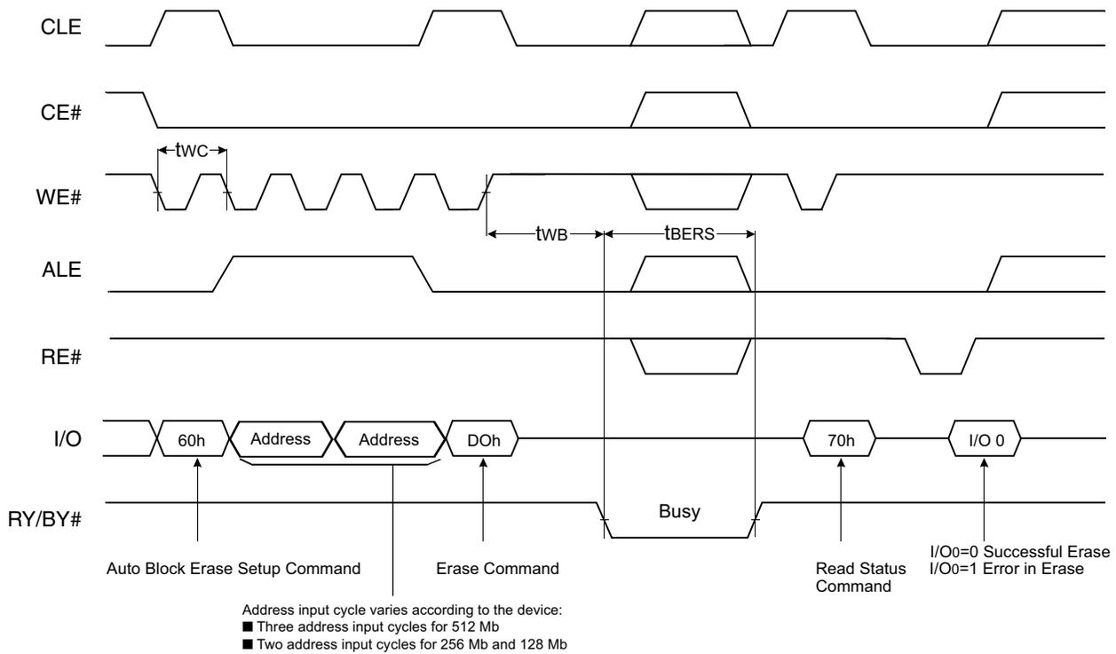
Figure 7.11 Spansion Command Mode Entry Timing Diagram
