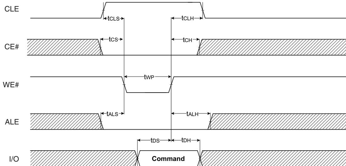
Figure 7.2 Address Latch Cycle Timing Diagram
