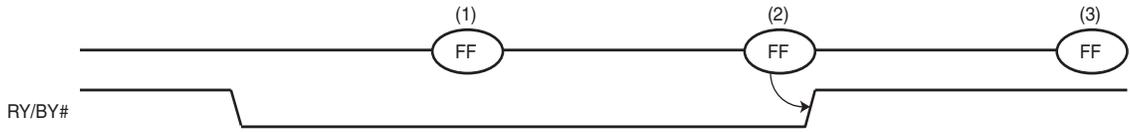
The second Reset command is invalid since the device has not internally completed the first Reset command.
