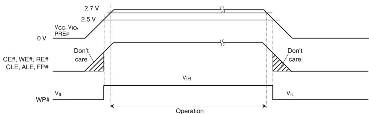
After power-on, access the device only after the RY/BY# pin indicates the device is ready. Do not issue any commands to the device while RY/BY# is busy.
