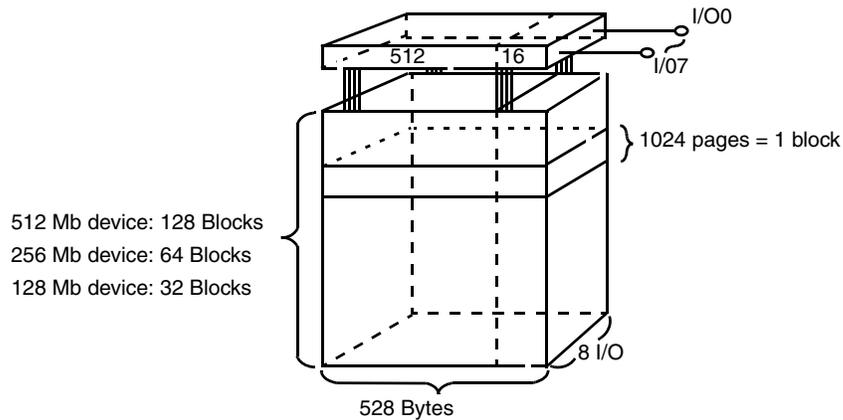
A page consists of 528 Bytes in which 512 Bytes are used for main memory storage and 16 Bytes are reserved for redundancy or other usage.
