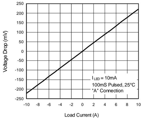
Figure 3. Linearity Characteristics
