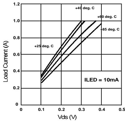
Figure 3. Typical On-Characteristics
