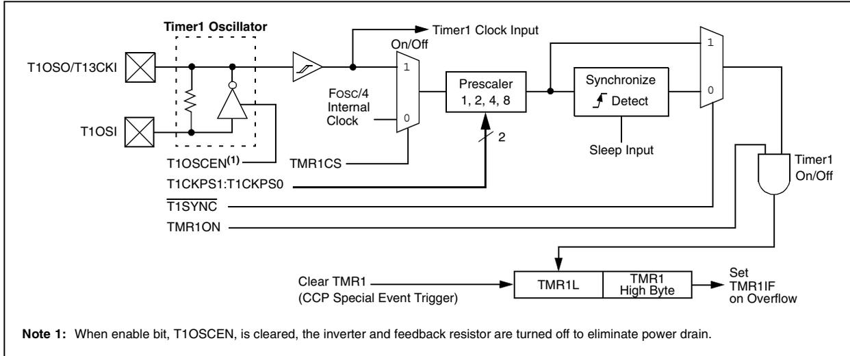
**FIGURE 11-2: TIMER1 BLOCK DIAGRAM (16-BIT READ/WRITE MODE)**
