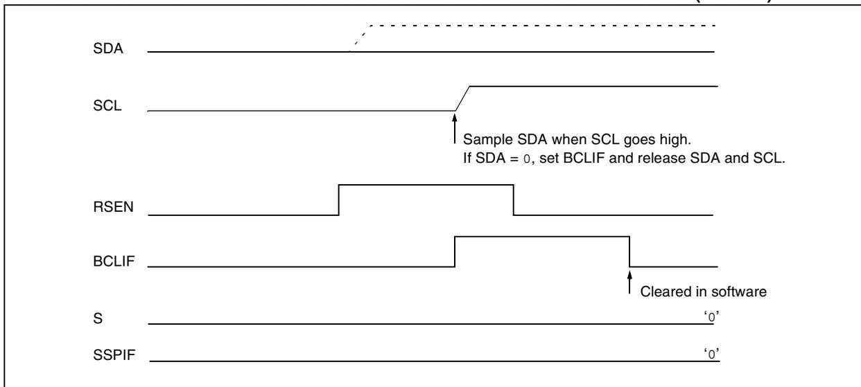
**FIGURE 16-32: BUS COLLISION DURING REPEATED START CONDITION (CASE 2)**
