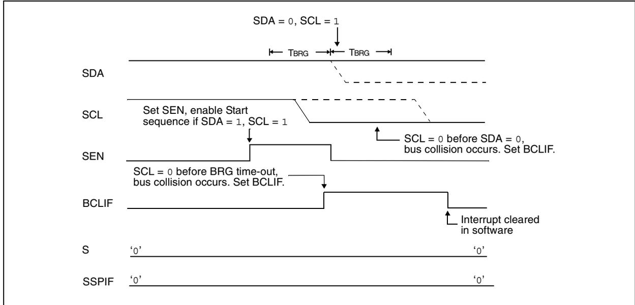
**FIGURE 16-30: BRG RESET DUE TO SDA ARBITRATION DURING START CONDITION**
