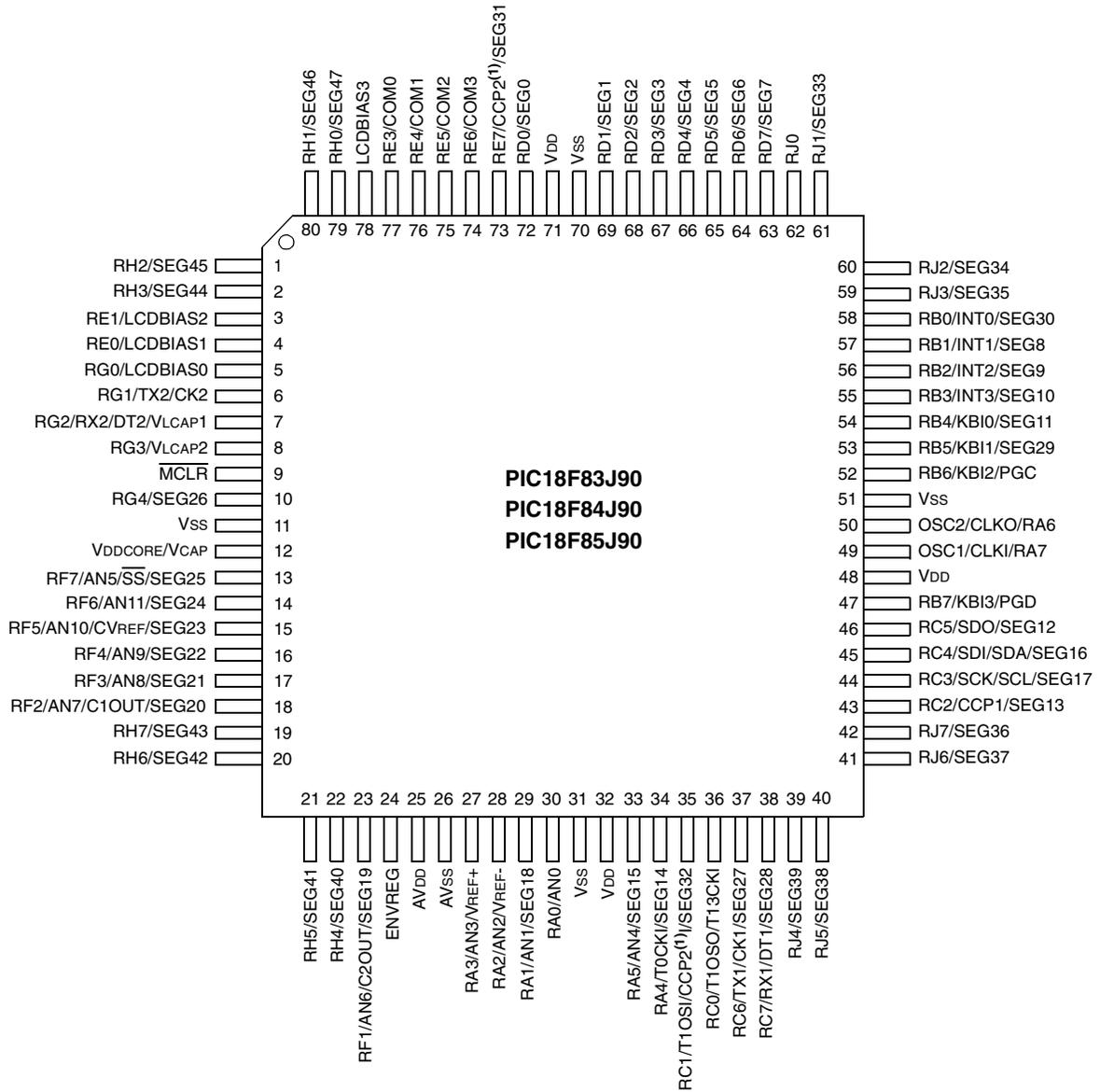
**Note 1:** The CCP2 pin placement depends on the CCP2MX bit setting.
