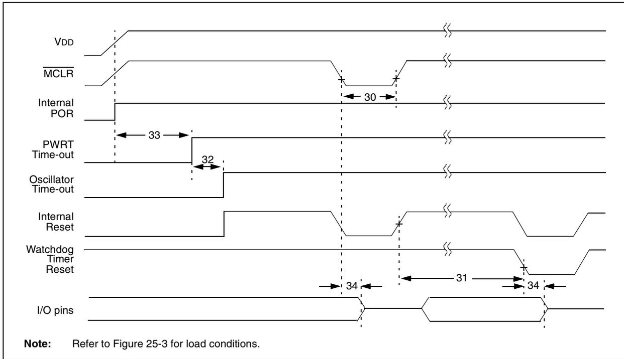
**TABLE 25-11: RESET, WATCHDOG TIMER, OSCILLATOR START-UP TIMER, POWER-UP TIMER AND BROWN-OUT RESET REQUIREMENTS**
