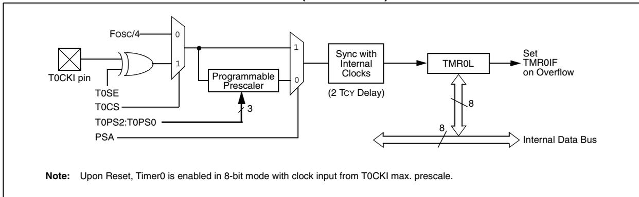
**FIGURE 10-2: TIMER0 BLOCK DIAGRAM (16-BIT MODE)**
