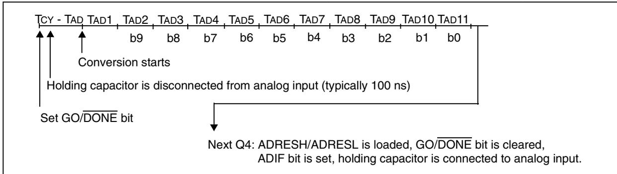
**FIGURE 19-4: A/D CONVERSION TAD CYCLES (ACQT2:ACQT0 = 010, TACQ = 4 TAD)**
