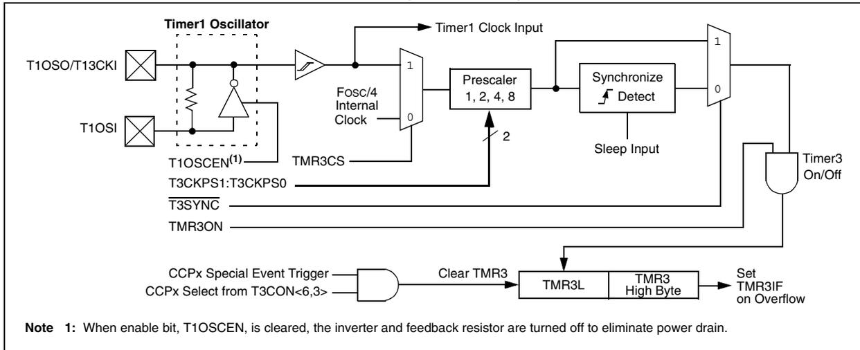
**FIGURE 13-2: TIMER3 BLOCK DIAGRAM (16-BIT READ/WRITE MODE)**
