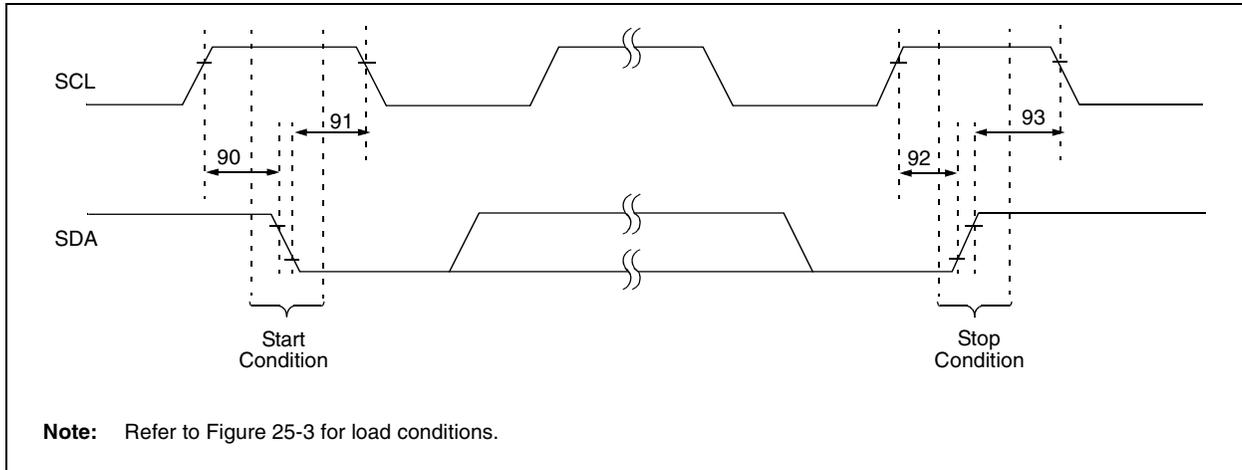
**TABLE 25-20: MSSP I<sup>2</sup>C™ BUS START/STOP BITS REQUIREMENTS**
