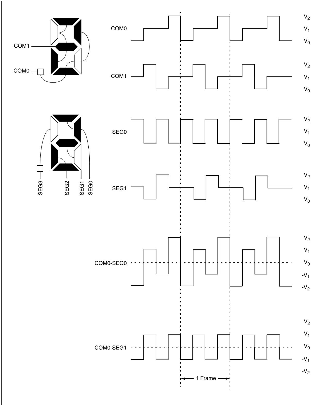
**FIGURE 15-8: TYPE-B WAVEFORMS IN 1/2 MUX, 1/2 BIAS DRIVE**
