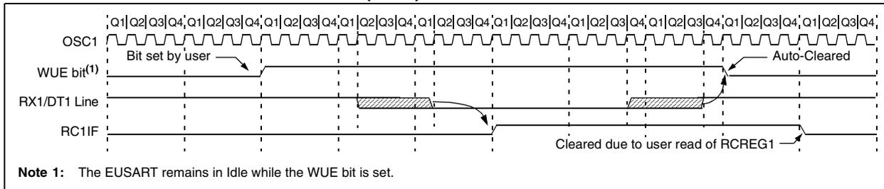
**FIGURE 17-9: AUTO-WAKE-UP BIT (WUE) TIMINGS DURING SLEEP**
