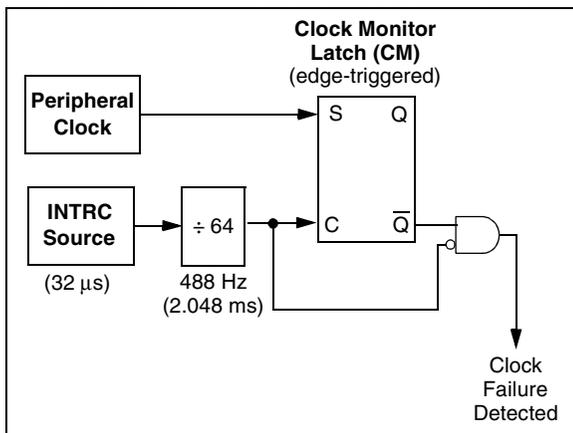
Clock failure is tested for on the falling edge of the sample clock. If a sample clock falling edge occurs while CM is still set, a clock failure has been detected (Figure 22-5). This causes the following:
