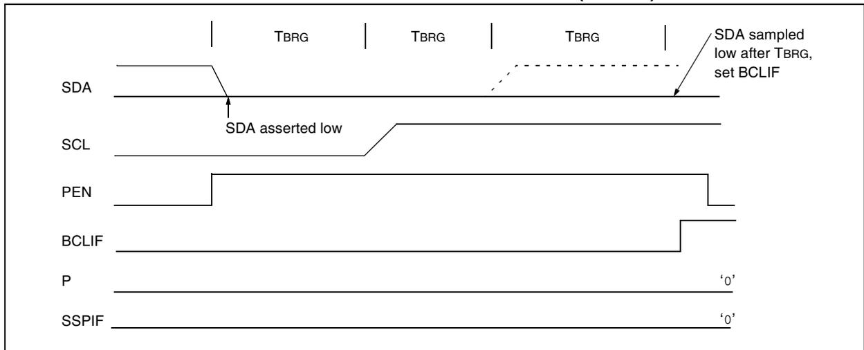
**FIGURE 16-34: BUS COLLISION DURING A STOP CONDITION (CASE 2)**
