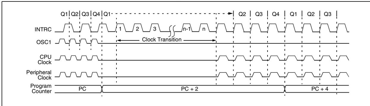
**FIGURE 3-4: TRANSITION TIMING FROM RC\_RUN MODE TO PRI\_RUN MODE**
