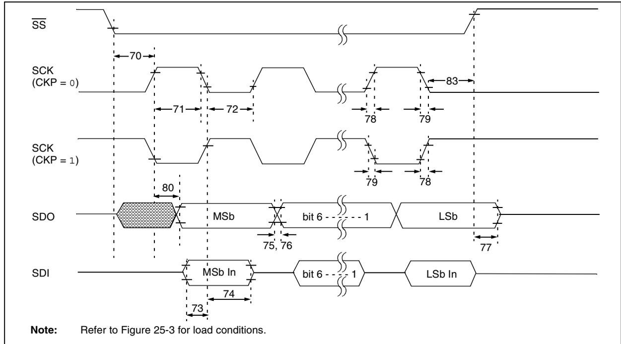
**TABLE 25-16: EXAMPLE SPI MODE REQUIREMENTS (SLAVE MODE TIMING, CKE = 0)**
