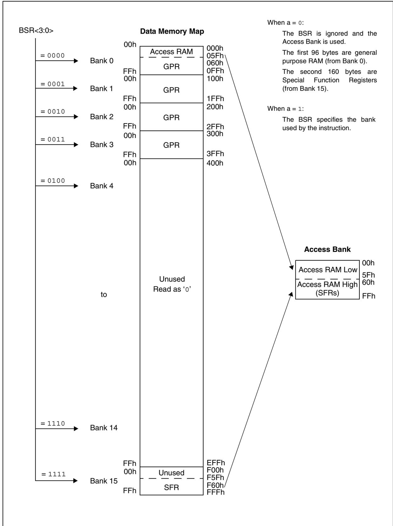
**FIGURE 5-8: USE OF THE BANK SELECT REGISTER (DIRECT ADDRESSING)**
