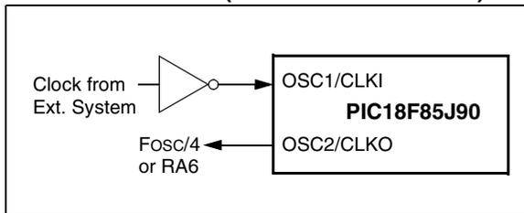
An external clock source may also be connected to the OSC1 pin in the HS mode, as shown in Figure 2-4. In this configuration, the divide-by-4 output on OSC2 is not available.
