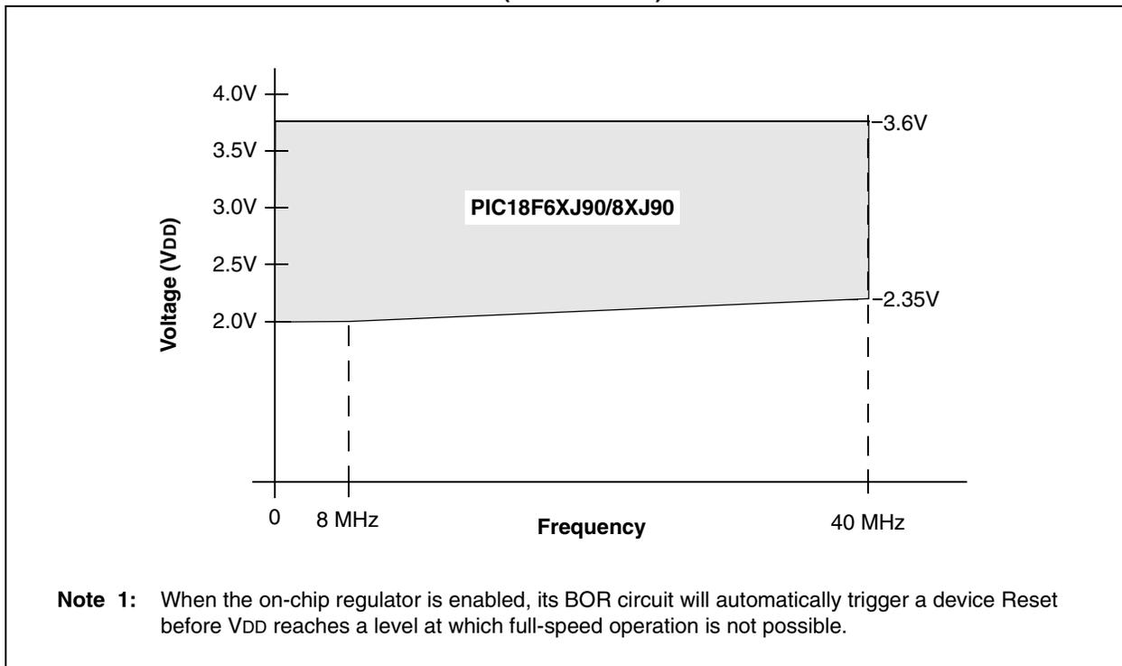
**FIGURE 25-2: PIC18F85J90 FAMILY VOLTAGE-FREQUENCY GRAPH, REGULATOR DISABLED (INDUSTRIAL)<sup>(1,2)</sup>**
