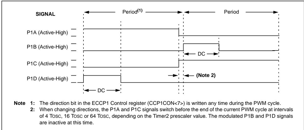
**FIGURE 18-9: PWM DIRECTION CHANGE AT NEAR 100% DUTY CYCLE<sup>(1)</sup>**
