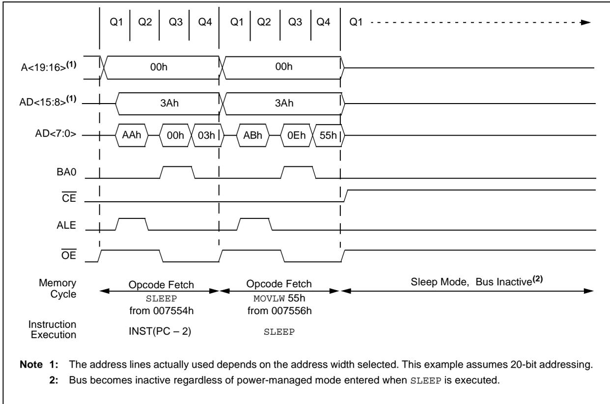
**FIGURE 7-11: TYPICAL OP CODE FETCH, 8-BIT MODE**
