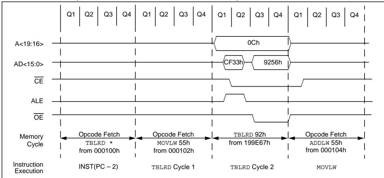
**FIGURE 7-6: EXTERNAL MEMORY BUS TIMING FOR SLEEP (MICROPROCESSOR MODE)**
