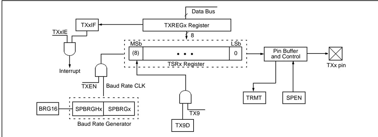
**FIGURE 20-4: ASYNCHRONOUS TRANSMISSION**
