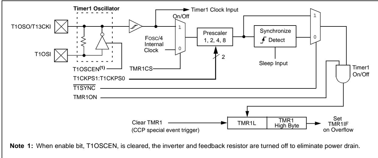
**FIGURE 13-2: TIMER1 BLOCK DIAGRAM (16-BIT READ/WRITE MODE)**
