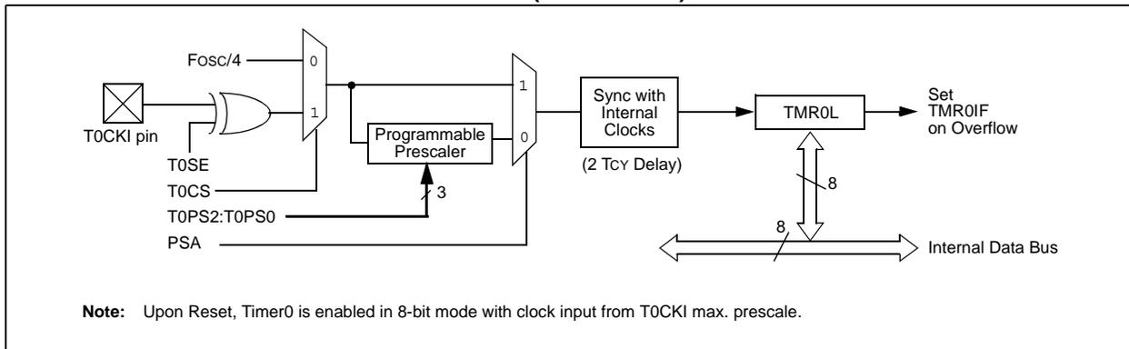
**FIGURE 12-2: TIMER0 BLOCK DIAGRAM (16-BIT MODE)**
