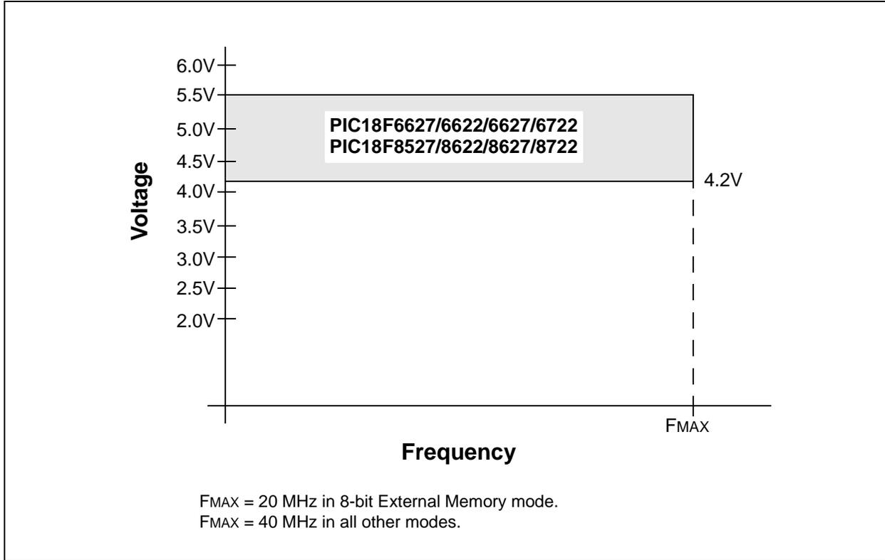
FIGURE 28-2: PIC18F8722 DEVICE FAMILY VOLTAGE-FREQUENCY GRAPH (EXTENDED)
