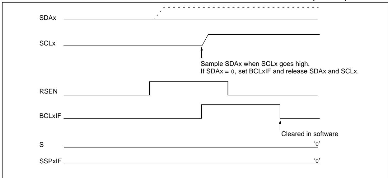
**FIGURE 19-30: BUS COLLISION DURING REPEATED START CONDITION (CASE 2)**
