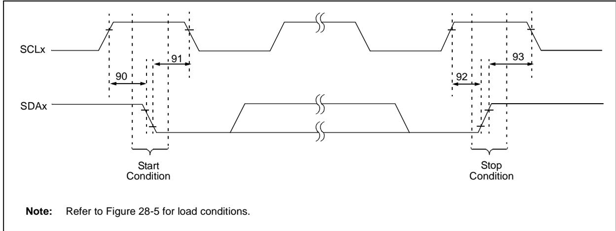
**TABLE 28-22: MASTER SSP I<sup>2</sup>C™ BUS START/STOP BITS REQUIREMENTS**
