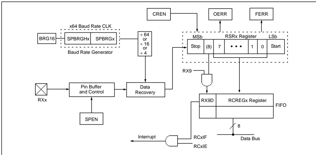
**FIGURE 20-7: ASYNCHRONOUS RECEPTION**
