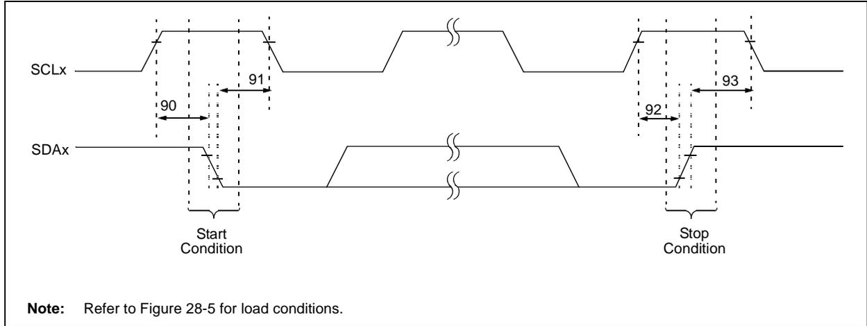
**TABLE 28-20: I<sup>2</sup>C™ BUS START/STOP BITS REQUIREMENTS (SLAVE MODE)**
