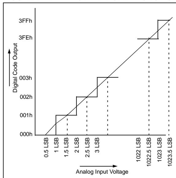
**FIGURE 21-3: ANALOG INPUT MODEL**
