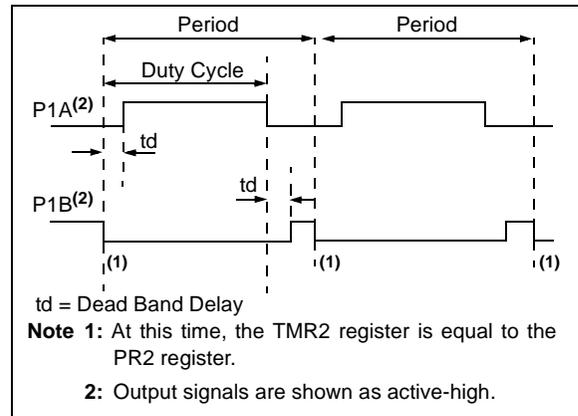
**FIGURE 18-5: EXAMPLES OF HALF-BRIDGE OUTPUT MODE APPLICATIONS**
