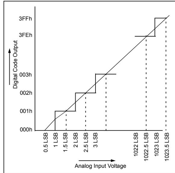
**FIGURE 19-3: ANALOG INPUT MODEL**
