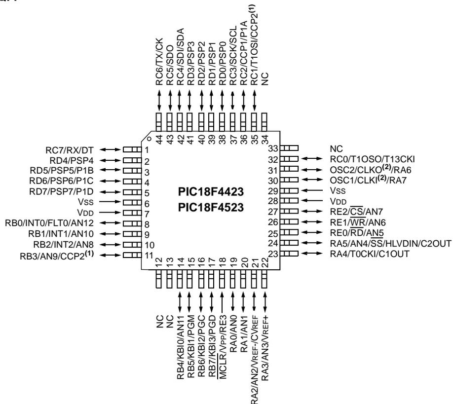
**Note 1:** RB3 is the alternate pin for CCP2 multiplexing.
