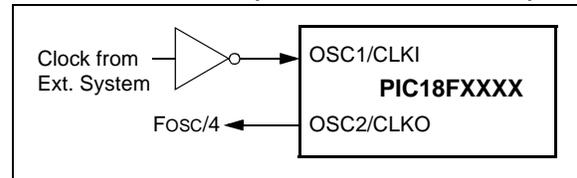
The ECIO Oscillator mode functions like the EC mode, except that the OSC2 pin becomes an additional general purpose I/O pin. The I/O pin becomes bit 6 of PORTA (RA6). Figure 2-4 shows the pin connections for the ECIO Oscillator mode.
