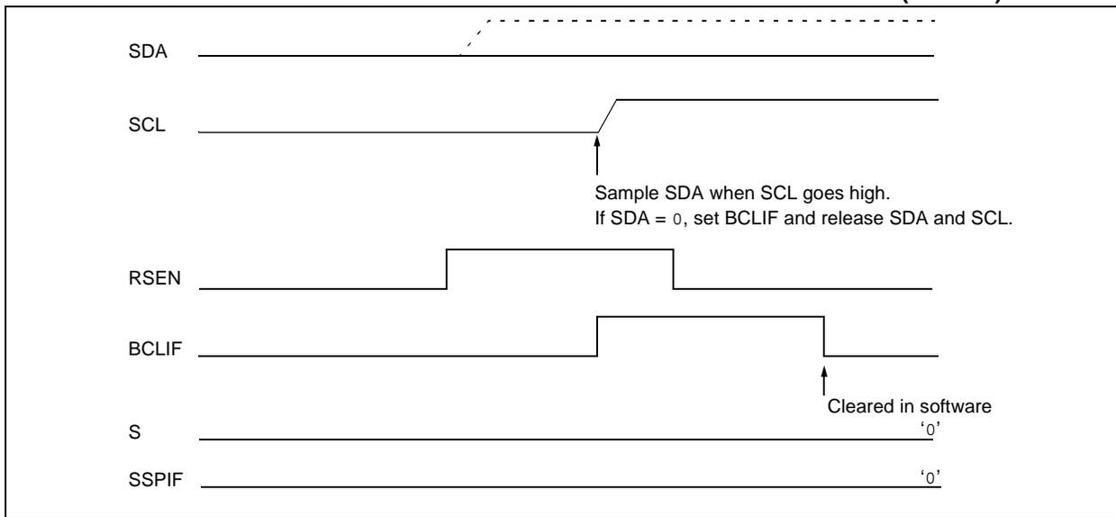
**FIGURE 17-32: BUS COLLISION DURING REPEATED START CONDITION (CASE 2)**
