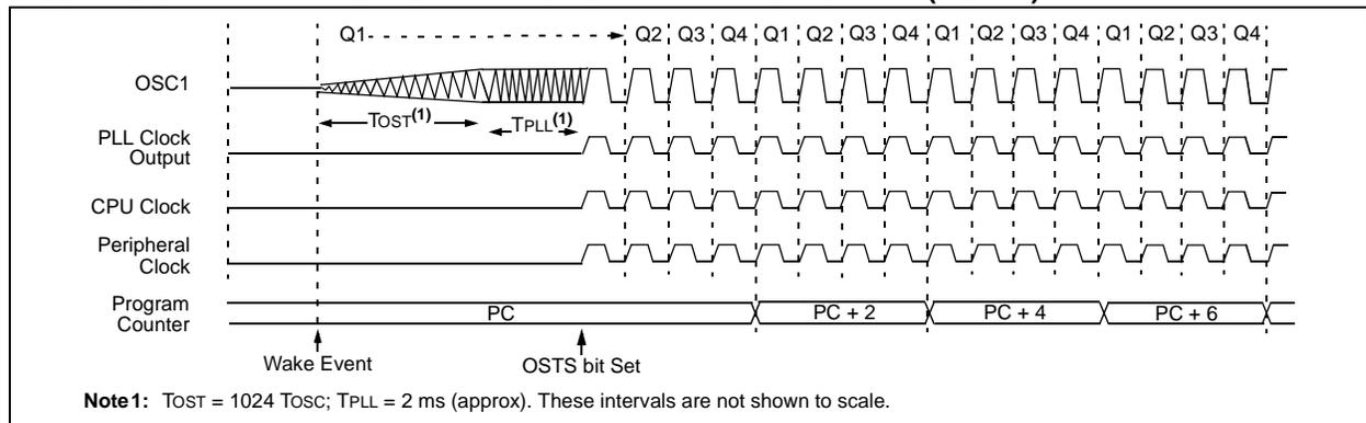
**Note 1:**  $T_{OST} = 1024 T_{OSC}$ ;  $T_{PLL} = 2$  ms (approx). These intervals are not shown to scale.
