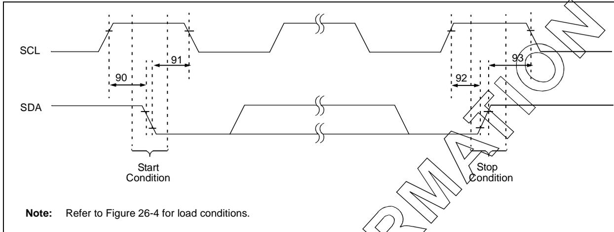
**TABLE 26-20: MASTER SSP I<sup>2</sup>C™ BUS START/STOP BITS REQUIREMENTS**
