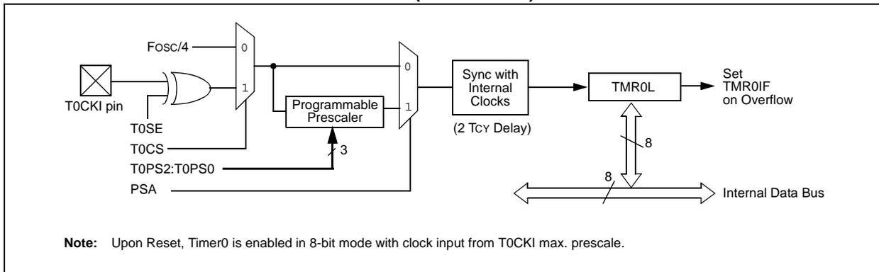
**FIGURE 11-2: TIMER0 BLOCK DIAGRAM (16-BIT MODE)**
