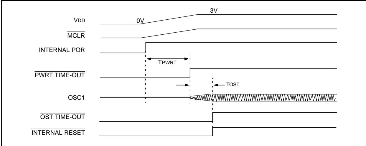
**FIGURE 4-7: TIME-OUT SEQUENCE ON POR w/PLL ENABLED ( $\overline{\text{MCLR}}$  TIED TO V<sub>DD</sub>)**
