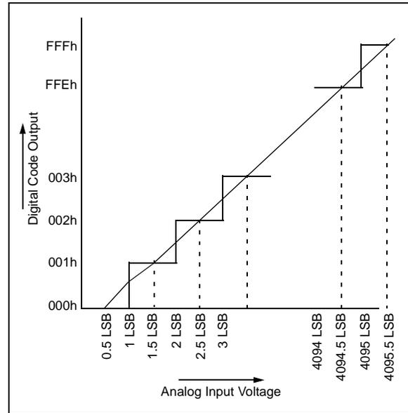
**FIGURE 19-3: ANALOG INPUT MODEL**
