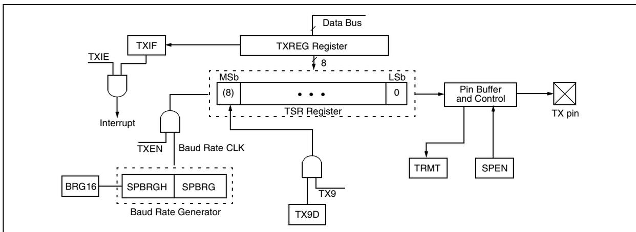
**FIGURE 17-4: ASYNCHRONOUS TRANSMISSION**
