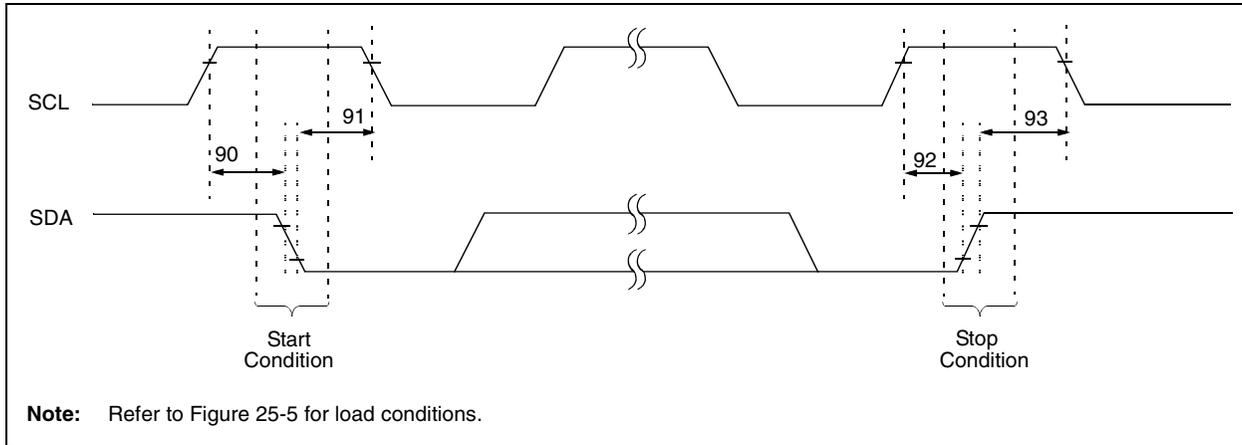
**TABLE 25-18: I<sup>2</sup>C™ BUS START/STOP BITS REQUIREMENTS (SLAVE MODE)**
