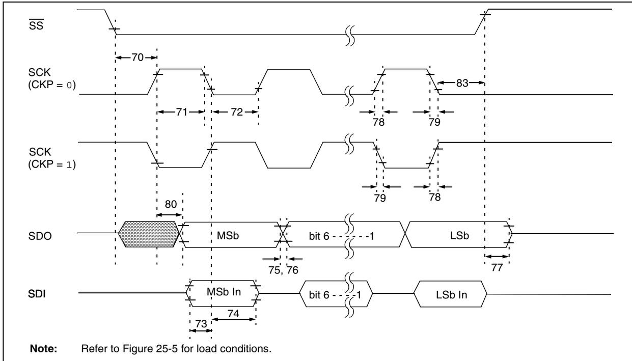
**TABLE 25-16: EXAMPLE SPI MODE REQUIREMENTS (SLAVE MODE TIMING, CKE = 0)**
