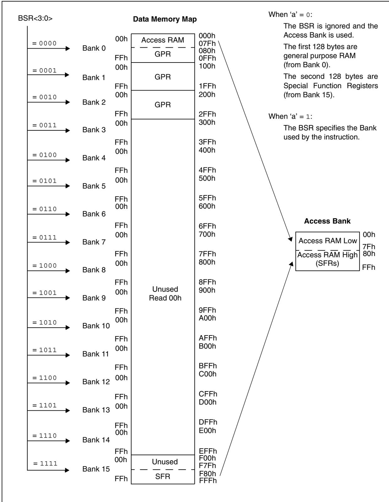
**FIGURE 5-6: DATA MEMORY MAP FOR PIC18F2510/4510 DEVICES**
