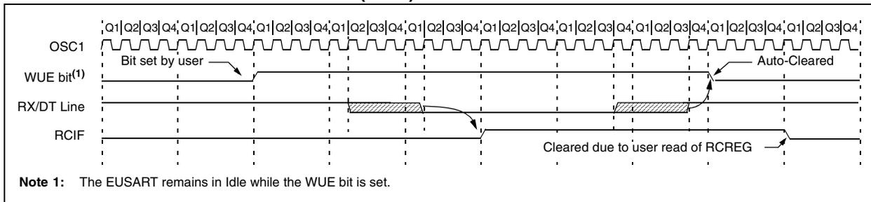
**FIGURE 17-9: AUTO-WAKE-UP BIT (WUE) TIMINGS DURING SLEEP**
