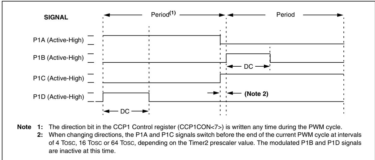
**FIGURE 15-9: PWM DIRECTION CHANGE AT NEAR 100% DUTY CYCLE**
