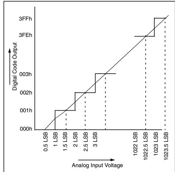
**FIGURE 18-3: ANALOG INPUT MODEL**
