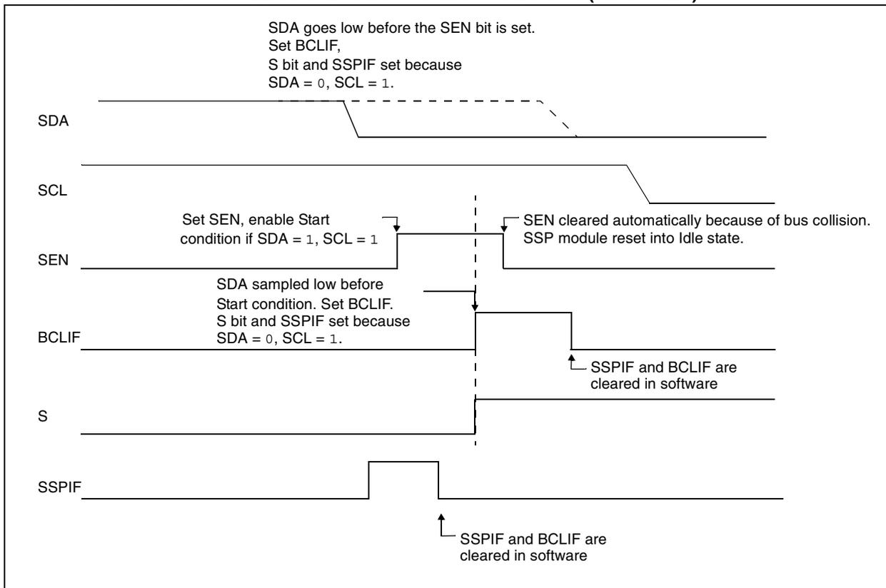
**FIGURE 16-27: BUS COLLISION DURING START CONDITION (SCL = 0)**
