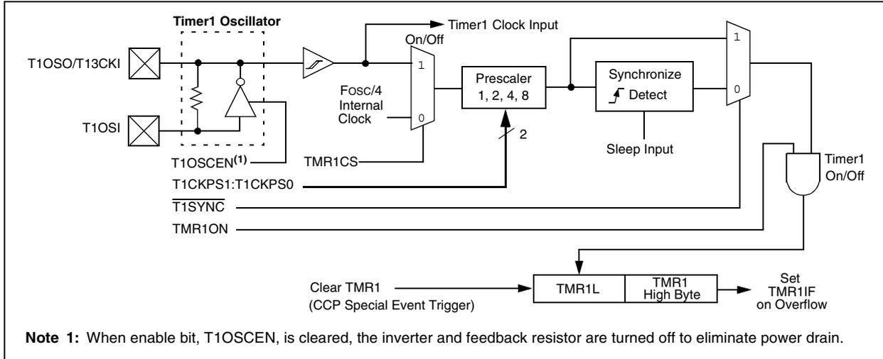
**FIGURE 11-2: TIMER1 BLOCK DIAGRAM (16-BIT READ/WRITE MODE)**
