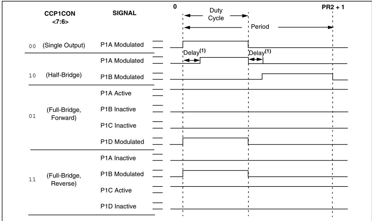
**FIGURE 15-3: PWM OUTPUT RELATIONSHIPS (ACTIVE-LOW STATE)**
