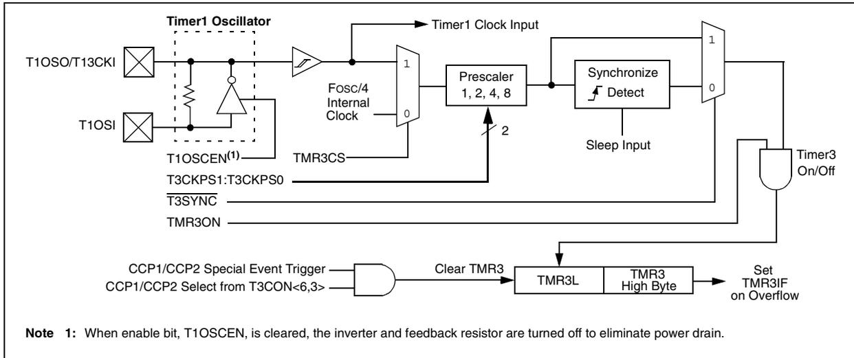
**FIGURE 13-2: TIMER3 BLOCK DIAGRAM (16-BIT READ/WRITE MODE)**
