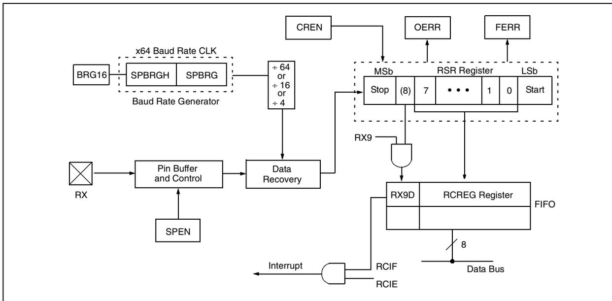
**FIGURE 17-7: ASYNCHRONOUS RECEPTION**
