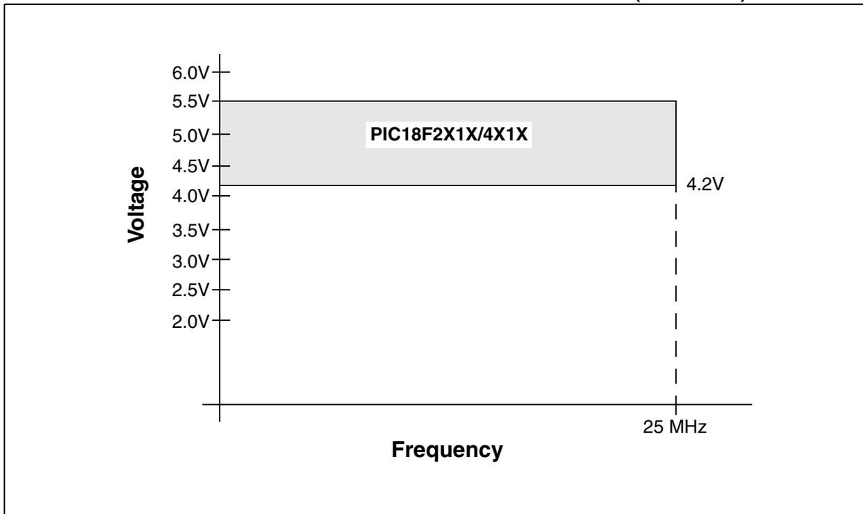
FIGURE 25-3: PIC18LF2X1X/4X1X VOLTAGE-FREQUENCY GRAPH (INDUSTRIAL)
