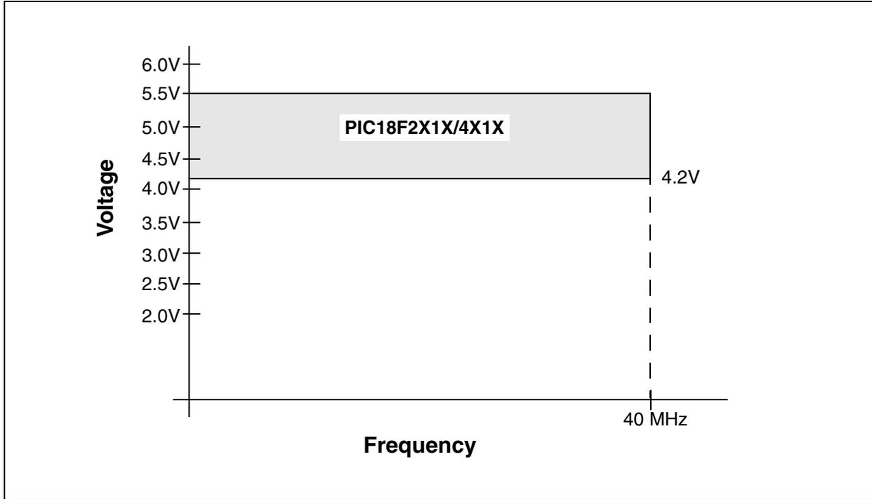
FIGURE 25-2: PIC18F2X1X/4X1X VOLTAGE-FREQUENCY GRAPH (EXTENDED)
