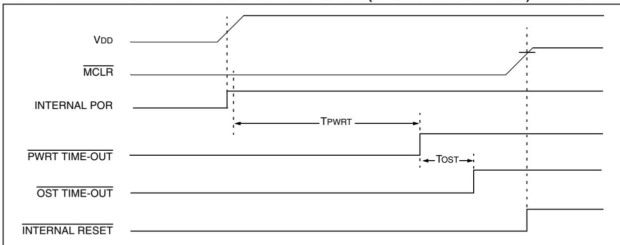
**FIGURE 4-6: SLOW RISE TIME ( $\overline{\text{MCLR}}$  TIED TO  $V_{DD}$ ,  $V_{DD}$  RISE  $>$   $T_{PWRT}$ )**
