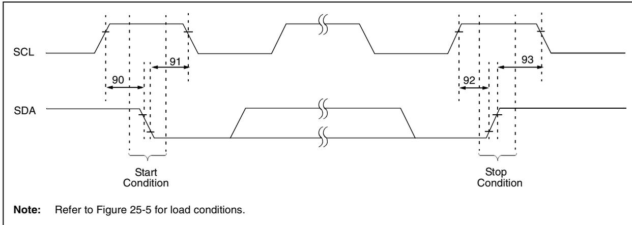
**TABLE 25-20: MASTER SSP I<sup>2</sup>C™ BUS START/STOP BITS REQUIREMENTS**
