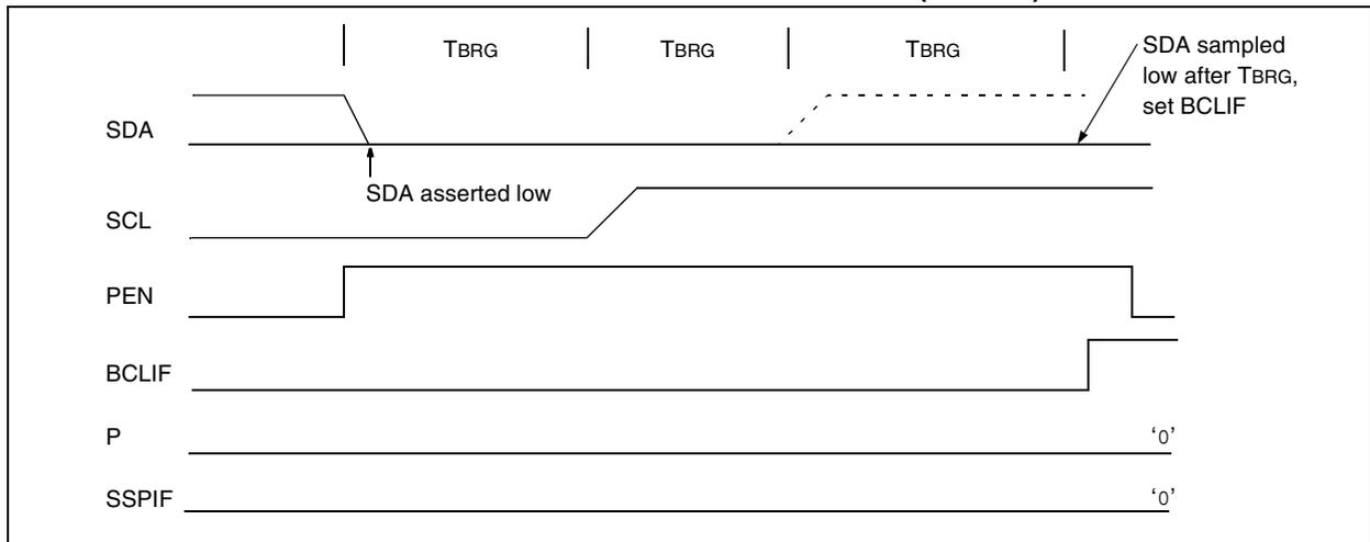
**FIGURE 16-32: BUS COLLISION DURING A STOP CONDITION (CASE 2)**
