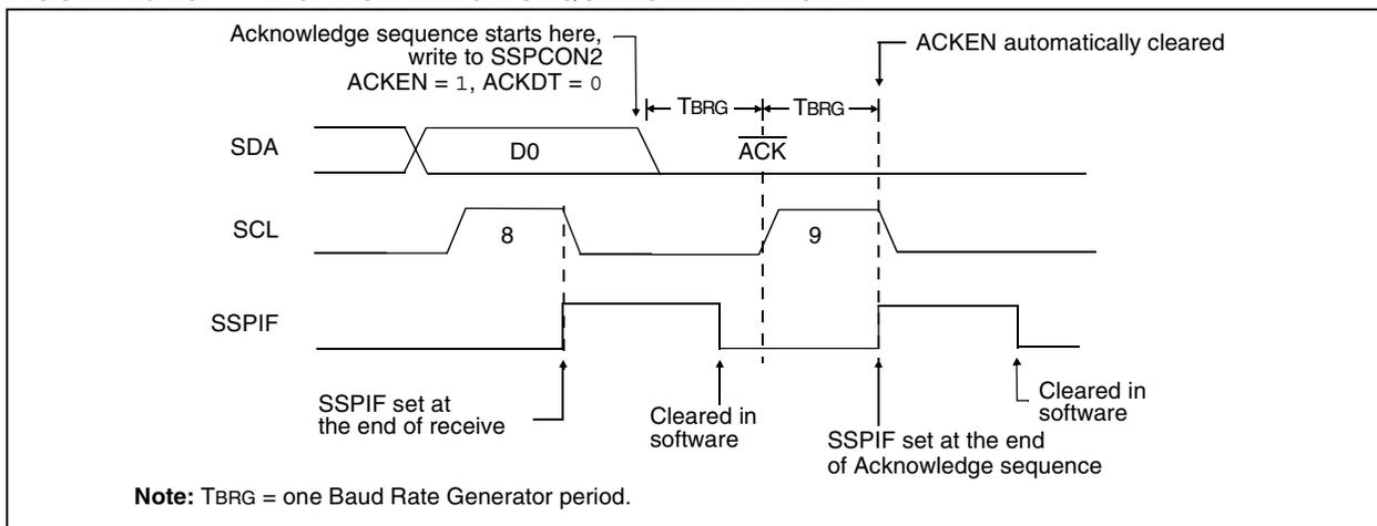
**FIGURE 16-24: STOP CONDITION RECEIVE OR TRANSMIT MODE**
