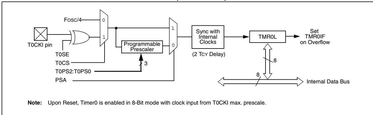
**FIGURE 10-2: TIMER0 BLOCK DIAGRAM (16-BIT MODE)**
