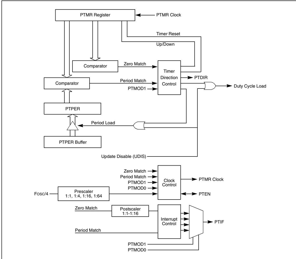
The PWM time base can be configured for four different modes of operation:
