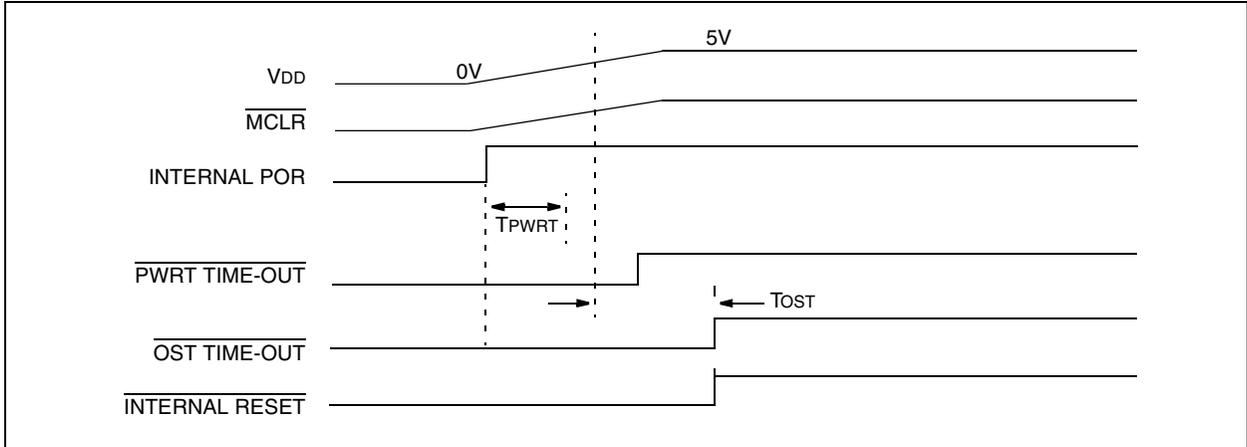
**FIGURE 4-7: TIME-OUT SEQUENCE ON POR W/PLL ENABLED ( $\overline{\text{MCLR}}$  TIED TO  $V_{\text{DD}}$ )**
