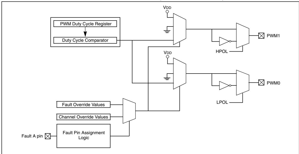
This module contains three duty cycle generators, numbered 0 through 2. The module has six PWM output pins, numbered 0 through 5. The six PWM outputs are grouped into output pairs of even and odd numbered outputs. In Complementary modes, the even PWM pins must always be the complement of the corresponding odd PWM pins. For example, PWM0 will be the complement of PWM1 and PWM2 will be the complement of PWM3. The dead-time generator
