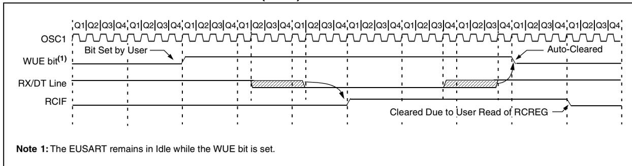
**FIGURE 14-9: AUTO-WAKE-UP BIT (WUE) TIMINGS DURING SLEEP**
