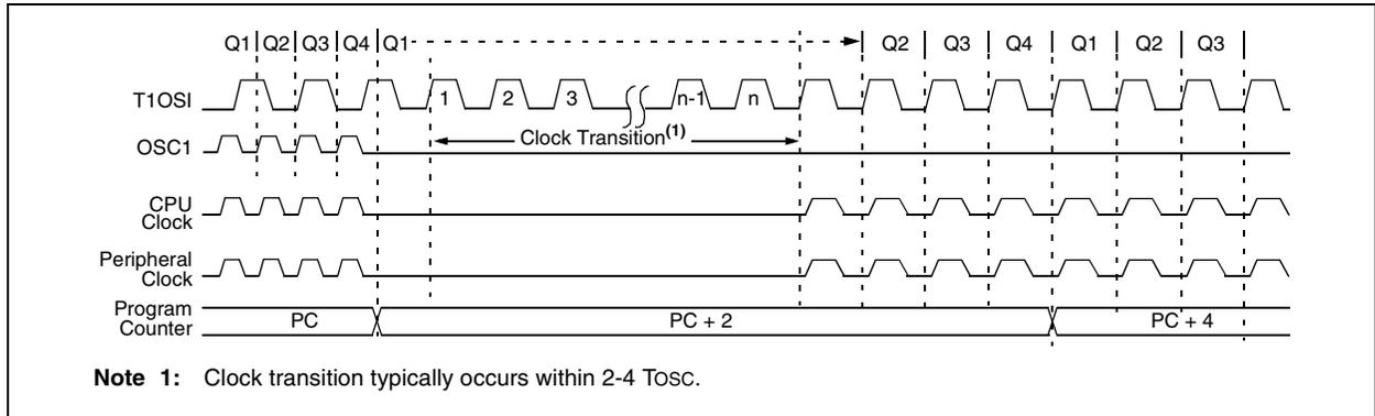
**FIGURE 3-2: TRANSITION TIMING FROM SEC\_RUN MODE TO PRI\_RUN MODE (HSPLL)**
