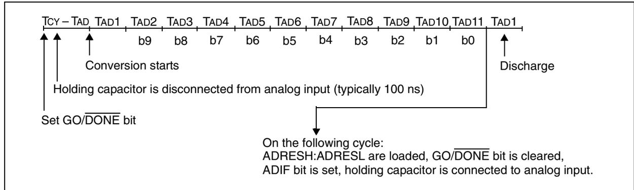
**FIGURE 15-5: A/D CONVERSION TAD CYCLES (ACQT<2:0> = 010, TACQ = 4 TAD)**
