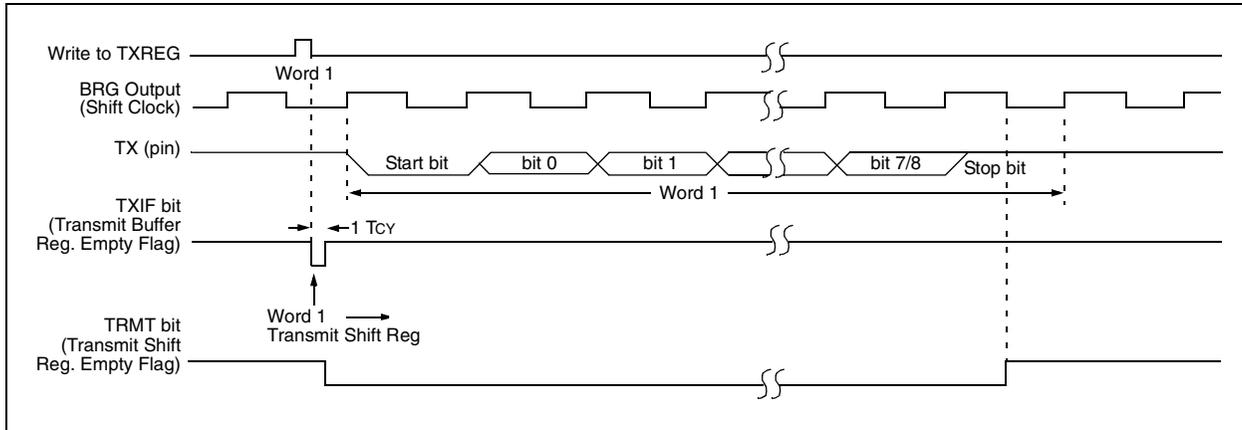
**FIGURE 14-5: ASYNCHRONOUS TRANSMISSION (BACK-TO-BACK)**
