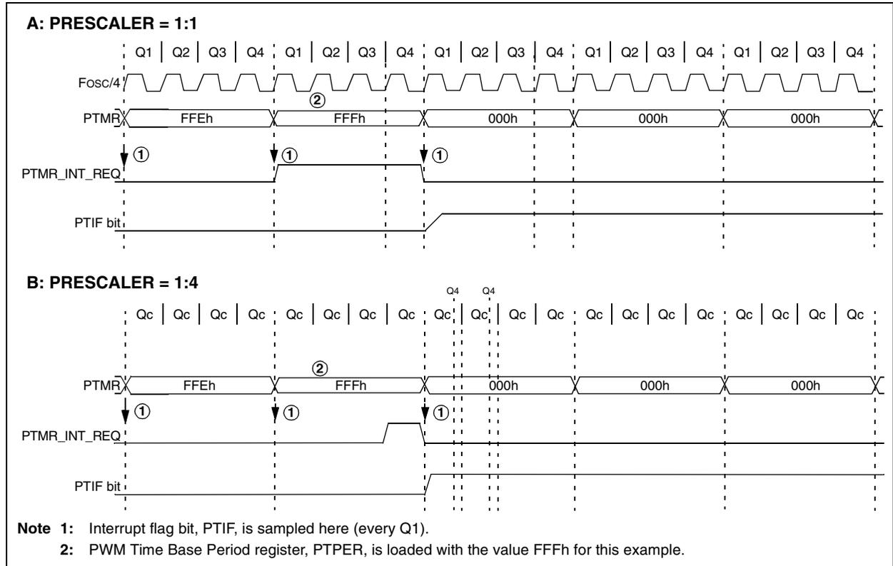
**FIGURE 13-7: PWM TIME BASE INTERRUPTS, CONTINUOUS UP/DOWN COUNT MODE**
