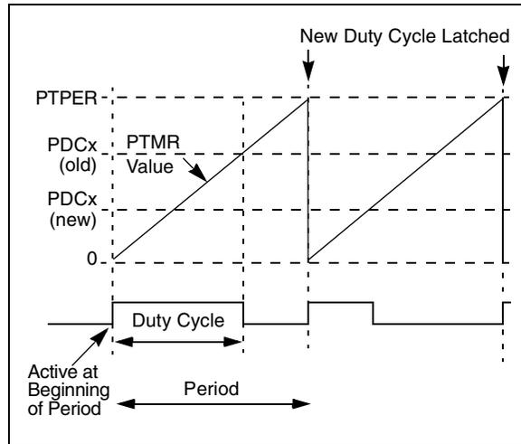
**FIGURE 13-13: DUTY CYCLE UPDATE TIMES IN CONTINUOUS UP/DOWN COUNT MODE**
