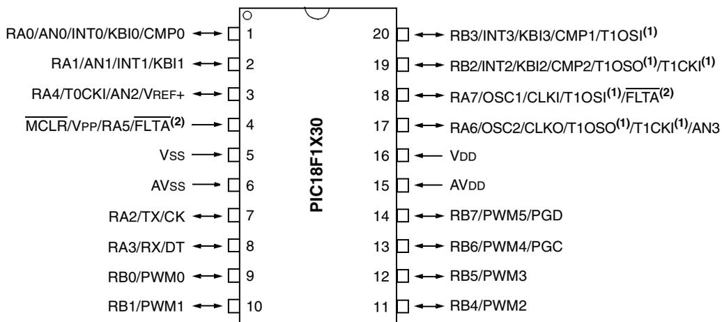
**Note 1:** Placement of T1OSI and T1OSO/T1CKI depends on the value of Configuration bit, T1OSCMX, of CONFIG3H.
