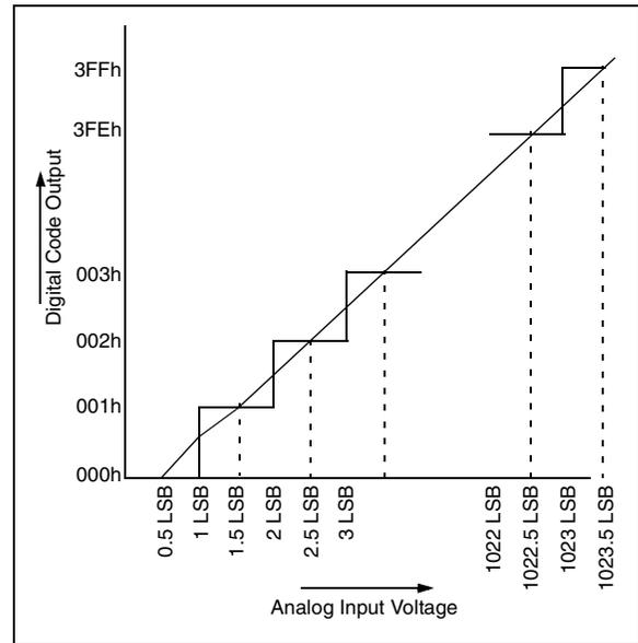
**FIGURE 15-3: ANALOG INPUT MODEL**
