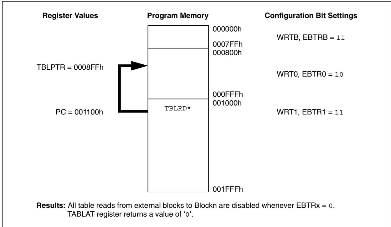
**FIGURE 19-8: EXTERNAL BLOCK TABLE READ (EBTRx) ALLOWED**
