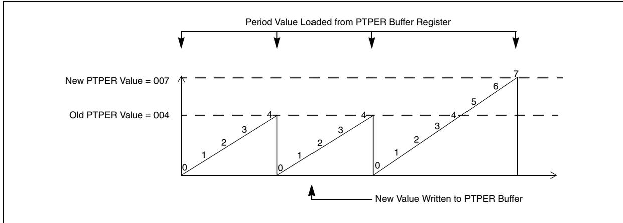
**FIGURE 13-10: PWM PERIOD BUFFER UPDATES IN CONTINUOUS UP/DOWN COUNT MODES**
