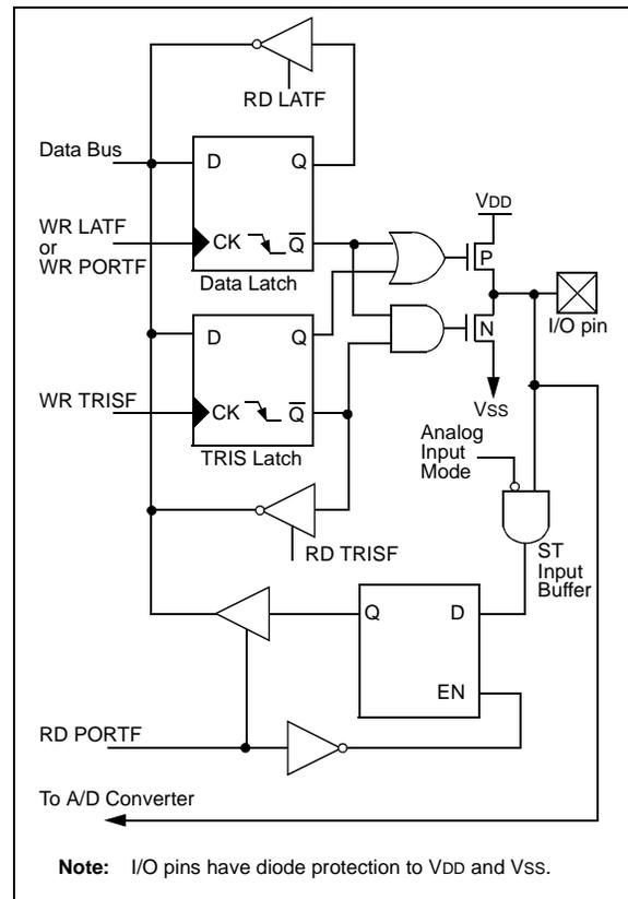
**FIGURE 9-12: RF5:RF3 PINS BLOCK DIAGRAM**
