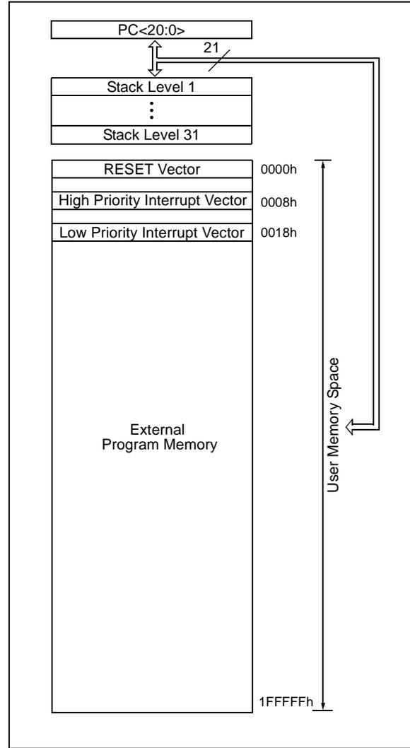
**FIGURE 4-3: PROGRAM MEMORY MAP AND STACK FOR PIC18C601 (PGRM = 1)**
