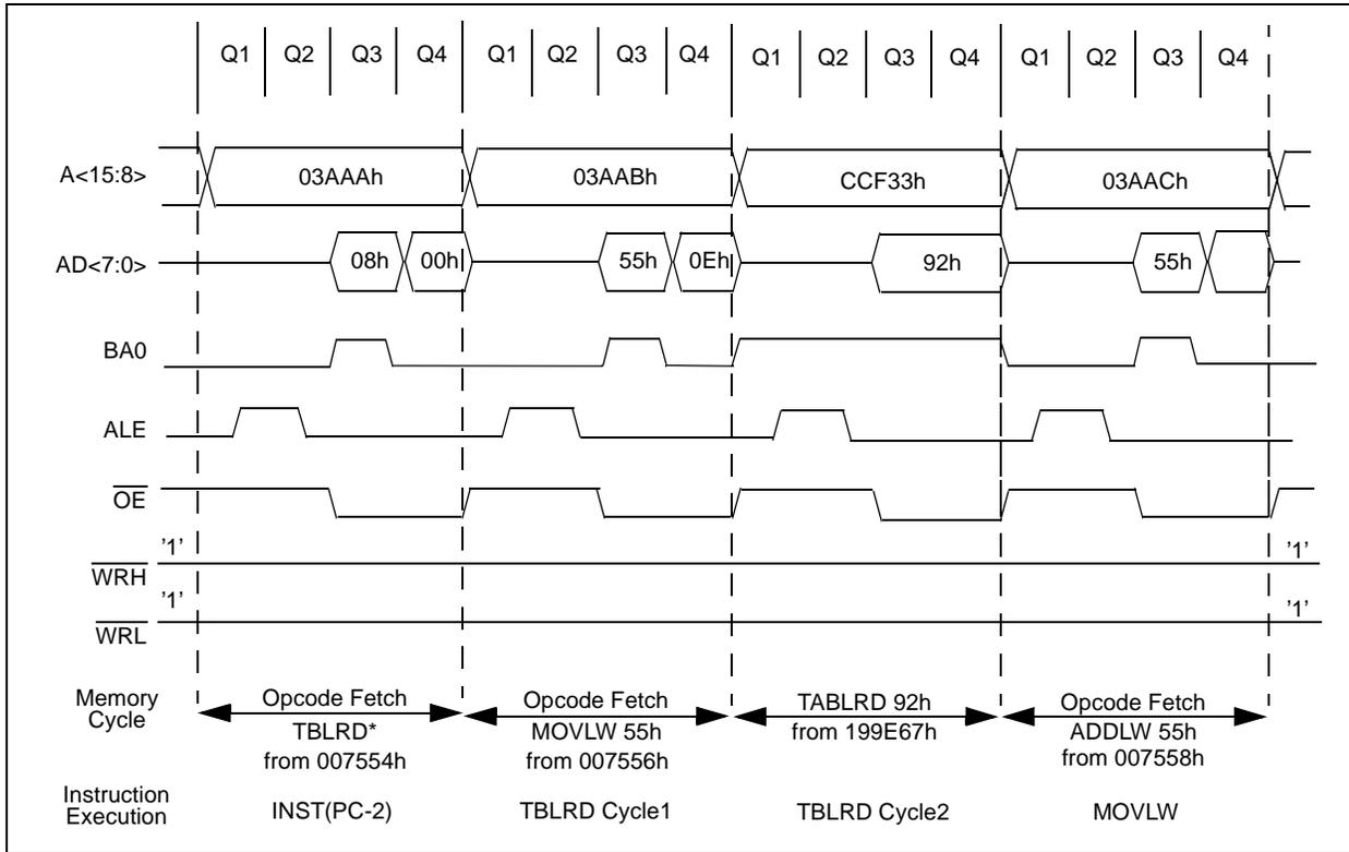
**FIGURE 6-5: TBLRD EXTERNAL BUS TIMING (16-BIT MODE)**
