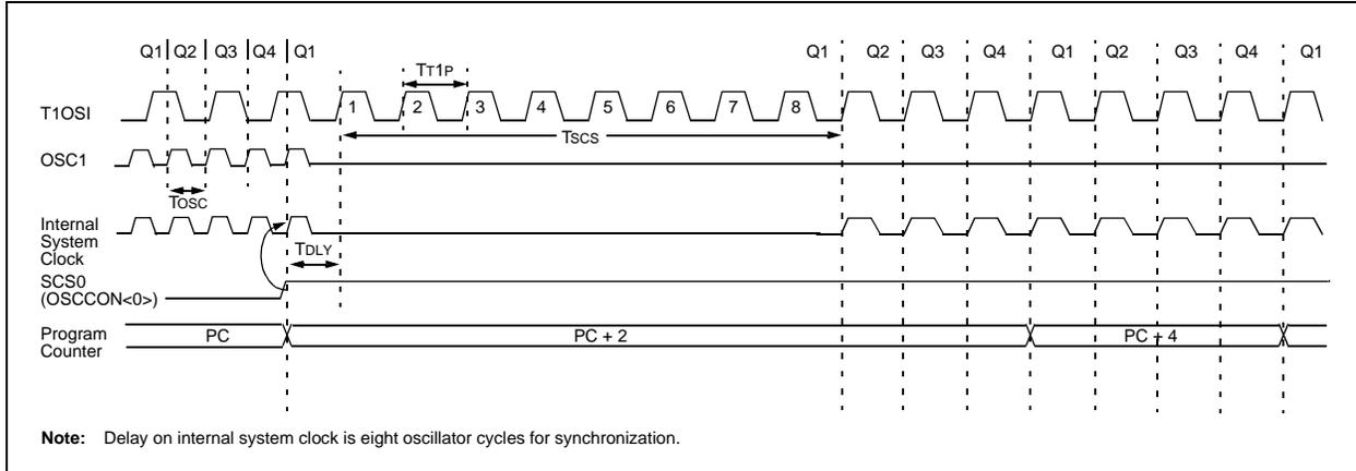
**FIGURE 2-7: TIMING DIAGRAM FOR TRANSITION BETWEEN TIMER1 AND OSC1 (HS, LP)**
