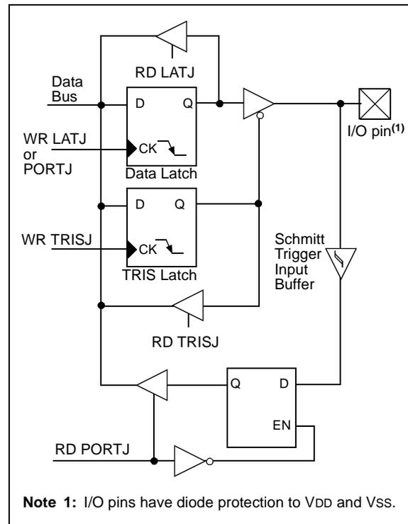
**FIGURE 9-20: PORTJ BLOCK DIAGRAM IN SYSTEM DATA BUS MODE**
