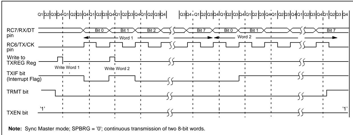
**FIGURE 16-7: SYNCHRONOUS TRANSMISSION (THROUGH TXEN)**
