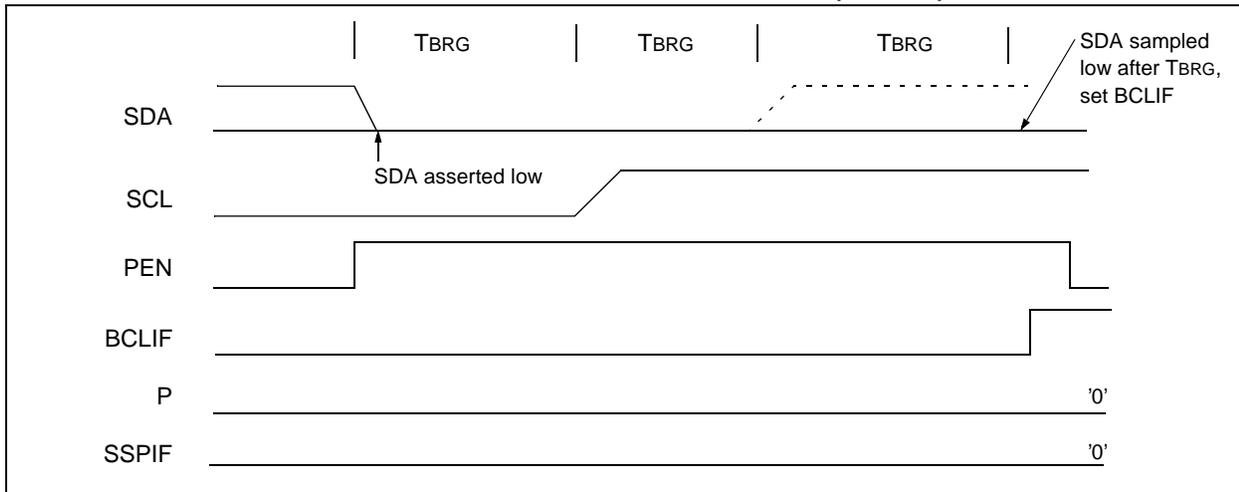
**FIGURE 15-27: BUS COLLISION DURING A STOP CONDITION (CASE 2)**
