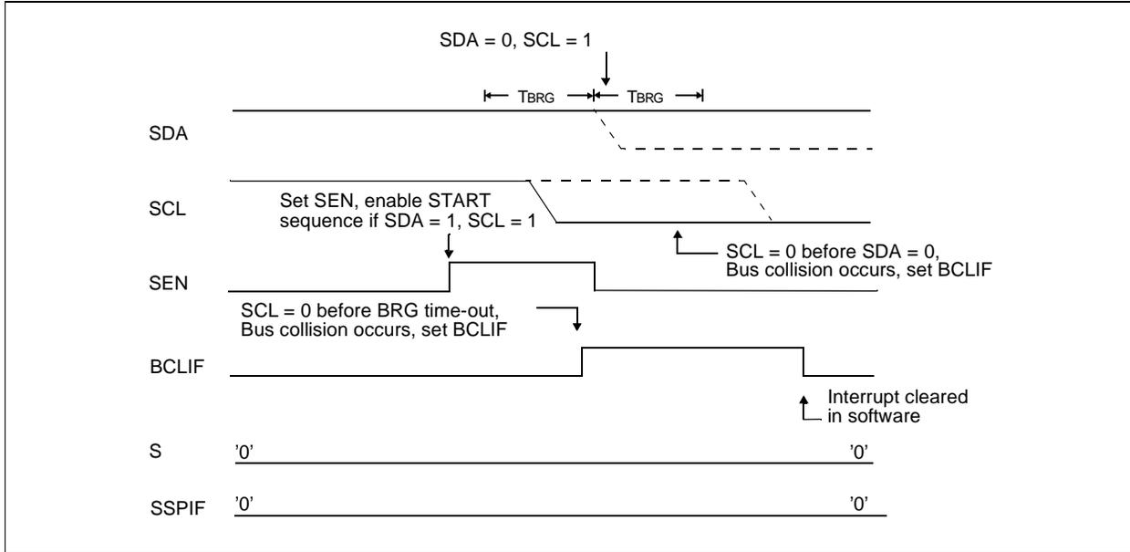
**FIGURE 15-23: BRG RESET DUE TO SDA ARBITRATION DURING START CONDITION**
