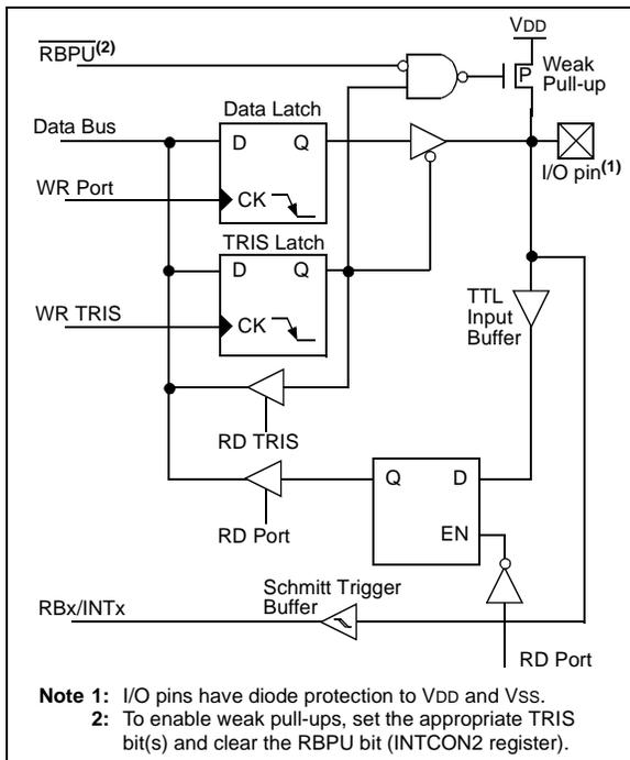
**FIGURE 9-5: RB3 PIN BLOCK DIAGRAM**
