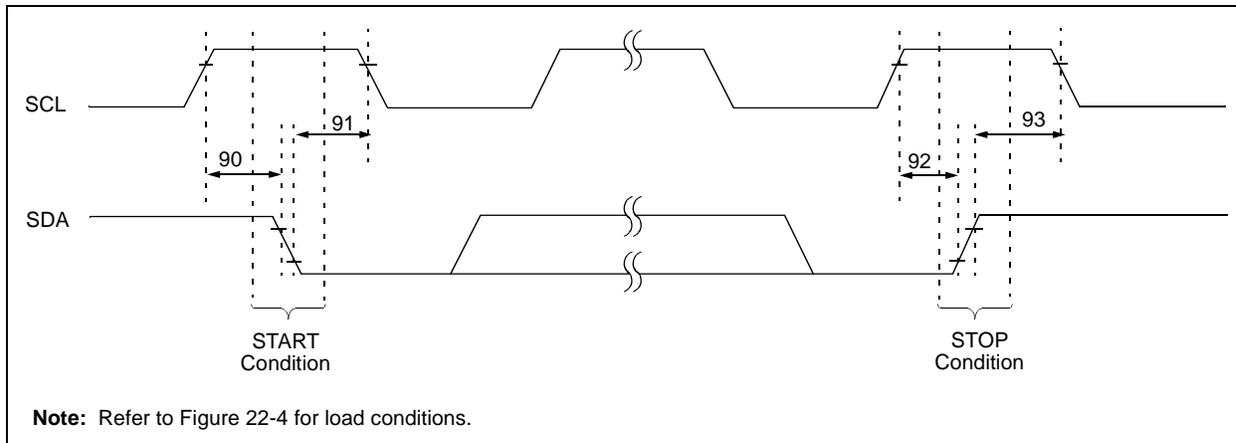
**TABLE 22-18: MASTER SSP I<sup>2</sup>C BUS START/STOP BITS REQUIREMENTS**
