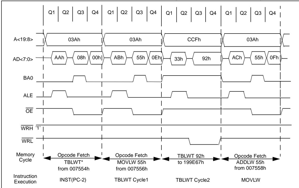
**FIGURE 6-7: TBLWT EXTERNAL INTERFACE TIMING (8-BIT DE-MULTIPLEXED MODE)**
