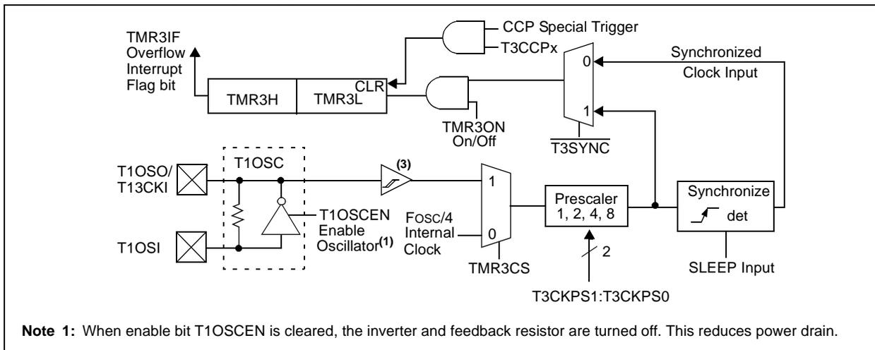
**FIGURE 13-2: TIMER3 BLOCK DIAGRAM CONFIGURED IN 16-BIT READ/WRITE MODE**
