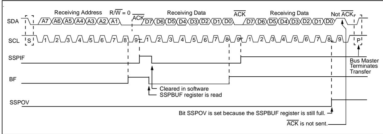
**FIGURE 15-8: I<sup>2</sup>C SLAVE MODE WAVEFORMS FOR TRANSMISSION (7-BIT ADDRESS)**
