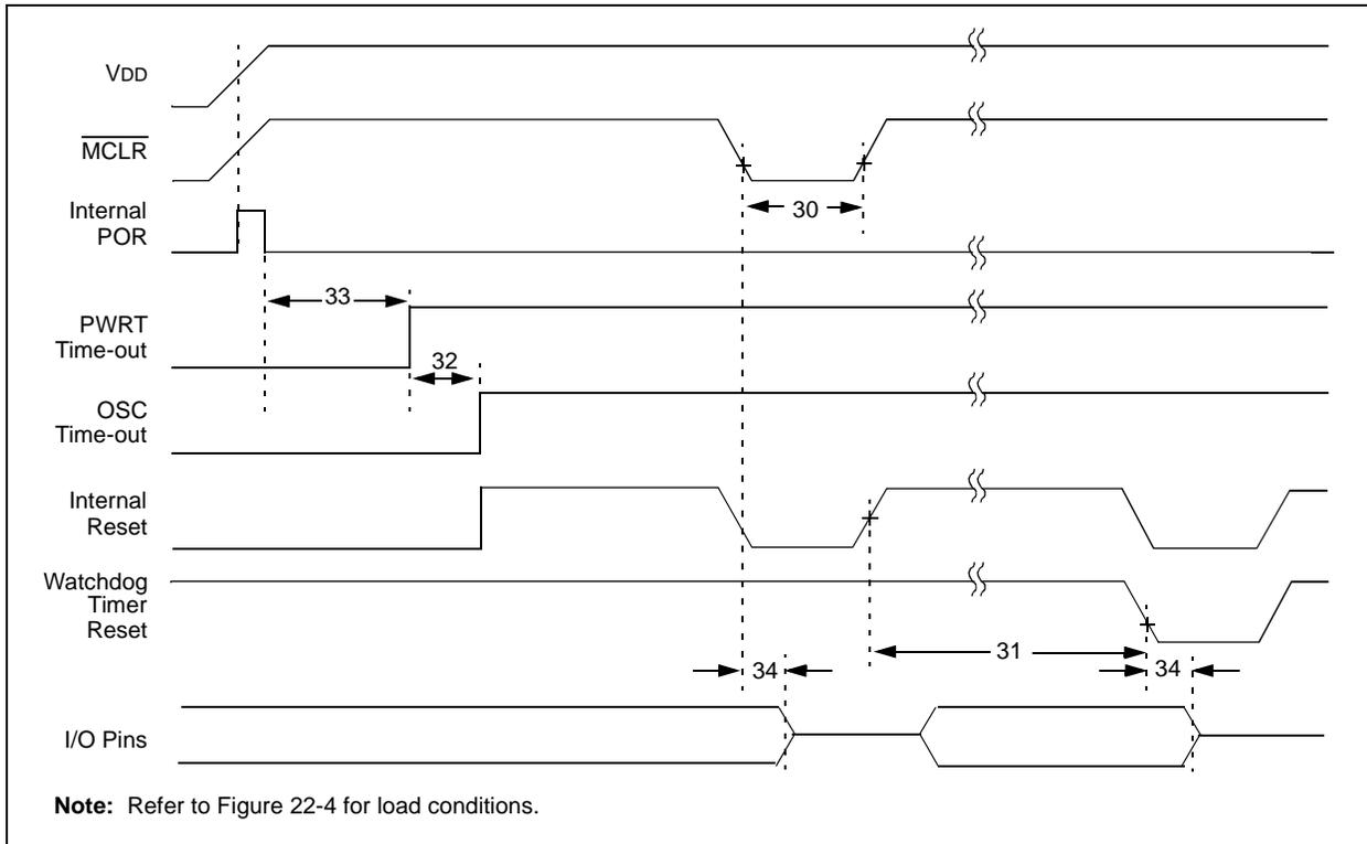
**TABLE 22-9: RESET, WATCHDOG TIMER, OSCILLATOR START-UP TIMER, POWER-UP TIMER AND BROWN-OUT RESET REQUIREMENTS**
