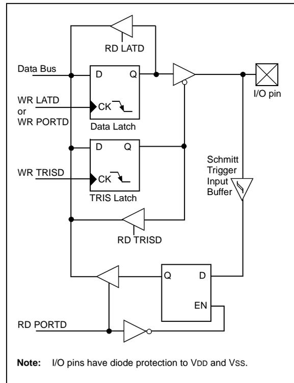
**FIGURE 9-8: PORTD BLOCK DIAGRAM IN SYSTEM BUS MODE**
