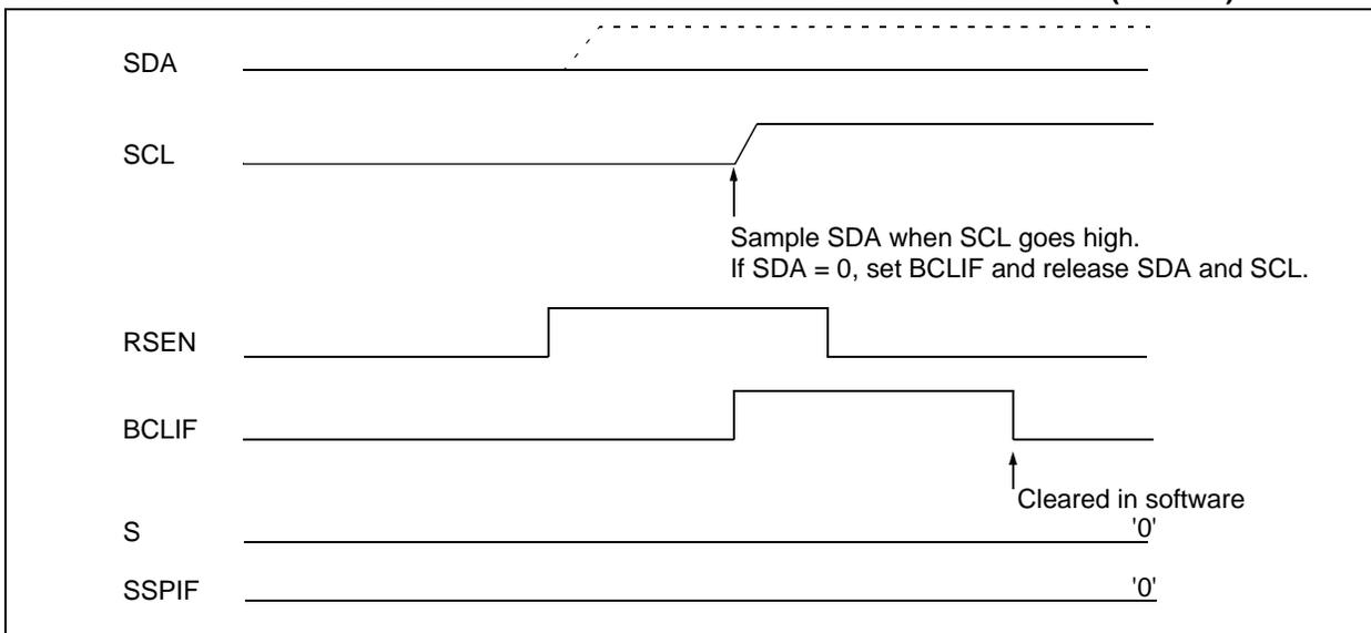
**FIGURE 15-25: BUS COLLISION DURING REPEATED START CONDITION (CASE 2)**
