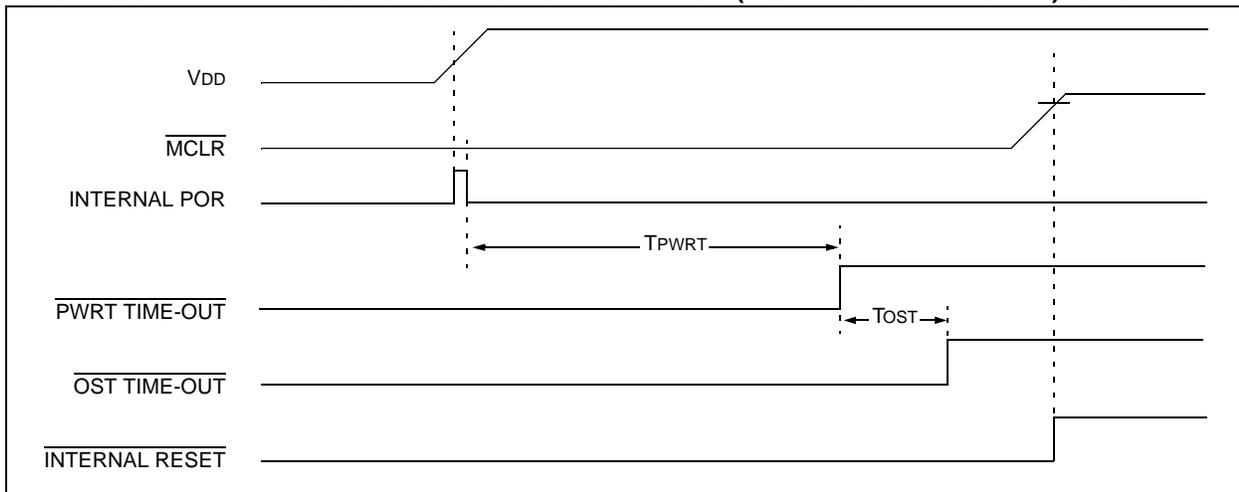
**FIGURE 3-6: SLOW RISE TIME ( $\overline{\text{MCLR}}$  TIED TO  $V_{DD}$ )**
