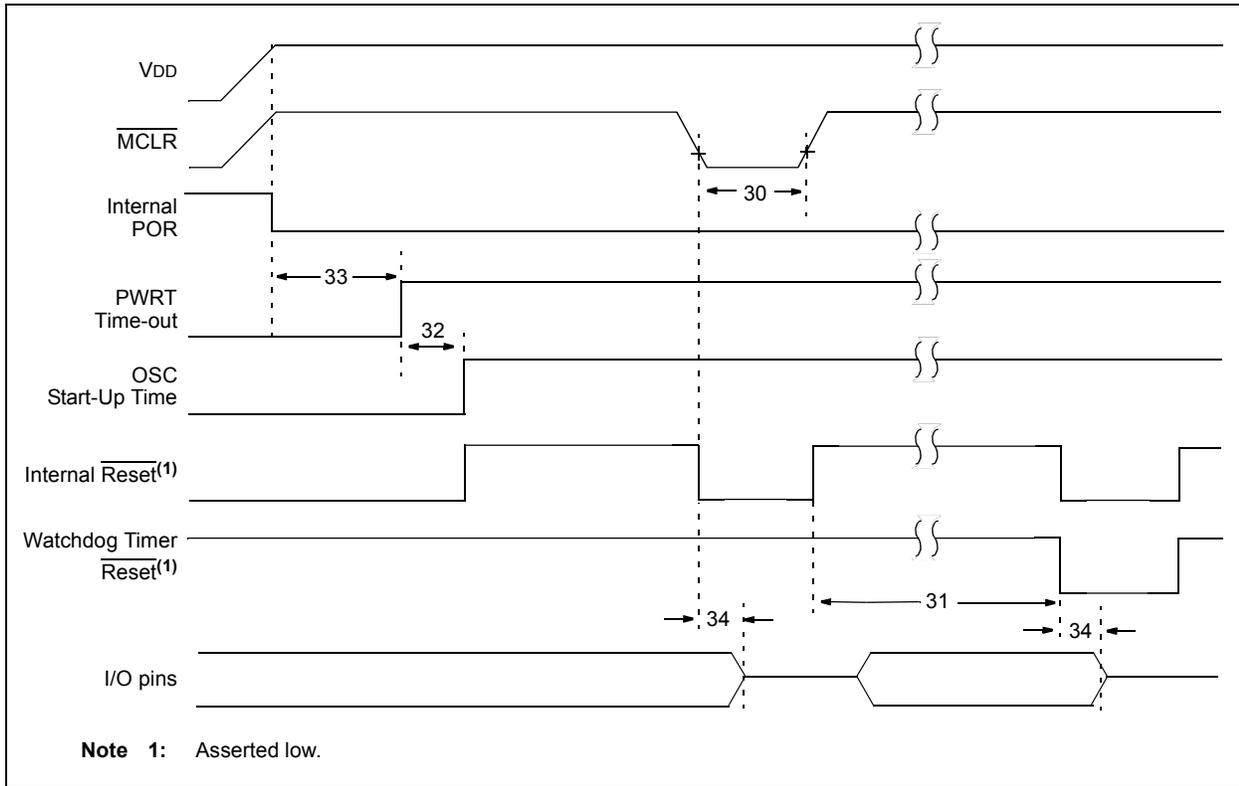
**FIGURE 17-7: BROWN-OUT RESET TIMING AND CHARACTERISTICS**
