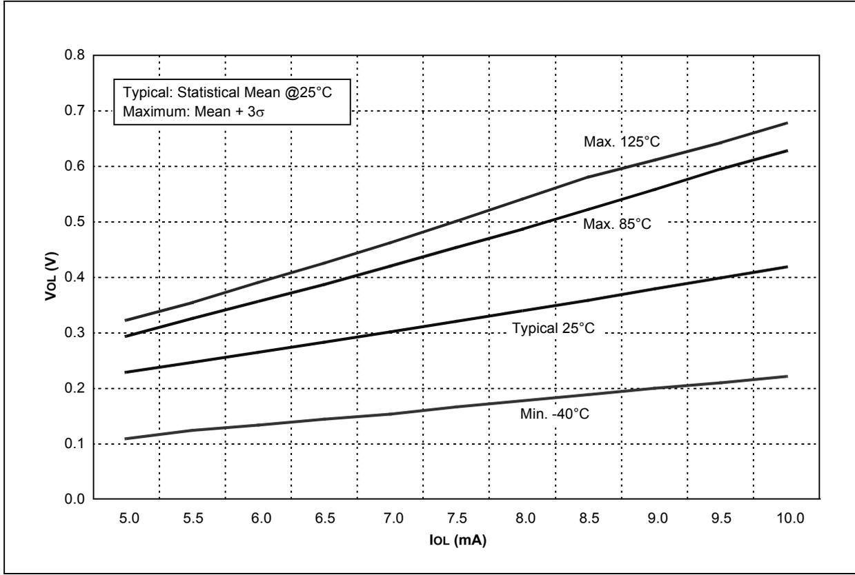
FIGURE 18-27: VOL vs. IOL OVER TEMPERATURE (VDD = 5.0V)
