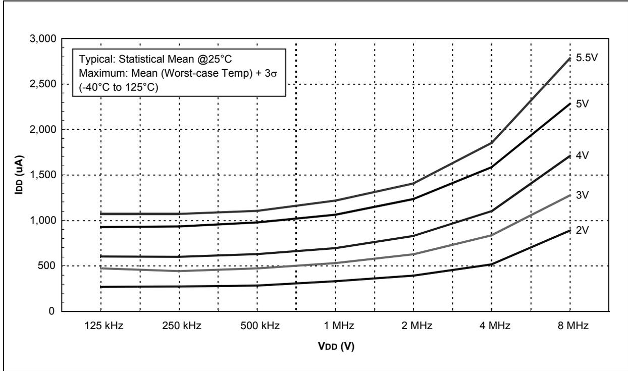
FIGURE 18-13: TYPICAL I<sub>PD</sub> vs. V<sub>DD</sub> (SLEEP MODE, ALL PERIPHERALS DISABLED)
