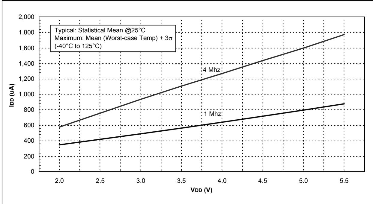
**FIGURE 18-9: I<sub>DD</sub> vs. V<sub>DD</sub> OVER F<sub>osc</sub> (LFINTOSC MODE, 31 kHz)**
