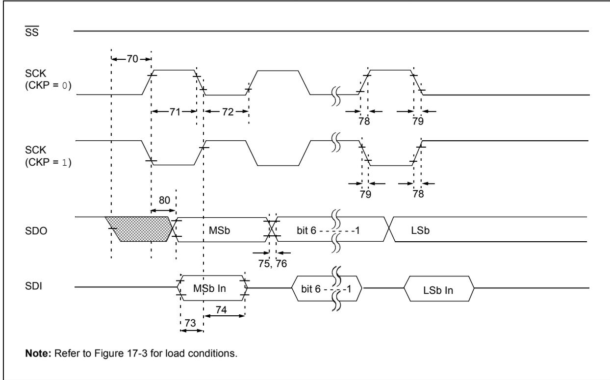
**FIGURE 17-15: SPI MASTER MODE TIMING (CKE = 1, SMP = 1)**
