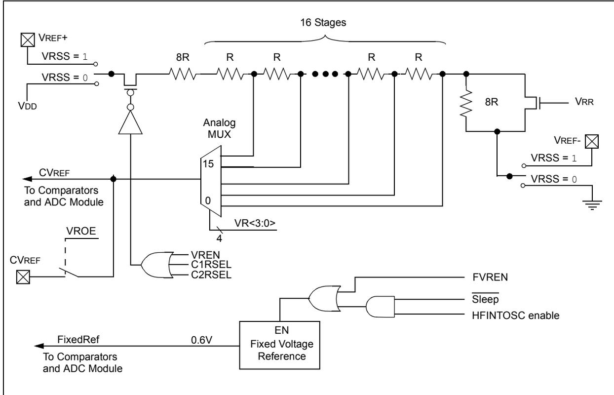
**FIGURE 8-9: COMPARATOR AND ADC VOLTAGE REFERENCE BLOCK DIAGRAM**
