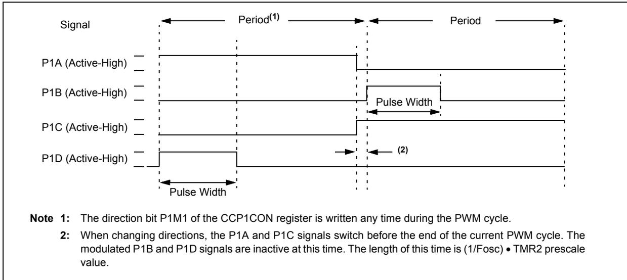
**FIGURE 11-13: EXAMPLE OF PWM DIRECTION CHANGE AT NEAR 100% DUTY CYCLE**
