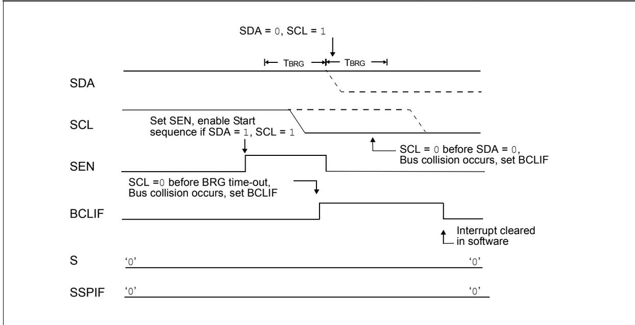
**FIGURE 13-23: BRG RESET DUE TO SDA ARBITRATION DURING START CONDITION**
