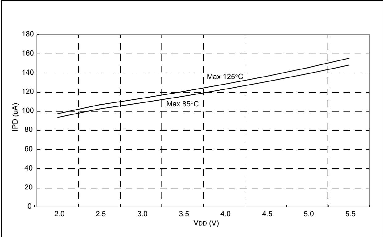
FIGURE 18-25: T1OSC IPD vs. VDD OVER TEMPERATURE (32 kHz)
