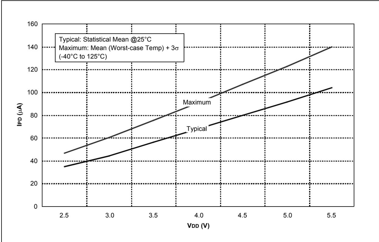
**FIGURE 18-17: TYPICAL WDT IPD vs. VDD (25°C)**
