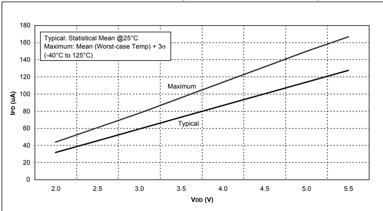
**FIGURE 18-16: BOR IPD vs. VDD OVER TEMPERATURE**
