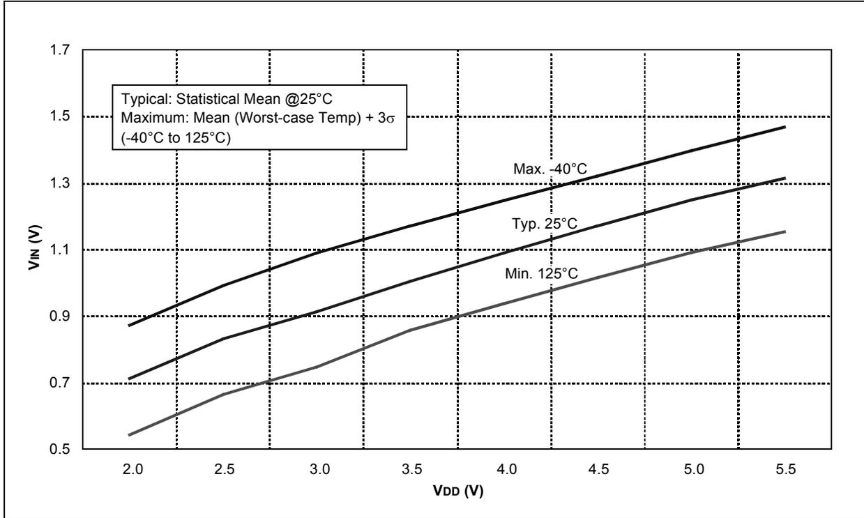
FIGURE 18-31: SCHMITT TRIGGER INPUT THRESHOLD  $V_{IN}$  vs.  $V_{DD}$  OVER TEMPERATURE
