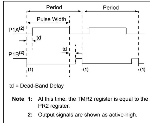
**FIGURE 11-18: EXAMPLE OF HALF-BRIDGE APPLICATIONS**
