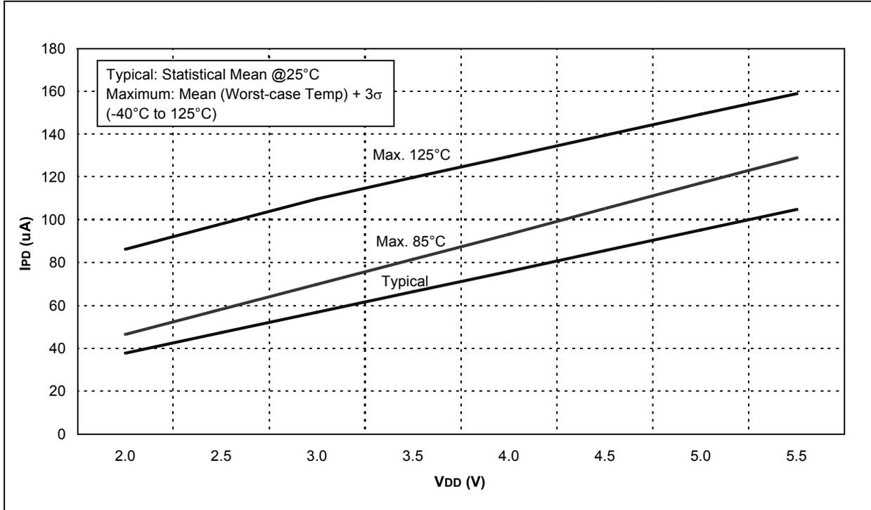
FIGURE 18-23: TYPICAL VP6 REFERENCE IPD vs. VDD (25°C)
