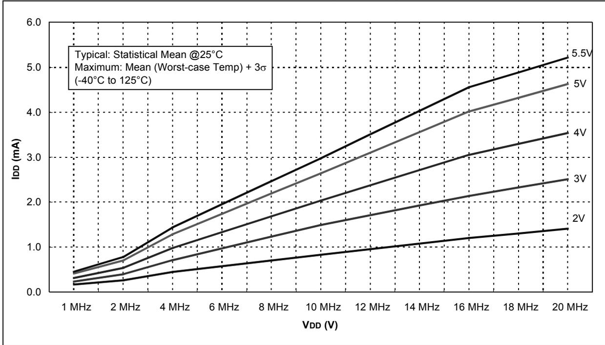
**FIGURE 18-3: TYPICAL I<sub>DD</sub> vs. F<sub>osc</sub> OVER V<sub>DD</sub> (HS MODE)**
