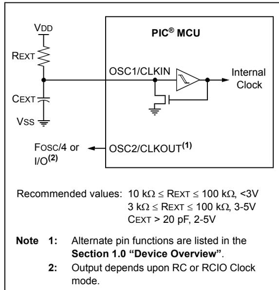
In RCIO mode, the RC circuit is connected to OSC1. OSC2 becomes an additional general purpose I/O pin.
