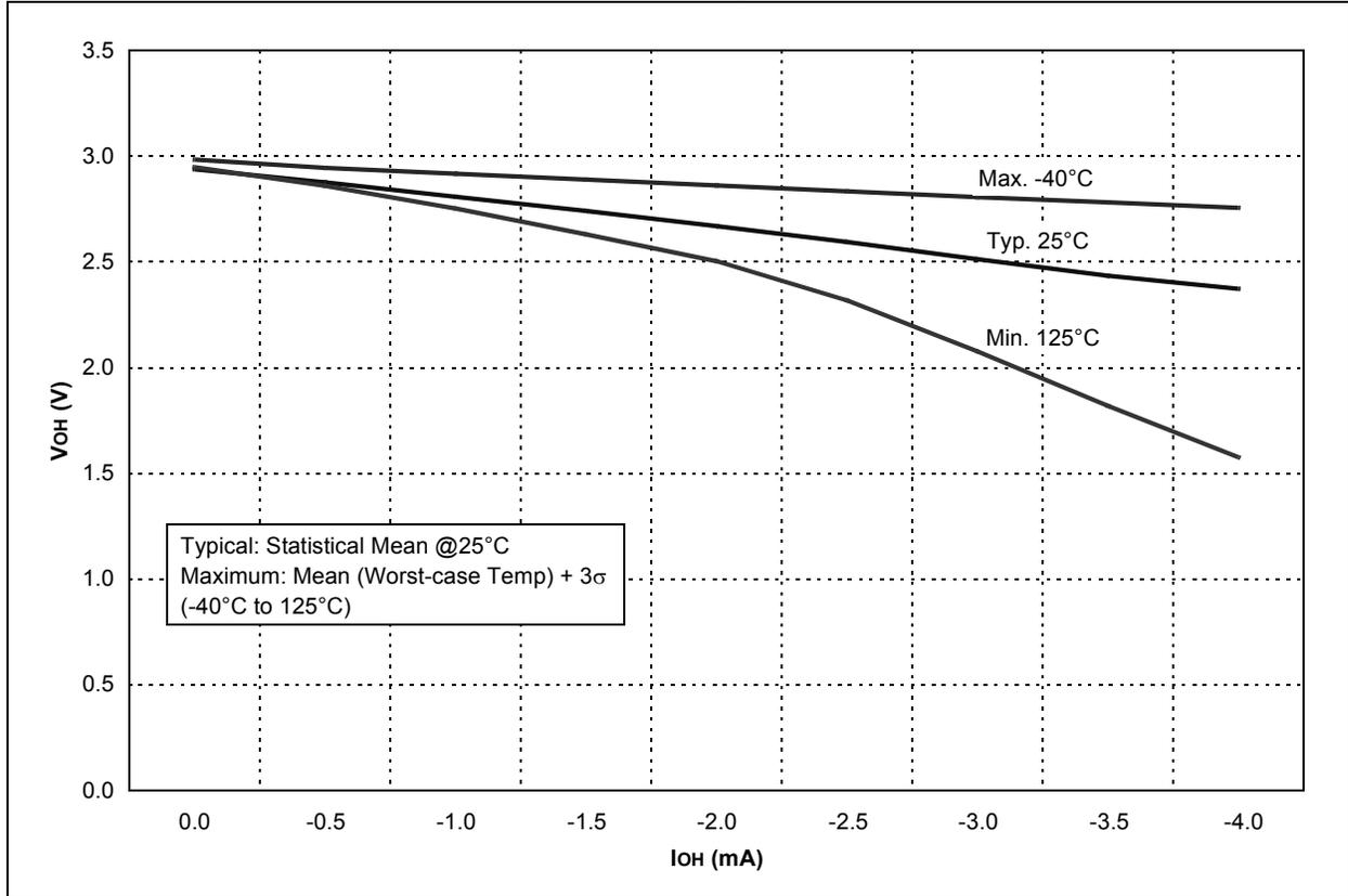
FIGURE 18-29:  $V_{OH}$  vs.  $I_{OH}$  OVER TEMPERATURE ( $V_{DD} = 5.0V$ )
