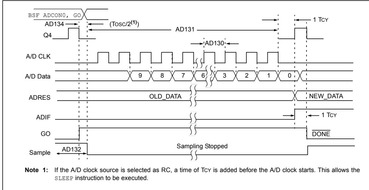
**FIGURE 17-11: PIC16F883/884/886/887 A/D CONVERSION TIMING (SLEEP MODE)**
