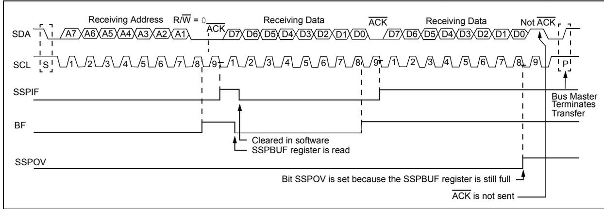
**FIGURE 13-8: I<sup>2</sup>C™ SLAVE MODE WAVEFORMS FOR TRANSMISSION (7-BIT ADDRESS)**
