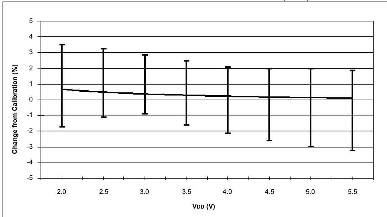
FIGURE 18-43: TYPICAL VP6 REFERENCE VOLTAGE vs.  $V_{DD}$  ( $25^{\circ}\text{C}$ )
