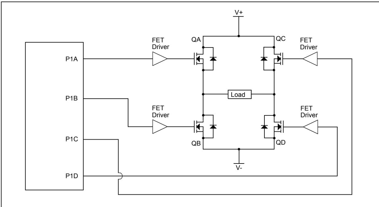
**FIGURE 11-11: EXAMPLE OF FULL-BRIDGE PWM OUTPUT**
