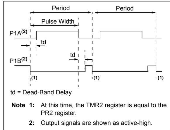
**FIGURE 11-9: EXAMPLE OF HALF-BRIDGE APPLICATIONS**
