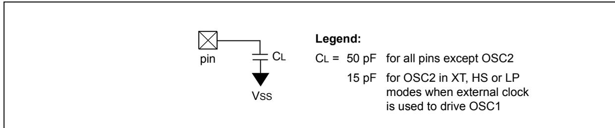
**FIGURE 14-4: EXTERNAL CLOCK TIMING**
