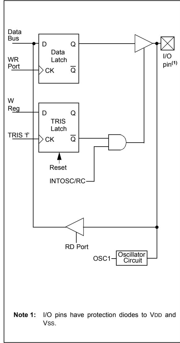
**FIGURE 5-8: BLOCK DIAGRAM OF RB5/GP5**
