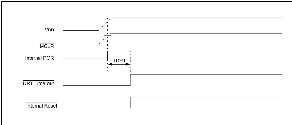
**FIGURE 10-10: TIME-OUT SEQUENCE ON POWER-UP ( $\overline{\text{MCLR}}$  TIED TO  $V_{\text{DD}}$ ): SLOW  $V_{\text{DD}}$  RISE TIME**
