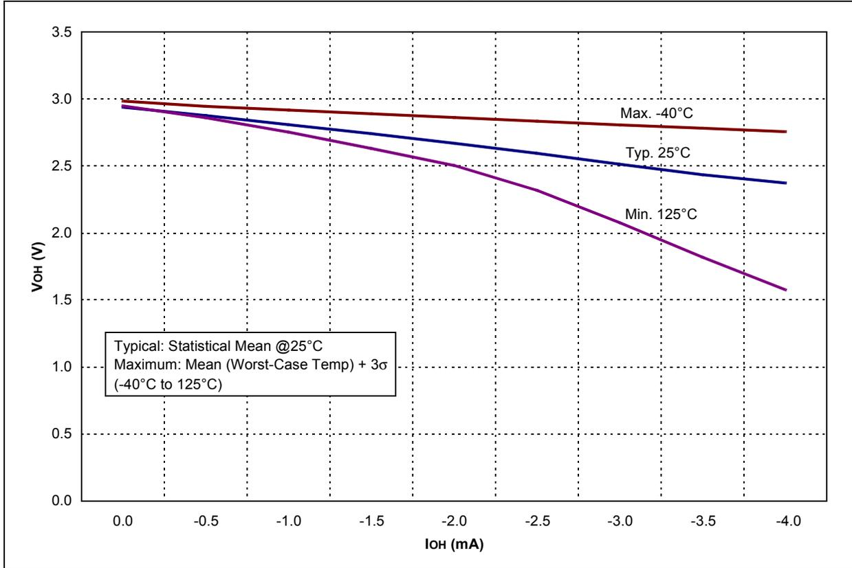
FIGURE 14-11:  $V_{OH}$  vs.  $I_{OH}$  OVER TEMPERATURE ( $V_{DD} = 5.0V$ )
