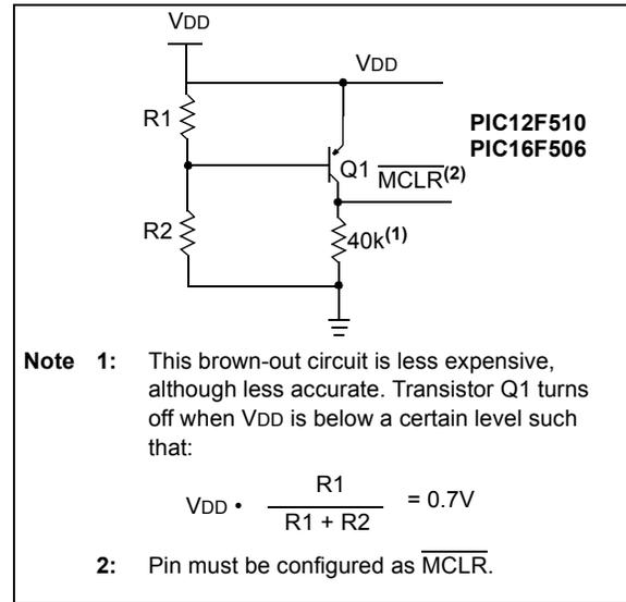
**FIGURE 10-14: BROWN-OUT PROTECTION CIRCUIT 3**
