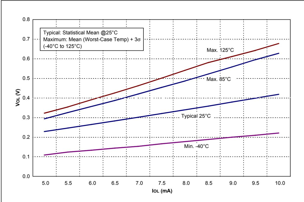
**FIGURE 14-9: VOL vs. IOL OVER TEMPERATURE (VDD = 5.0V)**
