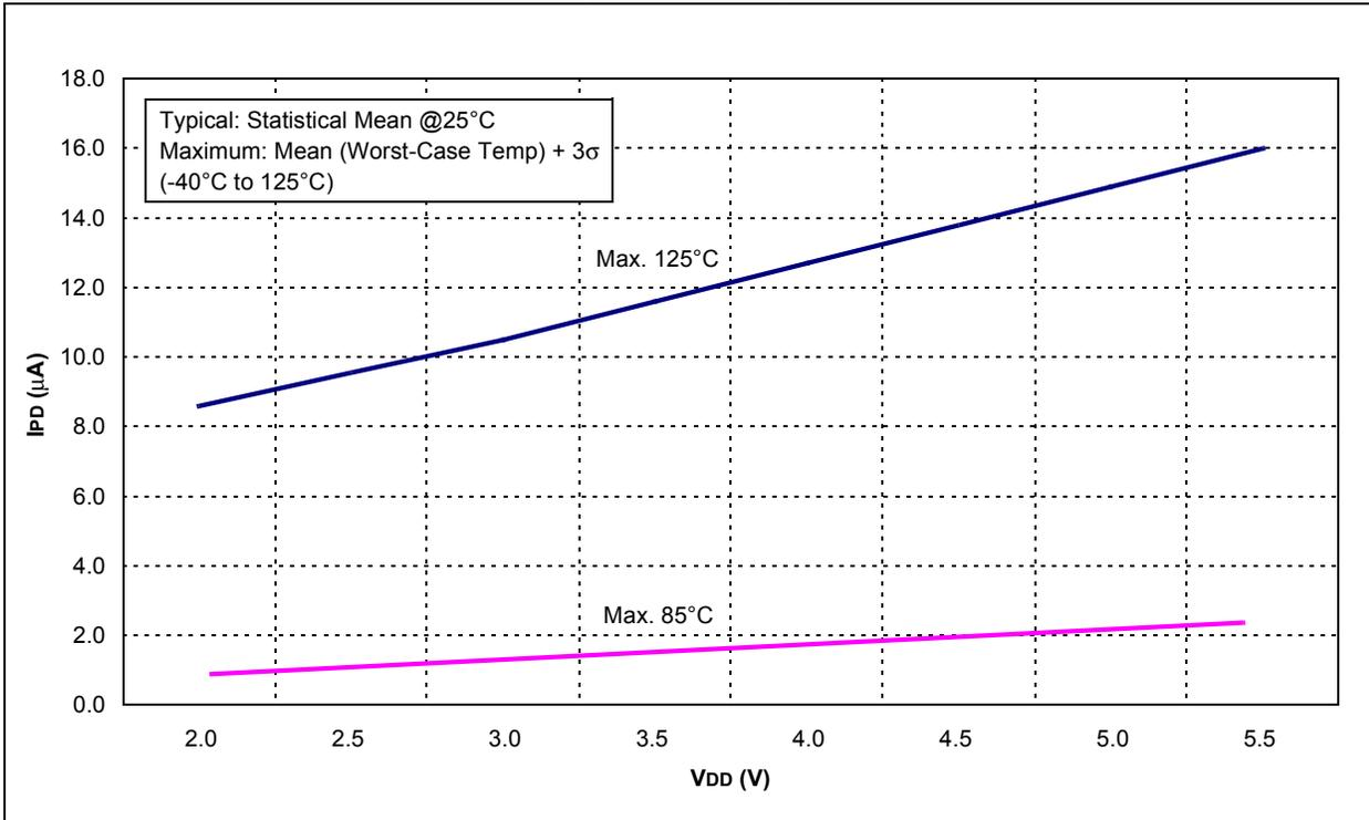
**FIGURE 14-4: COMPARATOR IPD vs. VDD (COMPARATOR ENABLED)**
