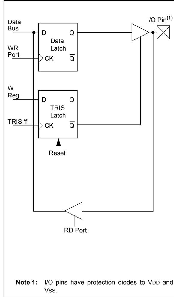
**FIGURE 5-12: BLOCK DIAGRAM OF RC4**
