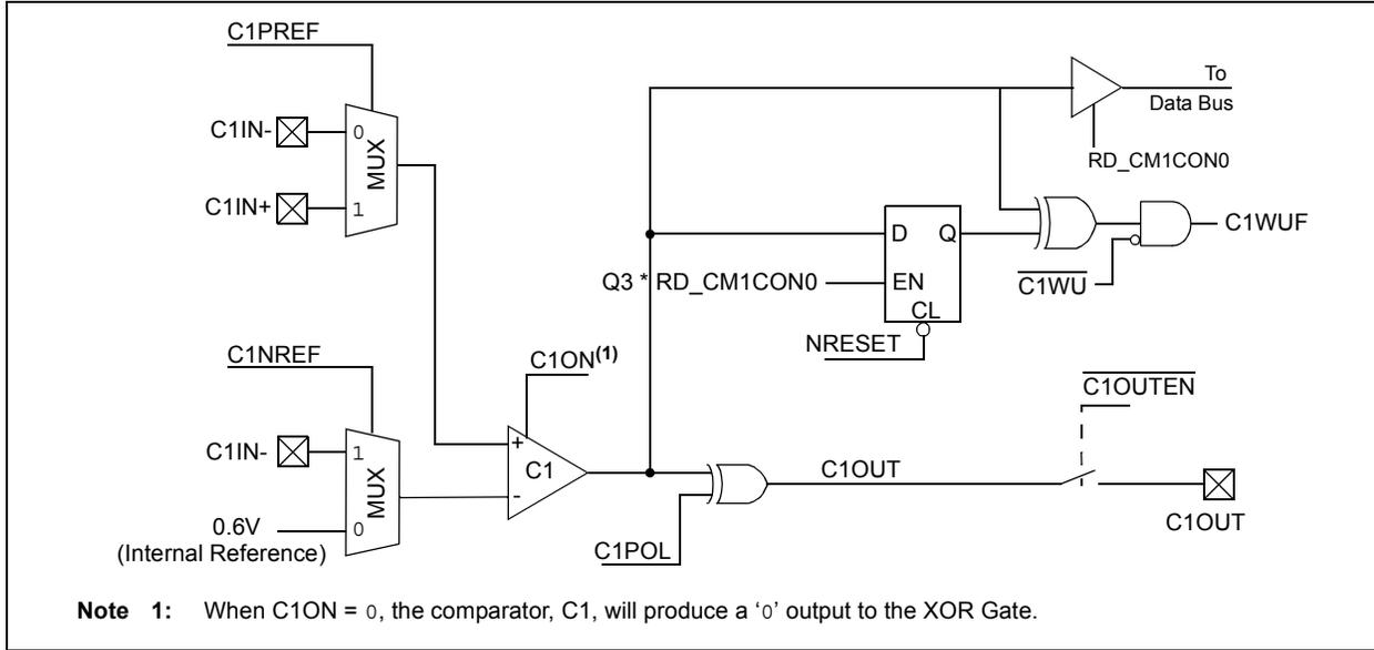
**FIGURE 7-2: COMPARATOR 2 BLOCK DIAGRAM (PIC16F506 ONLY)**
