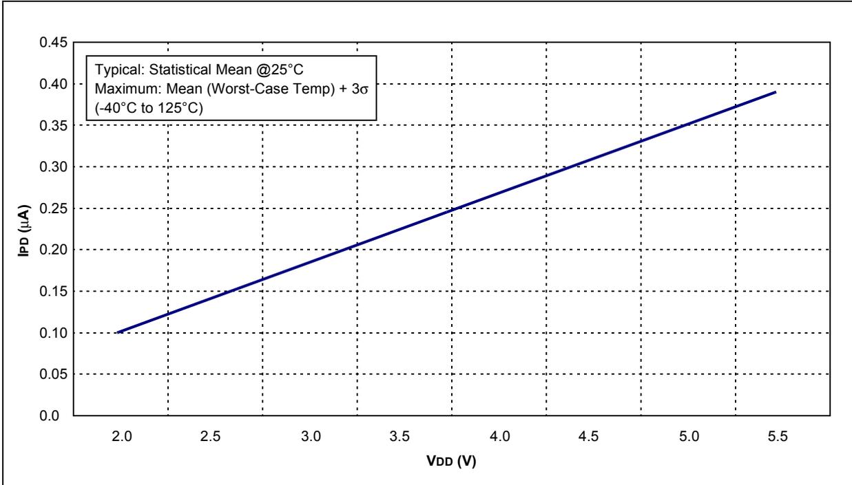
FIGURE 14-3: MAXIMUM  $I_{PD}$  vs.  $V_{DD}$  (SLEEP MODE, ALL PERIPHERALS DISABLED)
