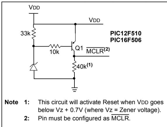
**FIGURE 10-13: BROWN-OUT PROTECTION CIRCUIT 2**
