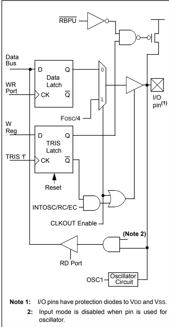
**FIGURE 5-7: BLOCK DIAGRAM OF GP4**
