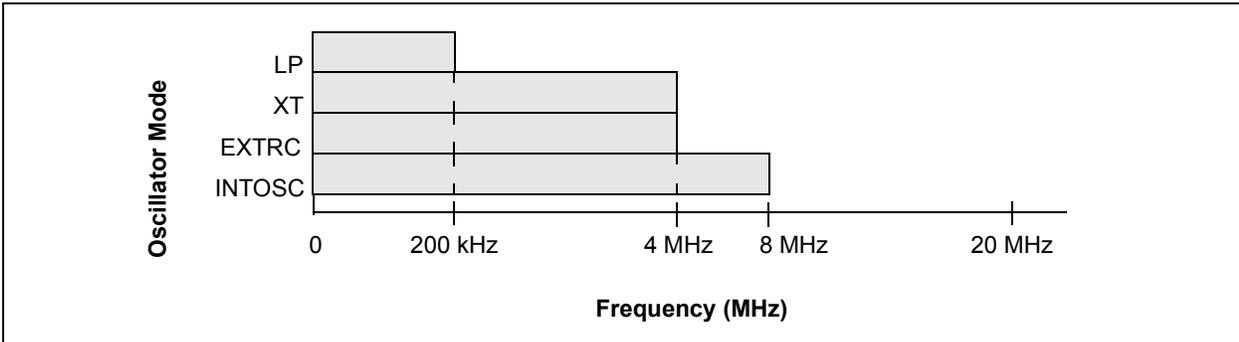
**FIGURE 13-3: VOLTAGE FREQUENCY GRAPH,  $-40^{\circ}\text{C} \leq T_A \leq +125^{\circ}\text{C}$  (PIC16F506)**
