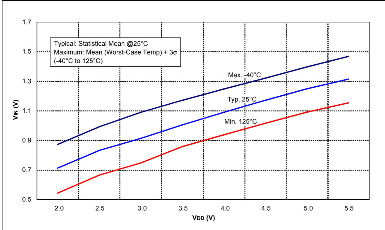
**FIGURE 14-13: SCHMITT TRIGGER INPUT THRESHOLD  $V_{IN}$  vs.  $V_{DD}$**
