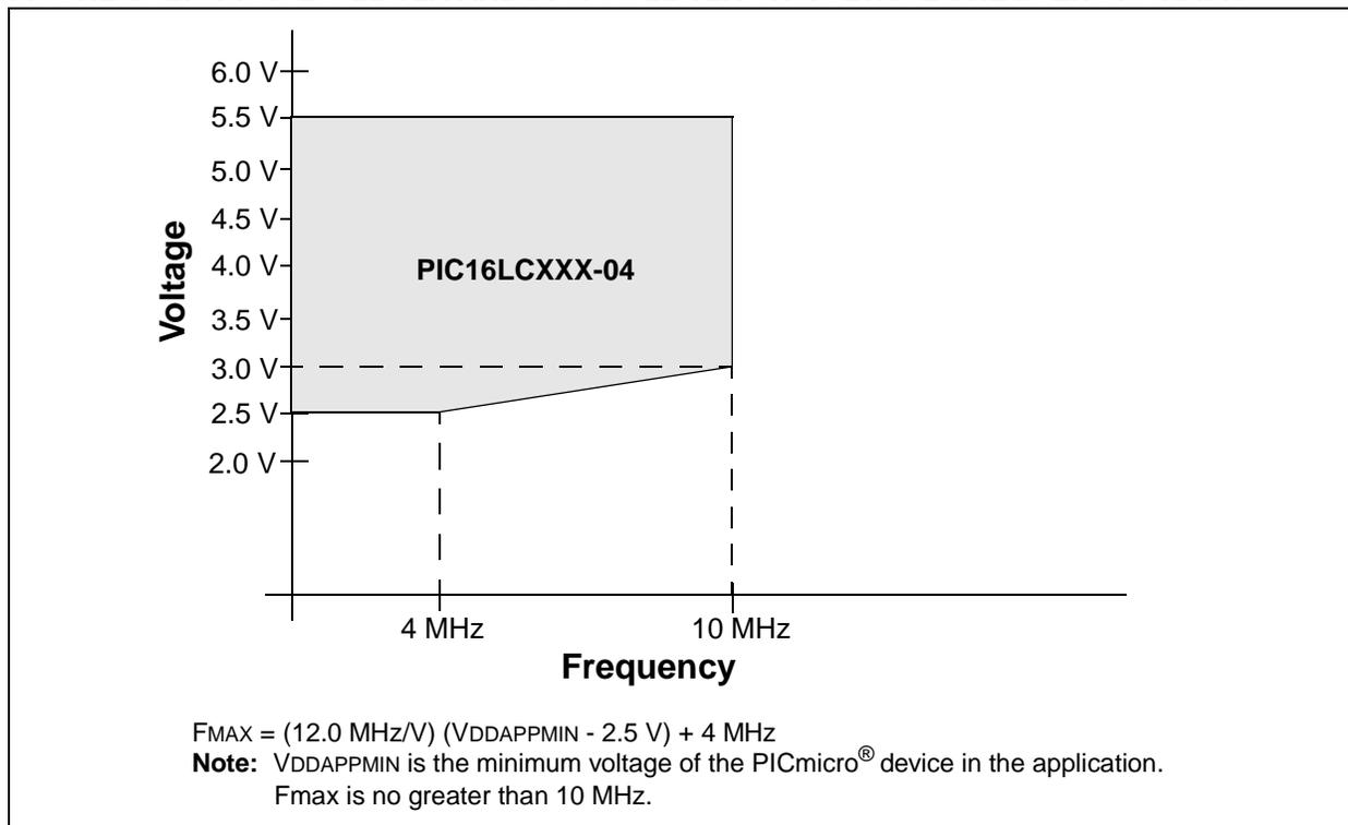
**FIGURE 13-3: PIC16C62B/72A-04 VOLTAGE-FREQUENCY GRAPH**
