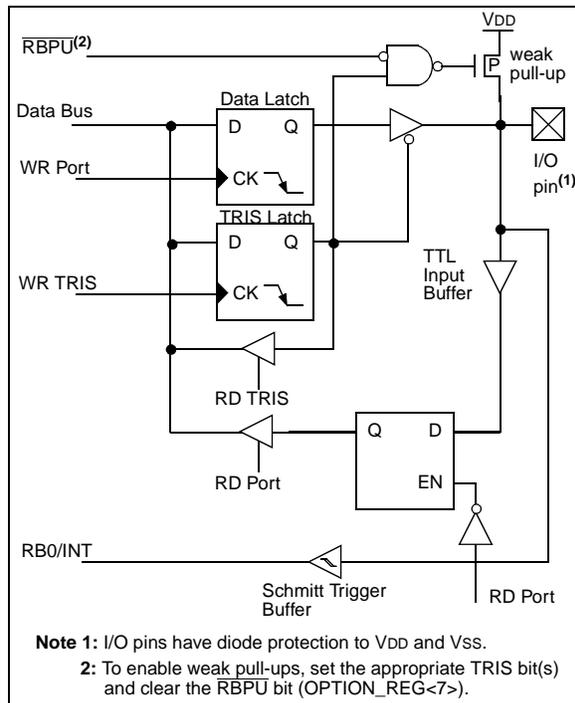
Four of PORTB's pins, RB7:RB4, have an interrupt on change feature. Only pins configured as inputs can cause this interrupt to occur (i.e. any RB7:RB4 pin configured as an output is excluded from the interrupt on change comparison). The input pins (of RB7:RB4) are compared with the old value latched on the last read of PORTB. The "mismatch" outputs of RB7:RB4 are OR'ed together to generate the RB Port Change Interrupt with flag bit RBIF (INTCON<0>).
