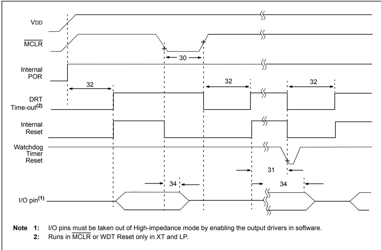
**TABLE 11-3: RESET, WATCHDOG TIMER AND DEVICE RESET TIMER – PIC12F519**
