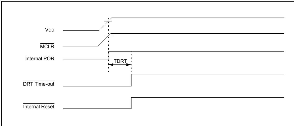
**FIGURE 8-10: TIME-OUT SEQUENCE ON POWER-UP ( $\overline{\text{MCLR}}$  TIED TO  $V_{\text{DD}}$ ): SLOW  $V_{\text{DD}}$  RISE TIME**
