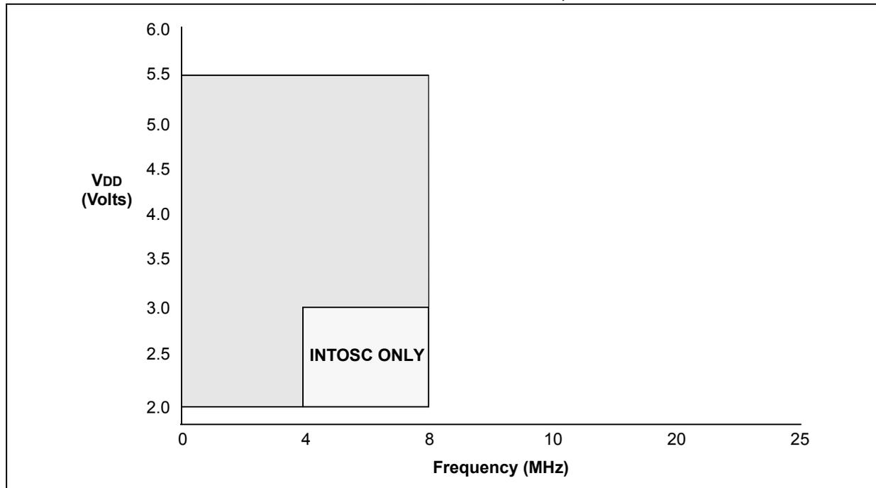
**FIGURE 11-2: MAXIMUM OSCILLATOR FREQUENCY TABLE**
