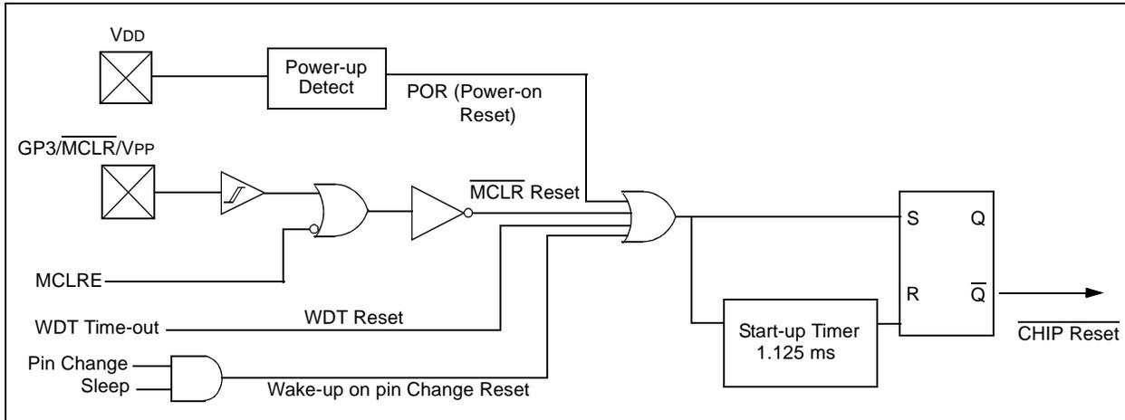
**FIGURE 8-3: TIME-OUT SEQUENCE ON POWER-UP ( $\overline{\text{MCLR}}$  PULLED LOW)**
