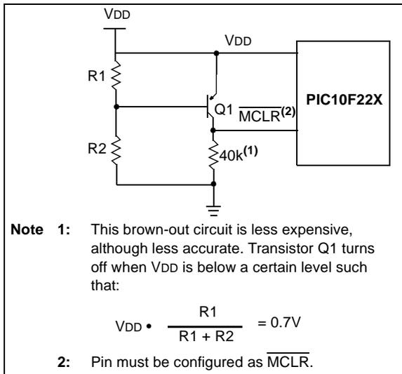
**FIGURE 8-9: BROWN-OUT PROTECTION CIRCUIT 3**
