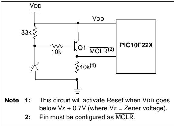
**FIGURE 8-8: BROWN-OUT PROTECTION CIRCUIT 2**
