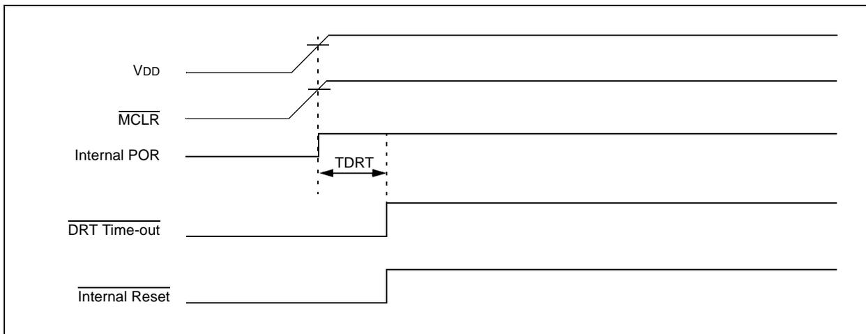
FIGURE 8-5: TIME-OUT SEQUENCE ON POWER-UP ( $\overline{\text{MCLR}}$  TIED TO  $V_{\text{DD}}$ ): SLOW  $V_{\text{DD}}$  RISE TIME
