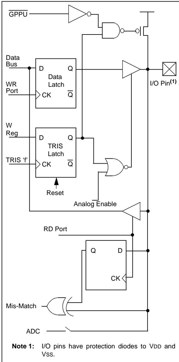
**FIGURE 5-3: BLOCK DIAGRAM OF GP2**
