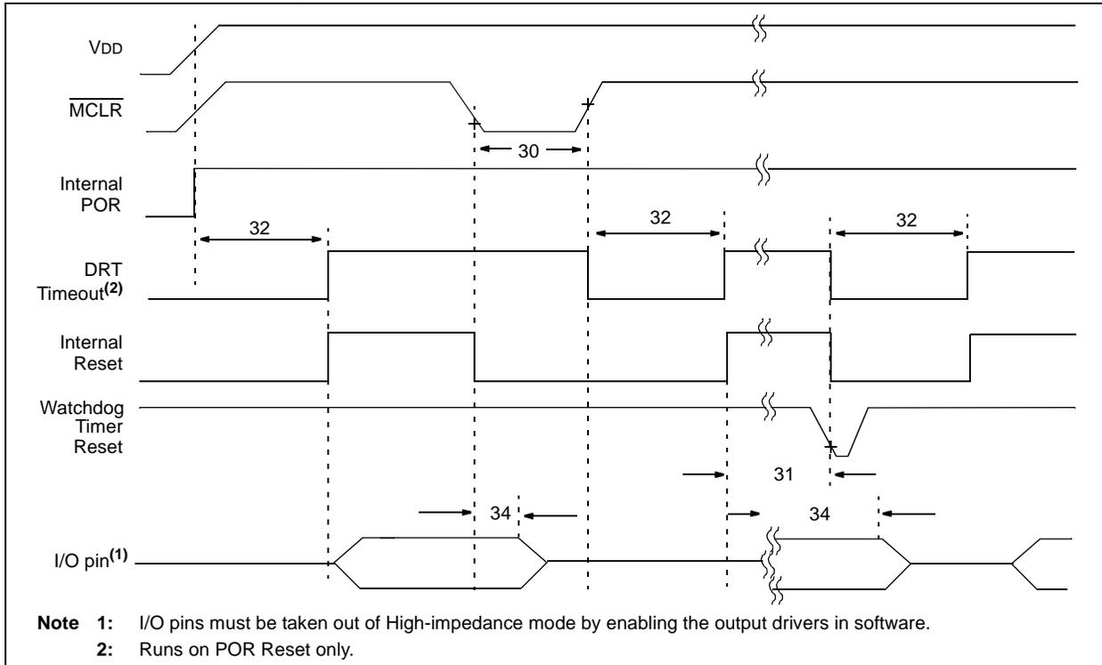
**TABLE 10-3: RESET, WATCHDOG TIMER AND DEVICE RESET TIMER – PIC10F220/222**
