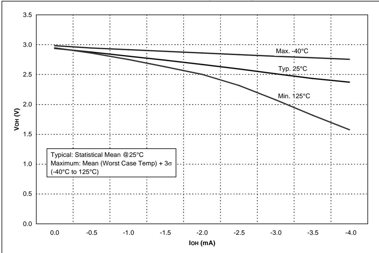
FIGURE 11-11:  $V_{OH}$  vs.  $I_{OH}$  OVER TEMPERATURE ( $V_{DD} = 5.0V$ )
