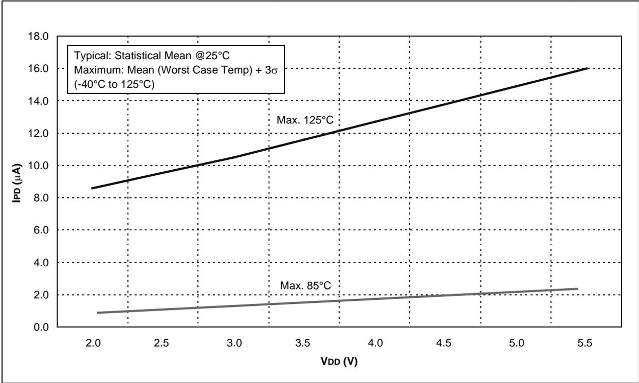
FIGURE 11-5: TYPICAL WDT IPD vs. VDD
