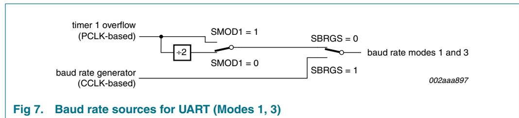
Fig 7. Baud rate sources for UART (Modes 1, 3)
