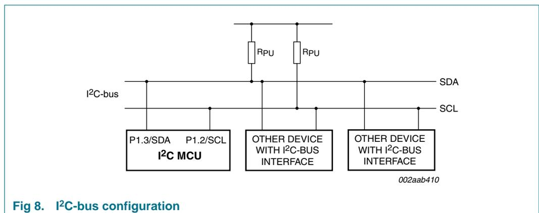
**Fig 8. I<sup>2</sup>C-bus configuration**
