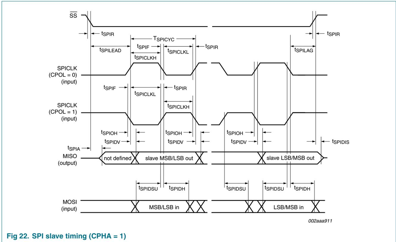
Fig 22. SPI slave timing (CPHA = 1)
