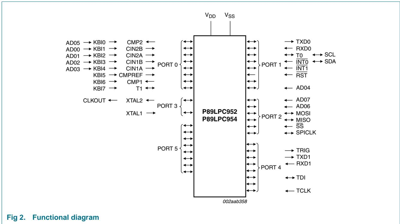
**Fig 2. Functional diagram**
