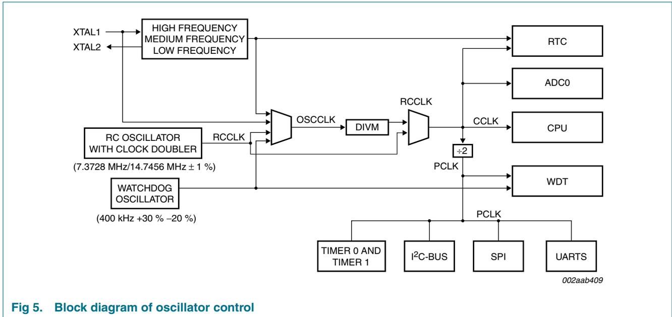
Fig 5. Block diagram of oscillator control
