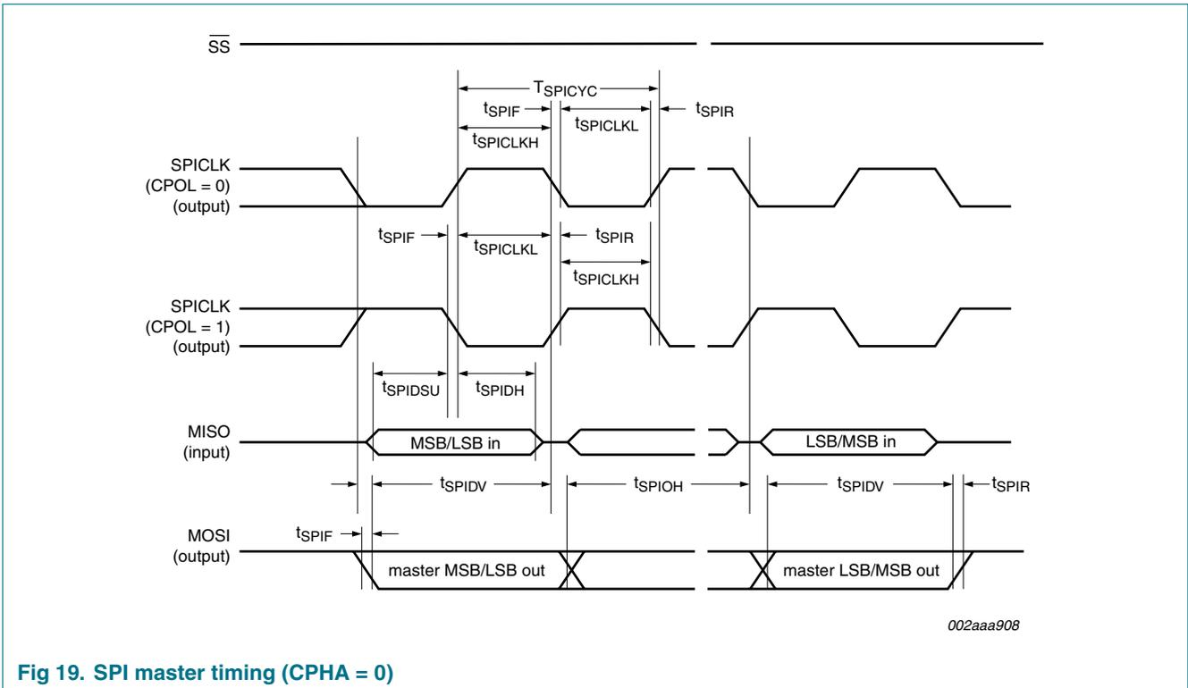
Fig 19. SPI master timing (CPHA = 0)
