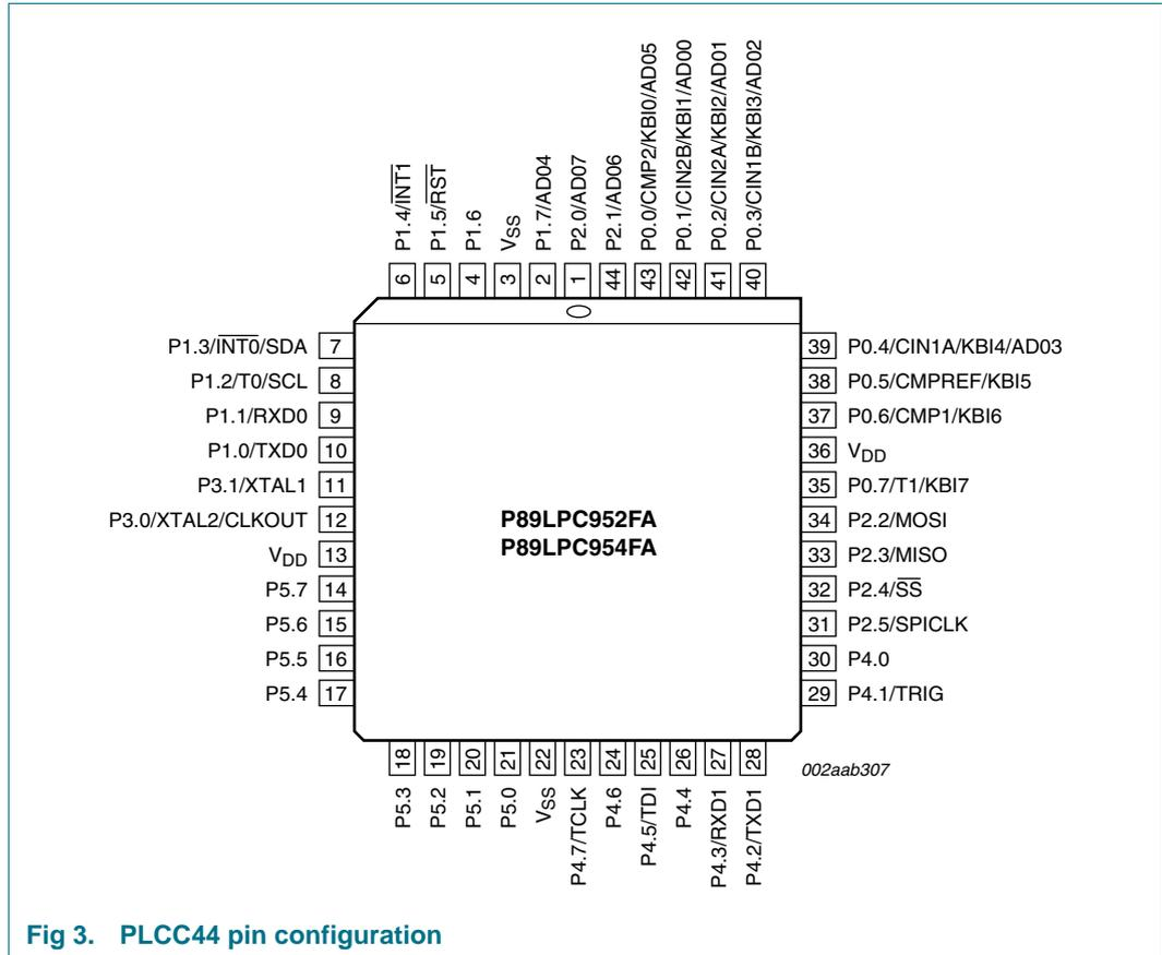
Fig 3. PLCC44 pin configuration
