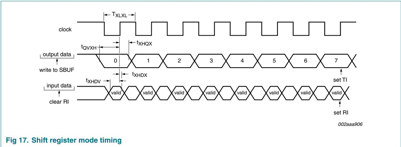
Fig 17. Shift register mode timing
