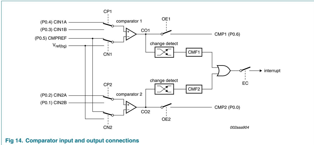
Fig 14. Comparator input and output connections
