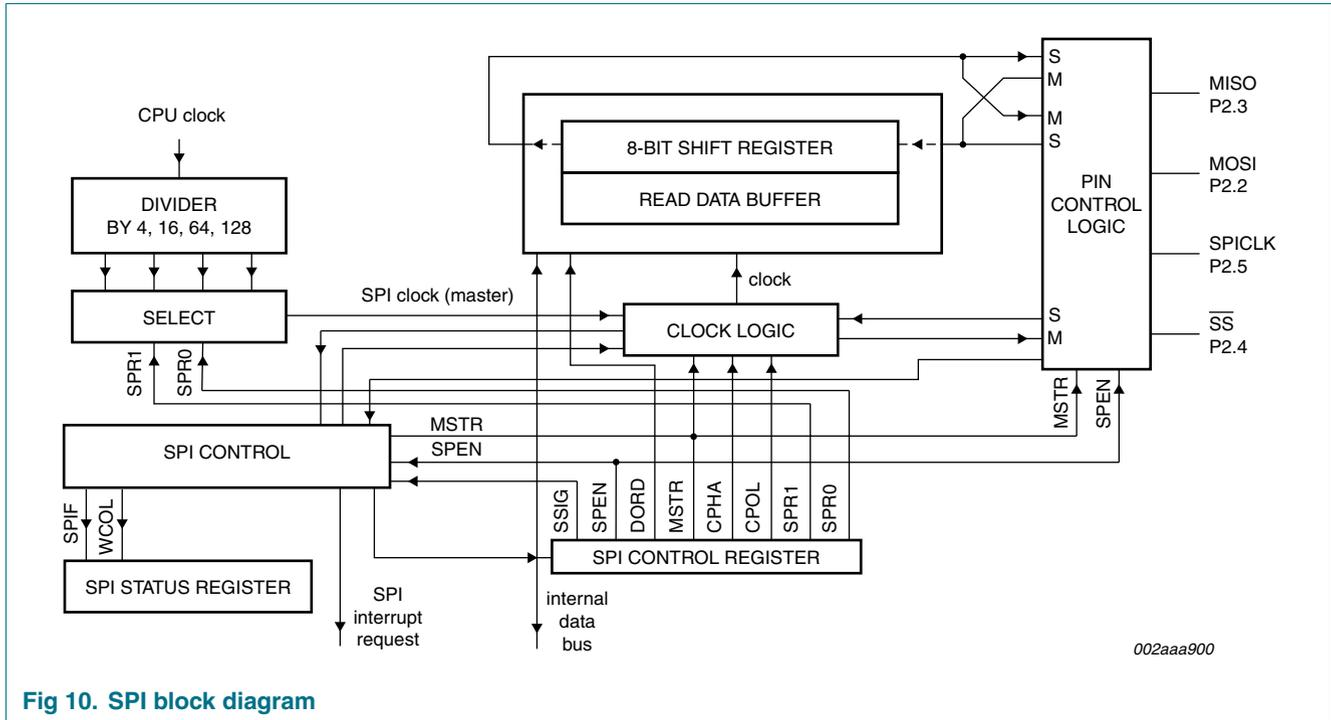
Fig 10. SPI block diagram
