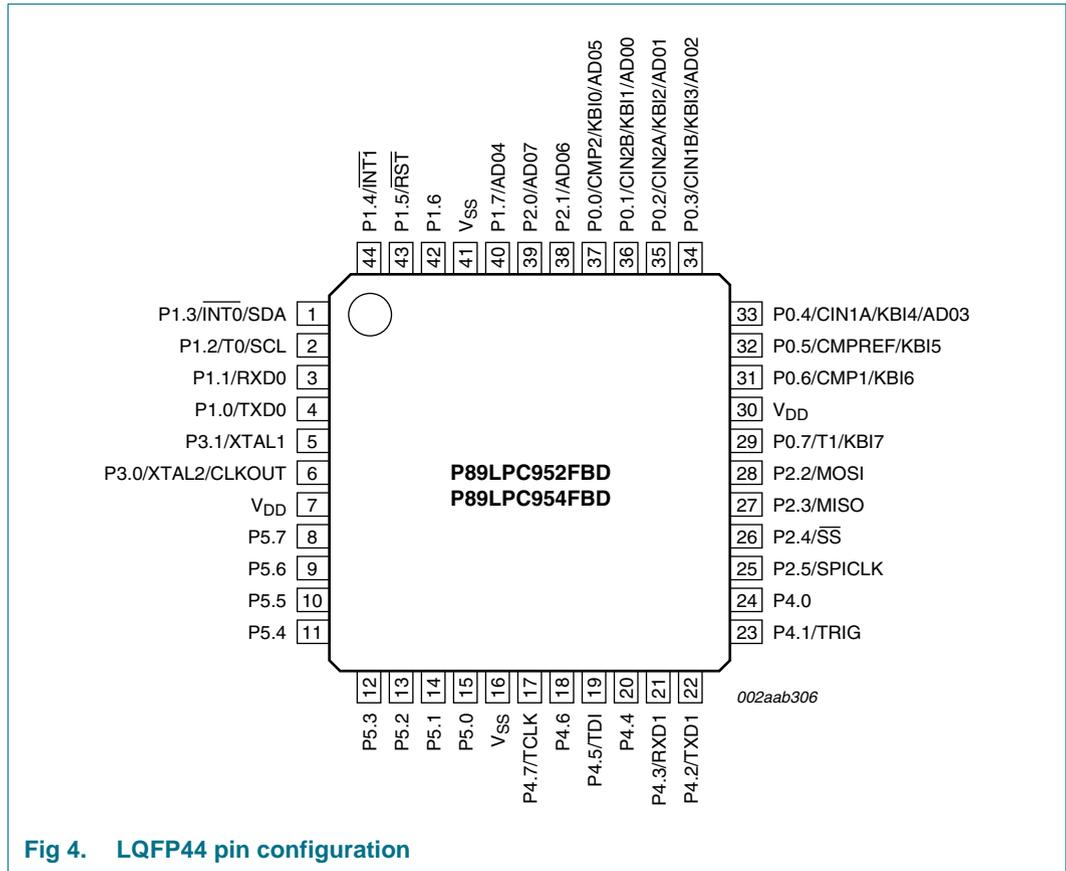
Fig 4. LQFP44 pin configuration
