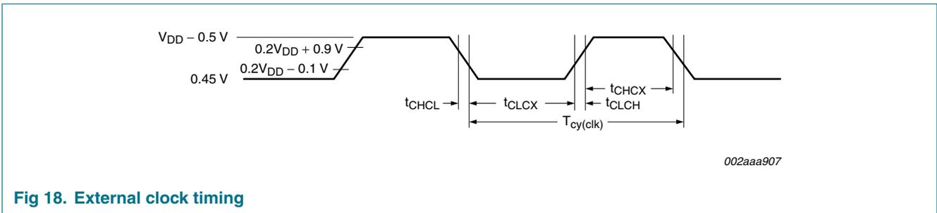
Fig 18. External clock timing
