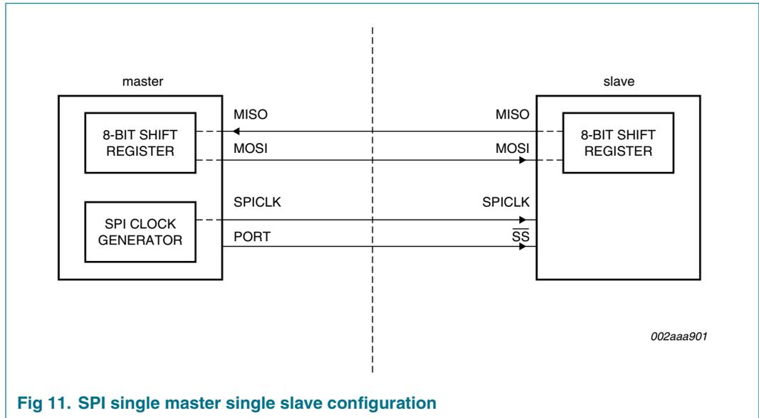
Fig 11. SPI single master single slave configuration
