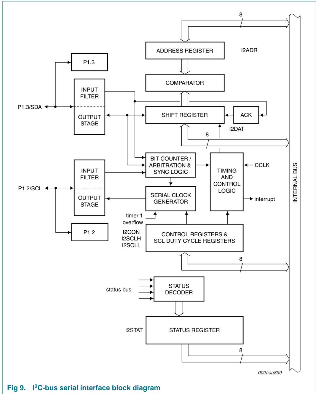
Fig 9. I2C-bus serial interface block diagram
