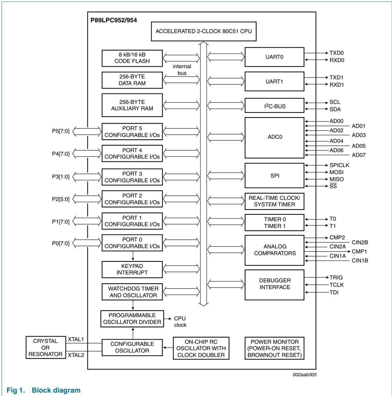
Fig 1. Block diagram
