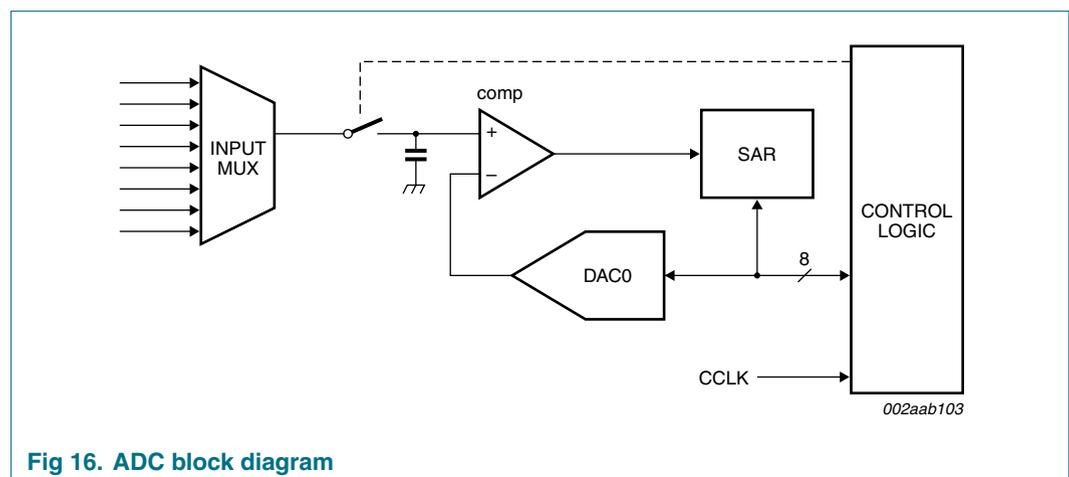
Fig 16. ADC block diagram
