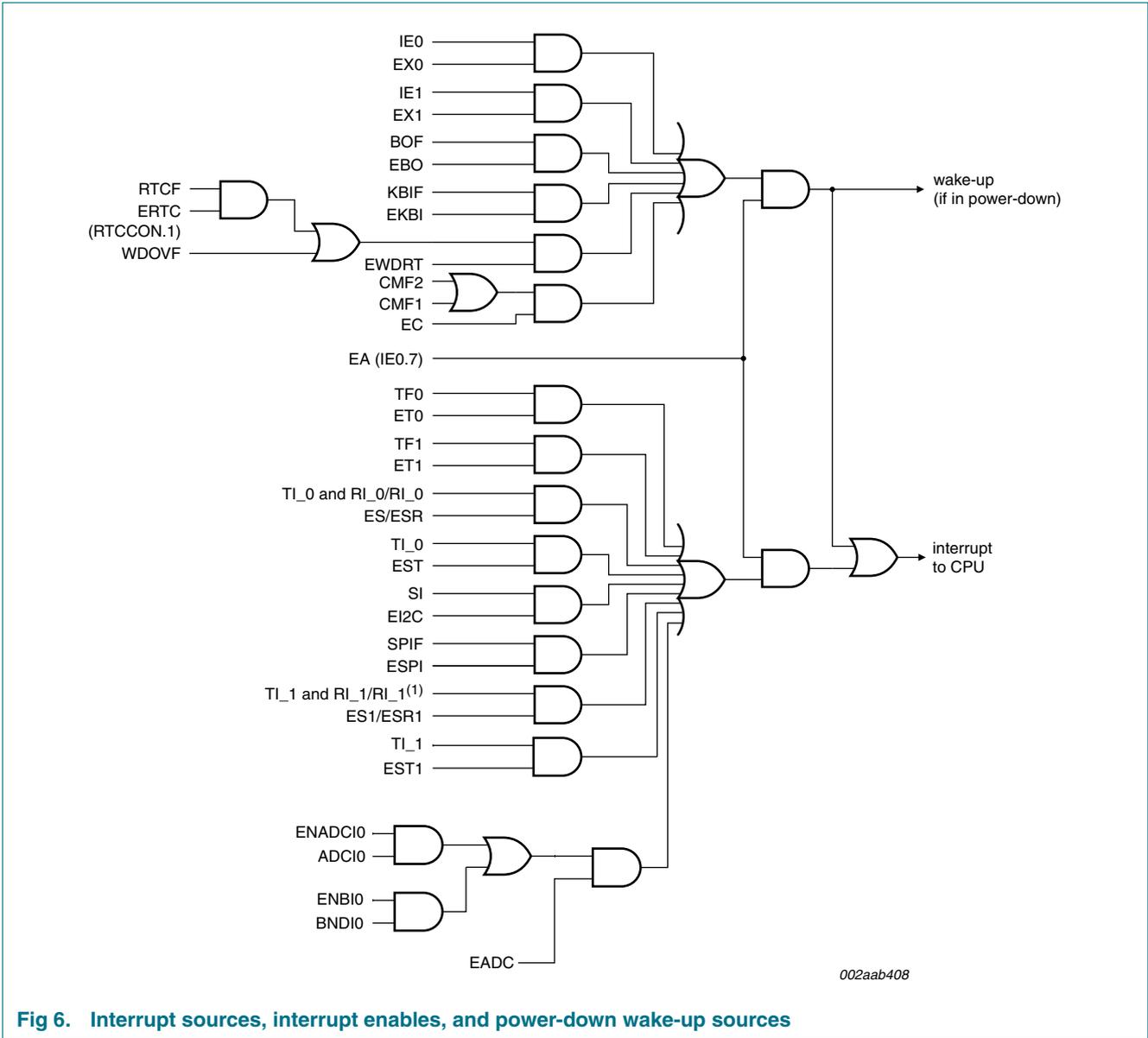
Fig 6. Interrupt sources, interrupt enables, and power-down wake-up sources
