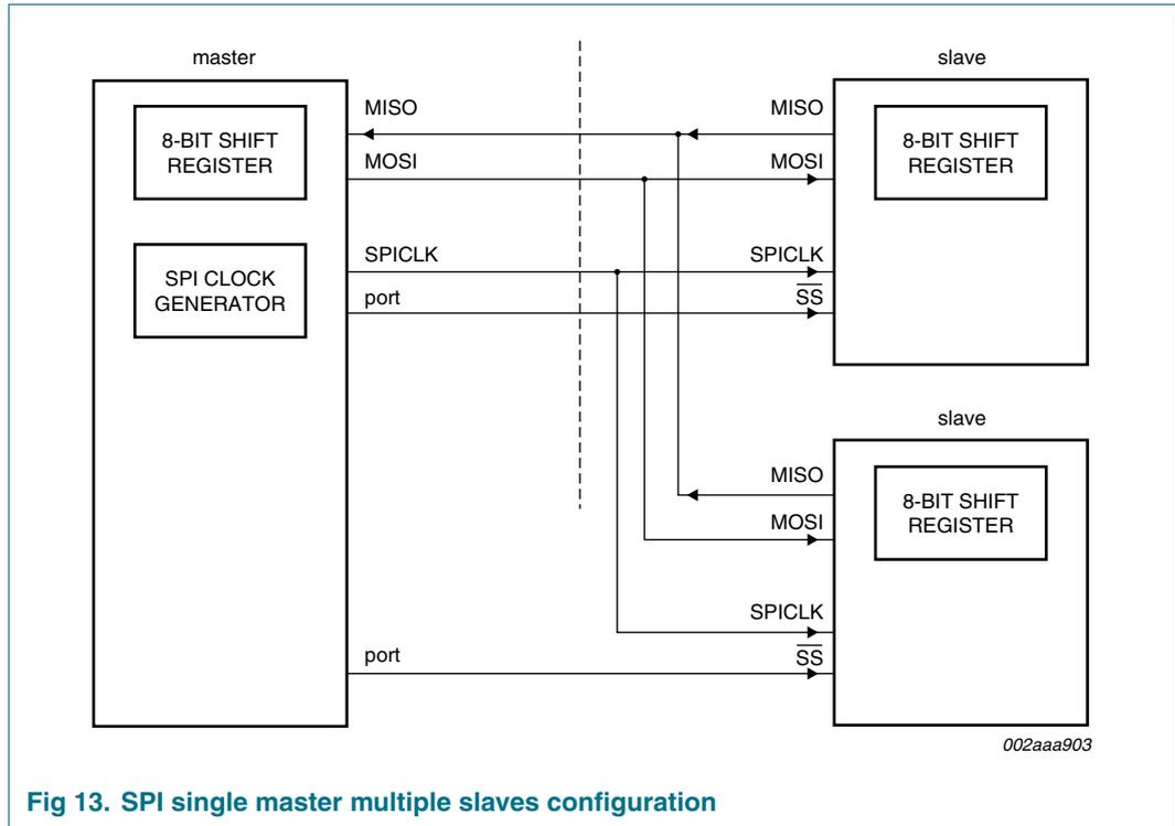
Fig 13. SPI single master multiple slaves configuration
