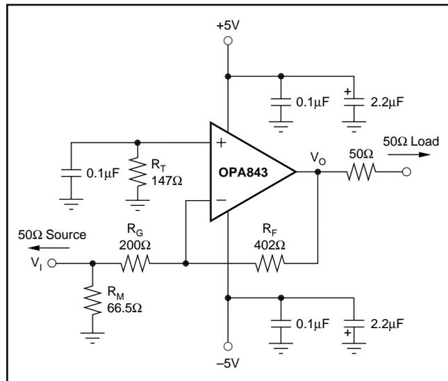
FIGURE 2. Inverting  $G = -2$  Specifications and Test Circuit.
