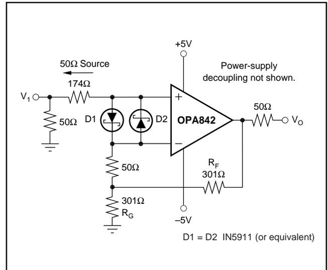
FIGURE 9. Gain of +2 with Input Protection.
