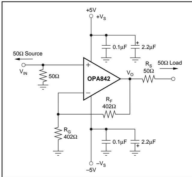
FIGURE 1. Gain of +2. High-frequency application and characterization circuit.
