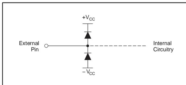
**Figure 11. Internal ESD Protection**
