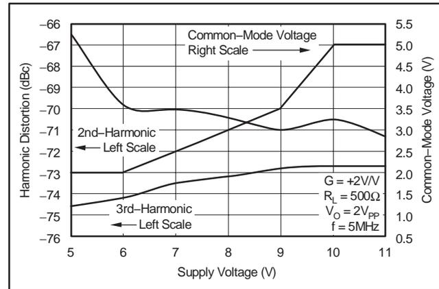
Figure 9. 5MHz Harmonic Distortion vs Supply Voltage
