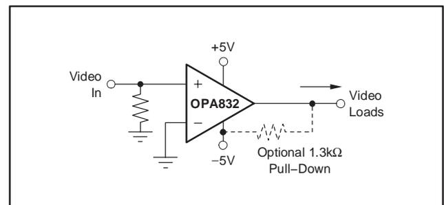
Figure 4. Gain of  $+2V/V$  Video Line Driver
