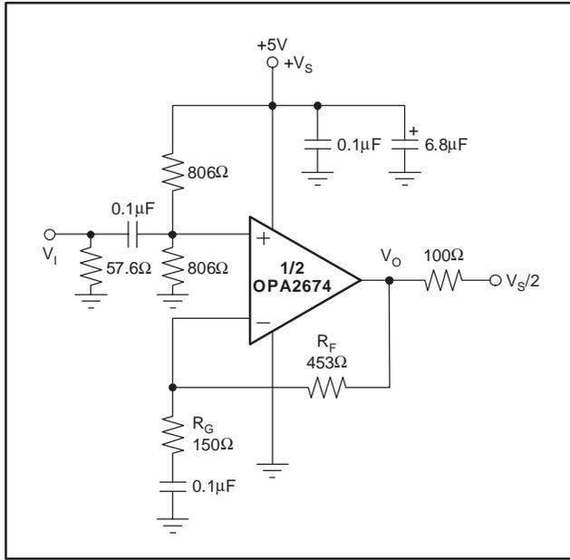
**Figure 3. AC-Coupled, G = +4, Single-Supply, Specification and Test Circuit**
