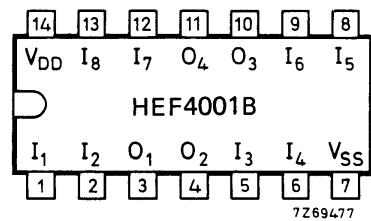
Fig.2 Pinning diagram.
