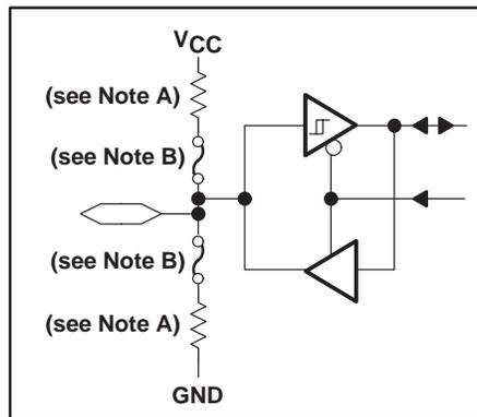
I/O WITH SCHMITT-TRIGGER INPUT (P0.x,
