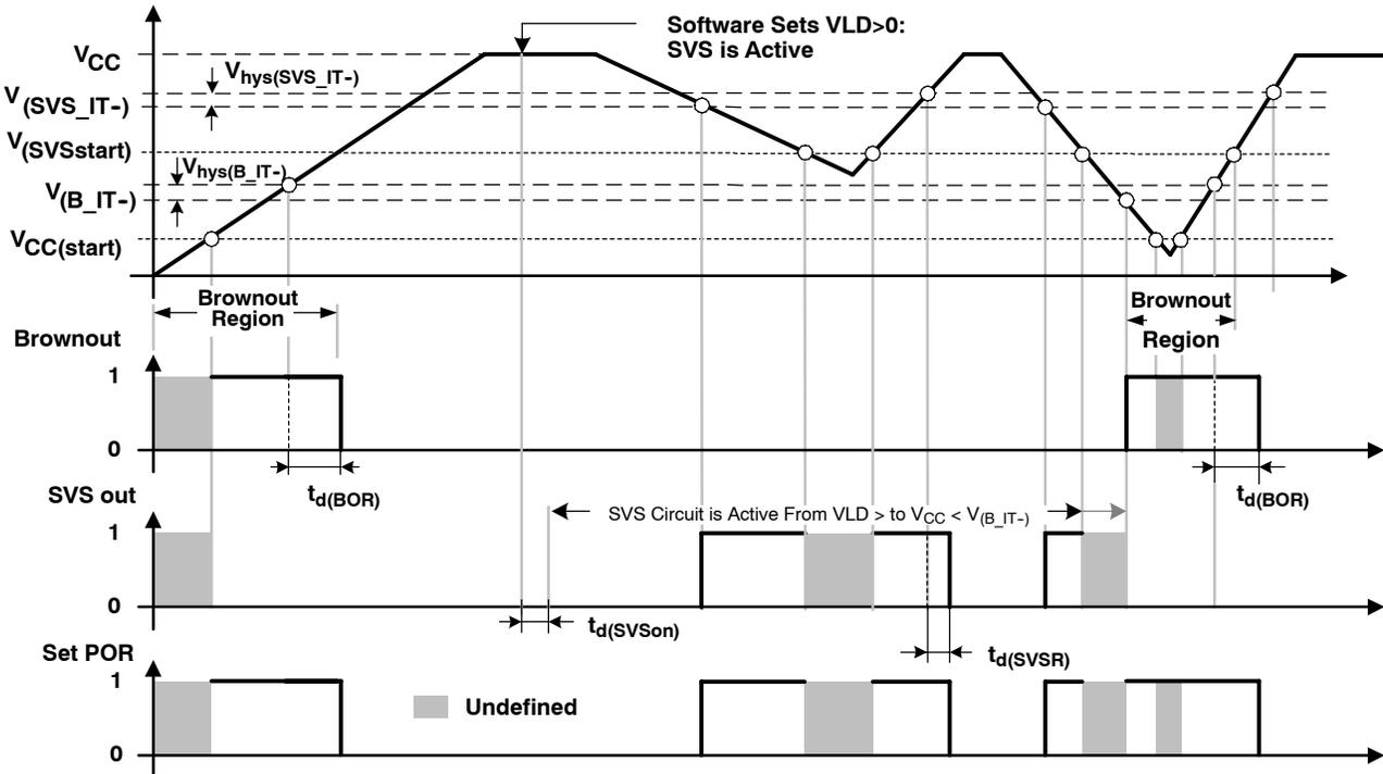
Figure 9. SVS Reset (SVSR) vs Supply Voltage
