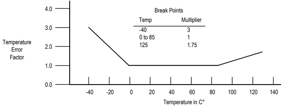
NOTE: The Temperature Multiplier is a linear response from 0°C to -40°C and from 85°C to 125°C
