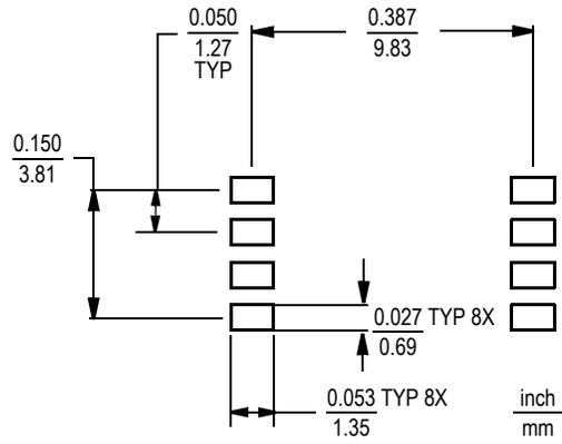
Figure 5. SSOP Footprint (Case 1317 and 1317A)
