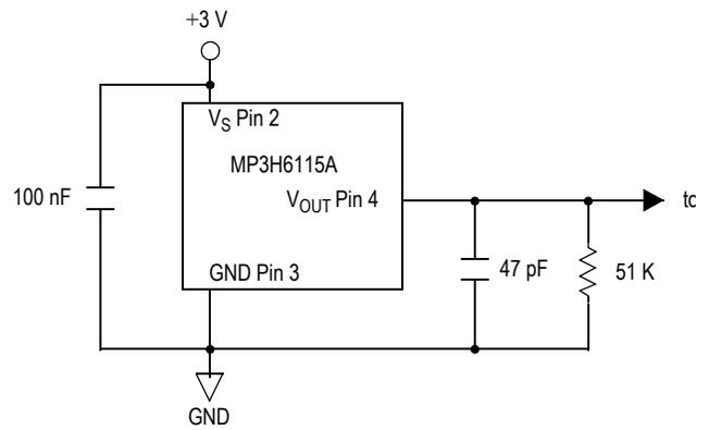
**Figure 3. Typical Application Circuit (Output Source Current Operation)**
