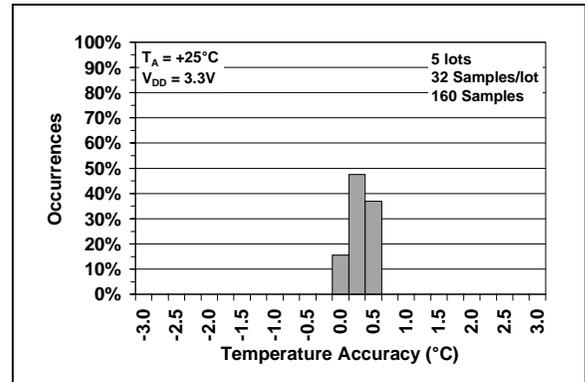
**FIGURE 2-4:** Temperature Accuracy Histogram,  $T_A = +25^\circ C$ .
