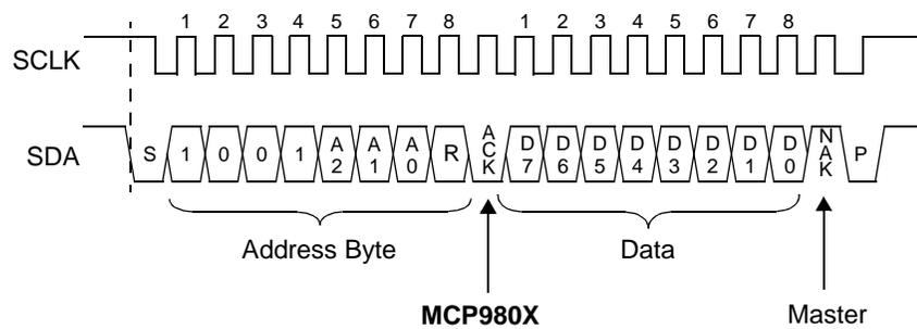
**Note:** User can continue to receive 1-byte data indefinitely from a previously set register pointer.
