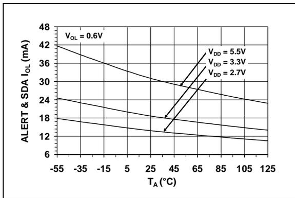
**FIGURE 2-7:** ALERT and SDA  $I_{OL}$  vs. Ambient Temperature.
