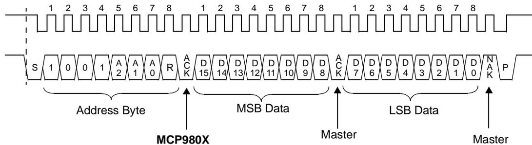
**Note:** User can continue to receive 2-byte data indefinitely from a previously set register pointer.
