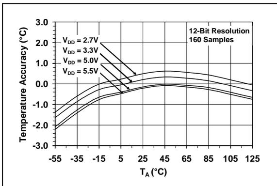
**FIGURE 2-2:** Average Temperature Accuracy vs. Ambient Temperature.
