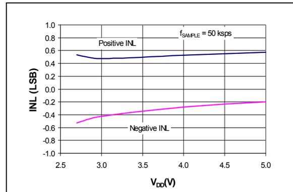
**FIGURE 2-5:** Integral Nonlinearity (INL) vs.  $V_{DD}$ .
