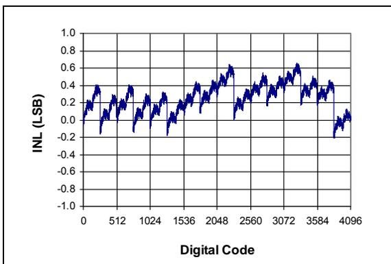
**FIGURE 2-3:** Integral Nonlinearity (INL) vs. Code (Representative Part).
