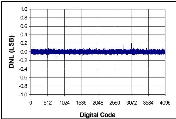
**FIGURE 2-13:** Differential Nonlinearity (DNL) vs. Code (Representative Part).
