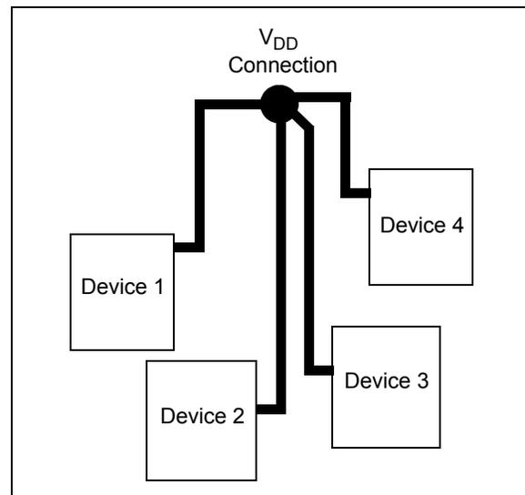
**FIGURE 6-4:** V<sub>DD</sub> traces arranged in a 'Star' configuration in order to reduce errors caused by current return paths.
