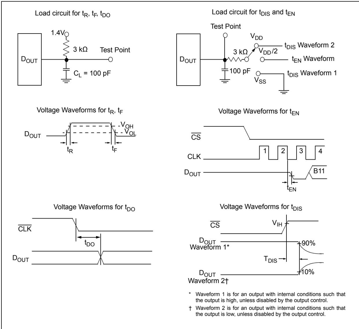
**FIGURE 1-2:** Test Circuits.
