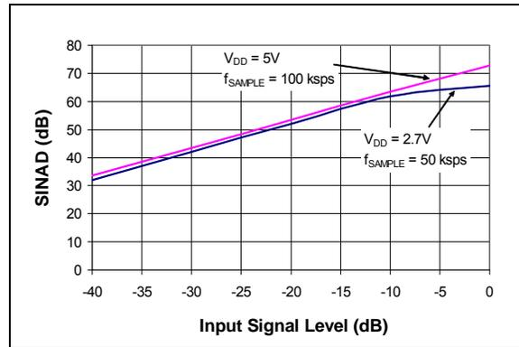
**FIGURE 2-24:** Signal-to-Noise and Distortion (SINAD) vs. Signal Level.
