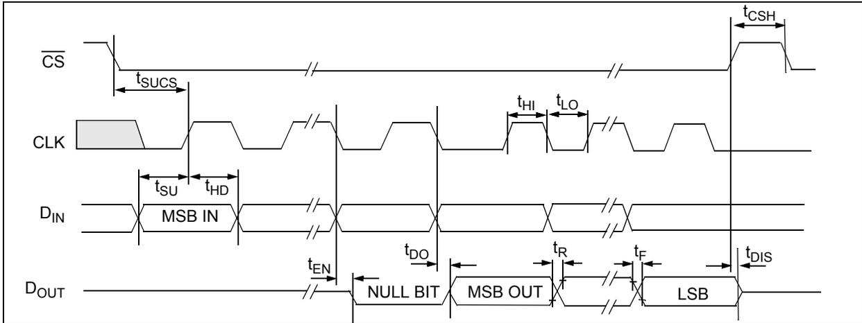
**FIGURE 1-1:** Serial Timing.
