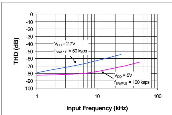
**FIGURE 2-21:** Total Harmonic Distortion (THD) vs. Input Frequency.
