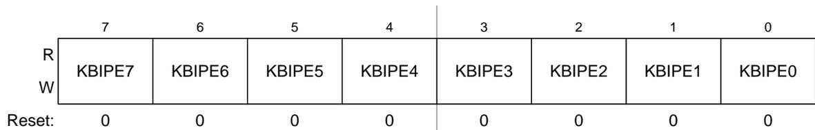
Figure 12-4. KBI Pin Enable Register
