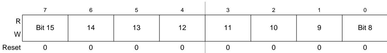
**Figure 15-13. TPM Channel Value Register High (TPMxCnVH)**
