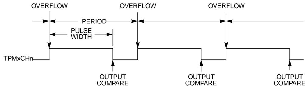
Figure 15-15. PWM Period and Pulse Width (ELSnA=0)
