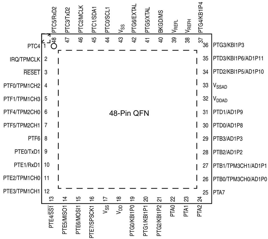
Figure 2-2. MC9S08AC60 Series in 48-Pin QFN Package
