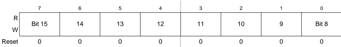
Figure 15-10. TPM Counter Modulo Register High (TPMxMODH)
