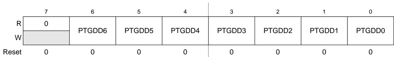
Figure 6-33. Data Direction for Port G (PTGDD)
