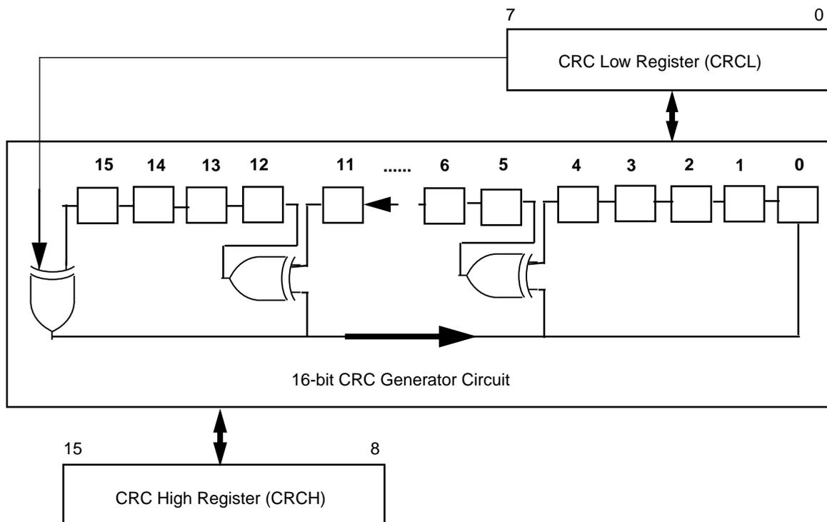
Figure 8-2. Cyclic Redundancy Check (CRC) Module Block Diagram
