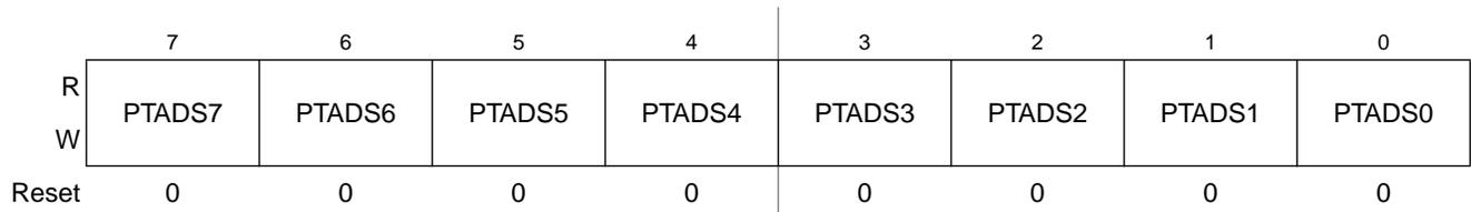
Figure 6-6. Drive Strength Selection for Port A (PTADS)
