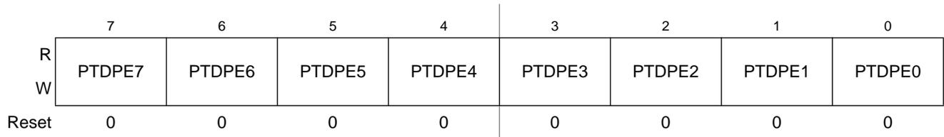
Figure 6-19. Internal Pullup Enable for Port D (PTDPE)
