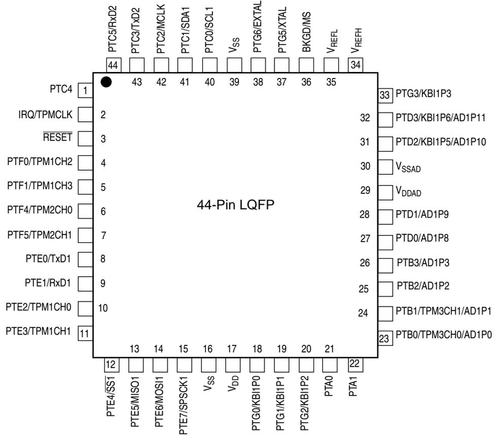
Figure 2-3. MC9S08AC60 Series in 44-Pin LQFP Package
