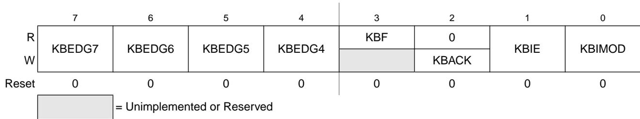
Figure 12-3. KBI Status and Control Register (KBISC)
