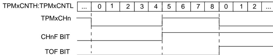
**Figure 15-4. Low-True Pulse of an Edge-Aligned PWM**
