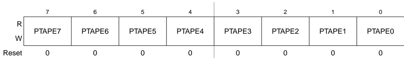
Figure 6-4. Internal Pullup Enable for Port A (PTAPE)
