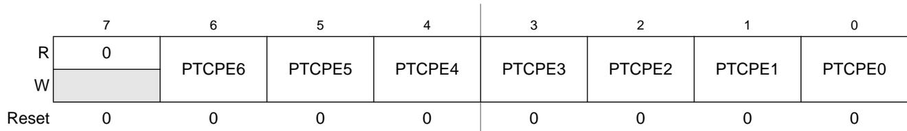
Figure 6-14. Internal Pullup Enable for Port C (PTCPE)
