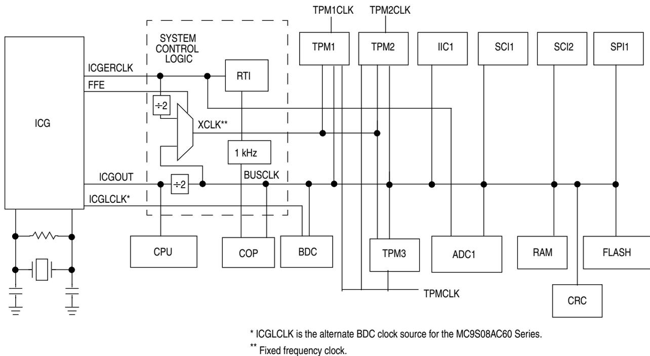
**Figure 1-2. System Clock Distribution Diagram**
