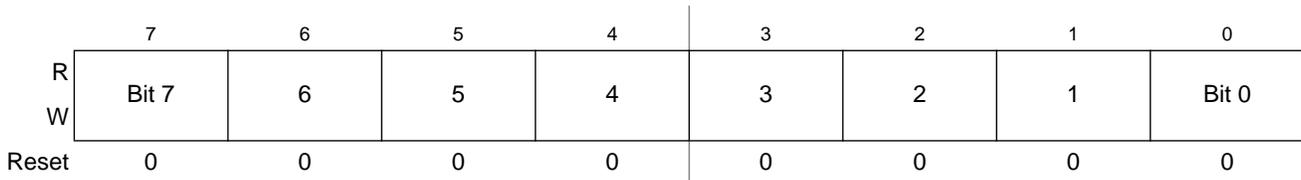
Figure 15-11. TPM Counter Modulo Register Low (TPMxMODL)
