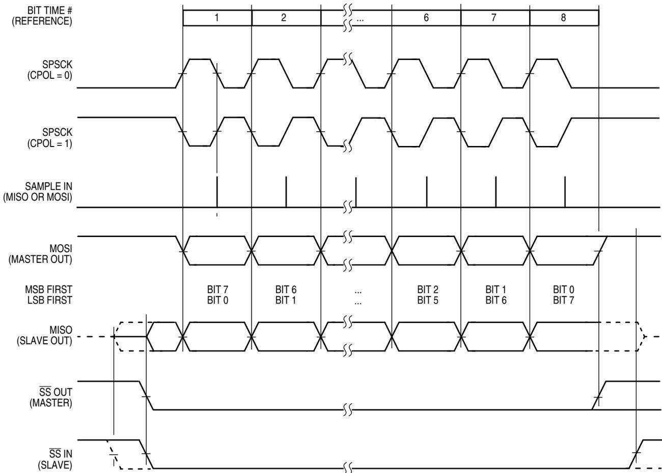
Figure 14-10. SPI Clock Formats (CPHA = 1)
