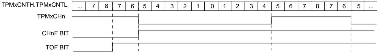
Figure 15-6. Low-True Pulse of a Center-Aligned PWM
