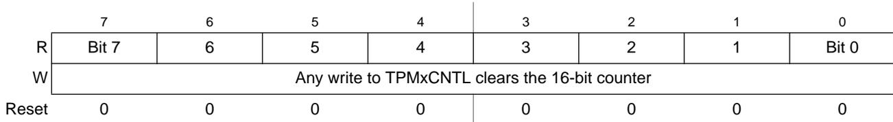
**Figure 15-9. TPM Counter Register Low (TPMxCNTL)**
