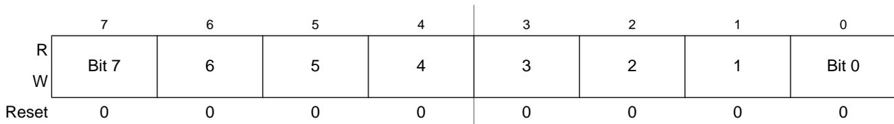
**Figure 15-14. TPM Channel Value Register Low (TPMxCnVL)**
