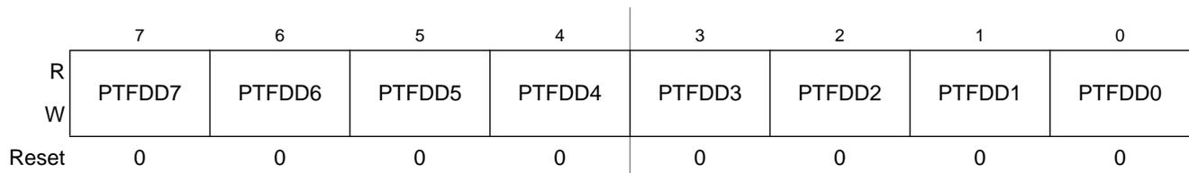
Figure 6-28. Data Direction for Port F (PTFDD)
