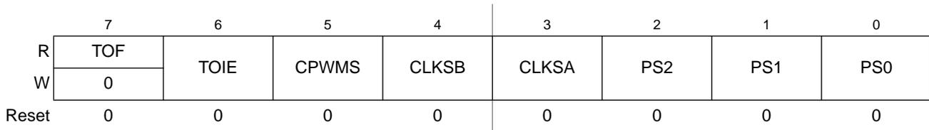
Figure 15-7. TPM Status and Control Register (TPMxSC)
