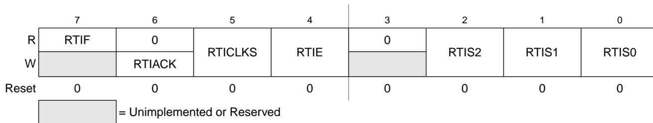
Figure 5-9. System RTI Status and Control Register (SRTISC)
