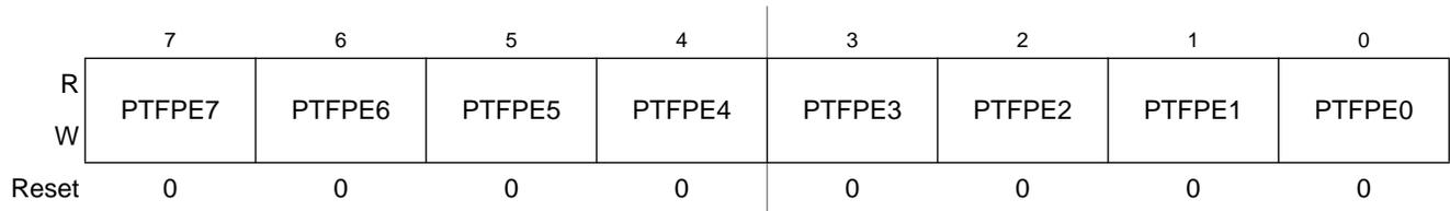
Figure 6-29. Internal Pullup Enable for Port F (PTFPE)
