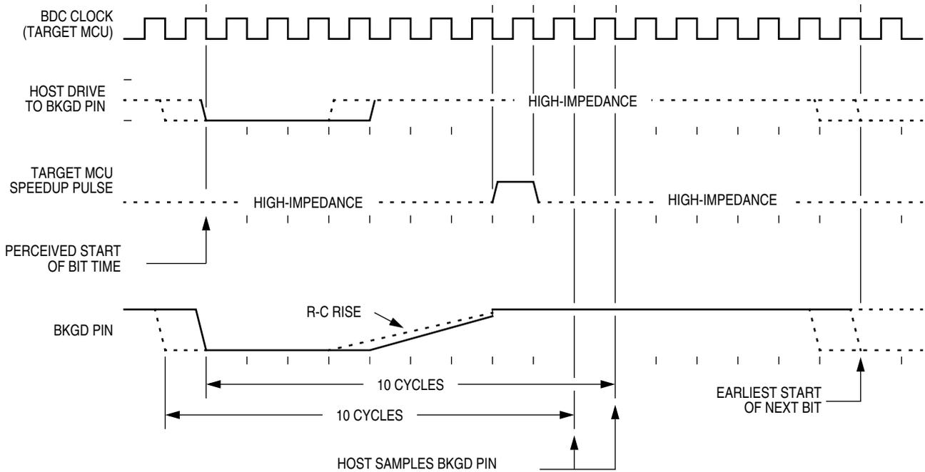
Figure 16-3. BDC Target-to-Host Serial Bit Timing (Logic 1)
