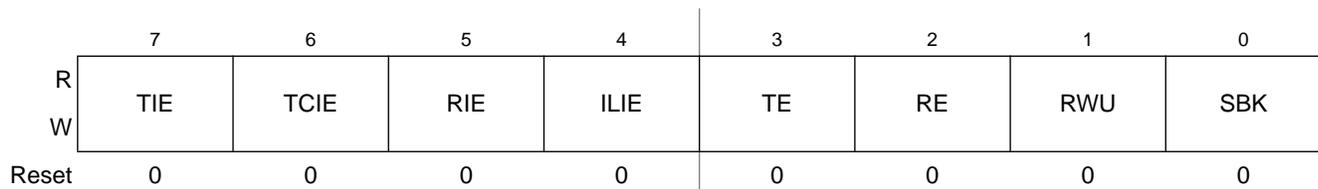
Figure 13-7. SCI Control Register 2 (SC1xC2)
