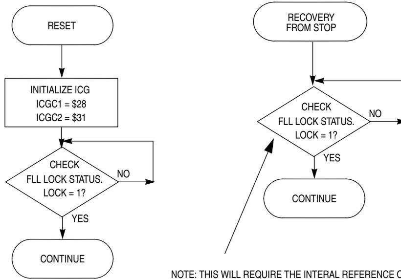
**Figure 10-16. ICG Initialization and Stop Recovery for Example #3**
