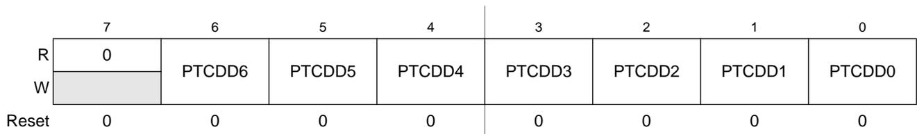
Figure 6-13. Data Direction for Port C (PTCDD)
