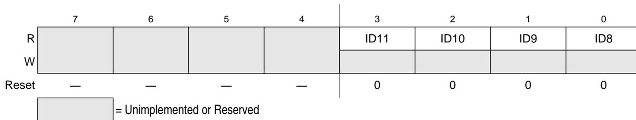
**Figure 5-7. System Device Identification Register — High (SDIDH)**
