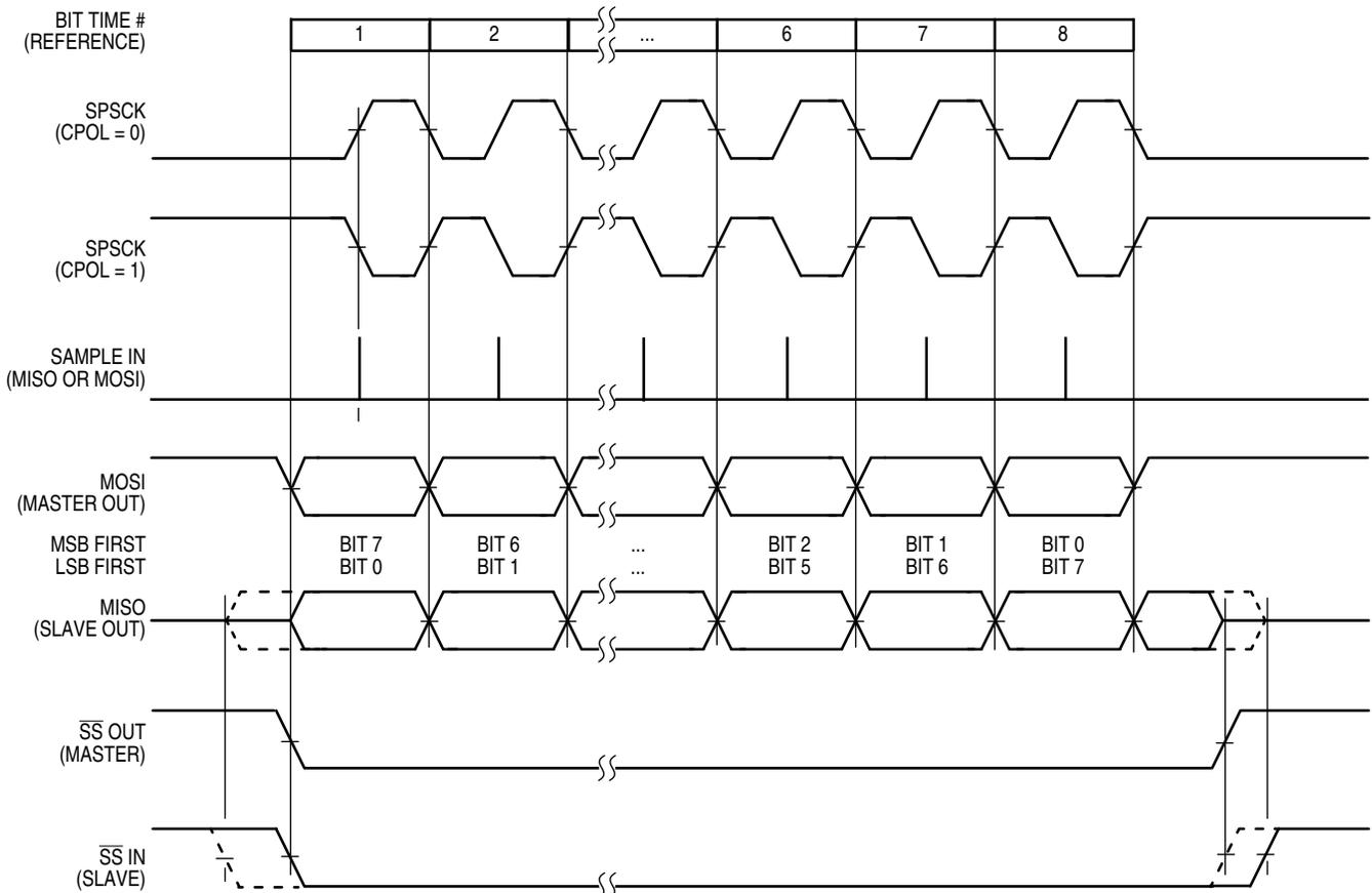
Figure 14-11. SPI Clock Formats (CPHA = 0)
