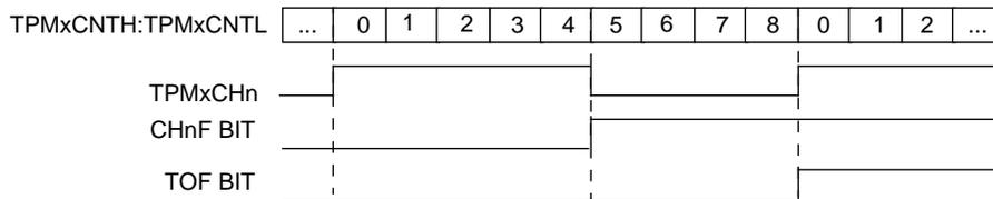
**Figure 15-3. High-True Pulse of an Edge-Aligned PWM**
