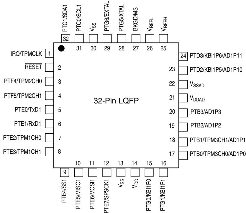
Figure 2-4. MC9S08AC60 Series in 32-Pin LQFP Package
