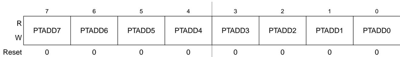
Figure 6-3. Data Direction for Port A Register (PTADD)
