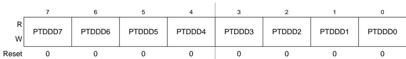
Figure 6-18. Data Direction for Port D (PTDDD)
