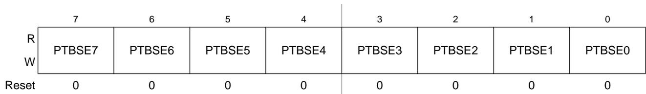
Figure 6-10. Output Slew Rate Control Enable (PTBSE)
