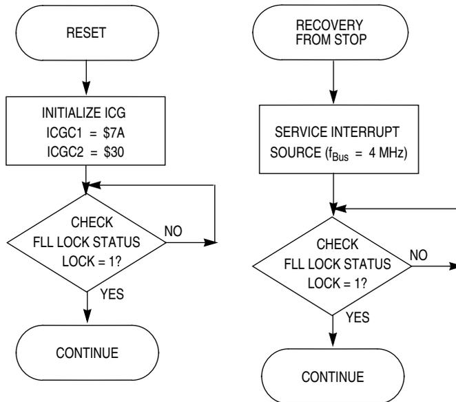
Figure 10-15. ICG Initialization and Stop Recovery for Example #2
