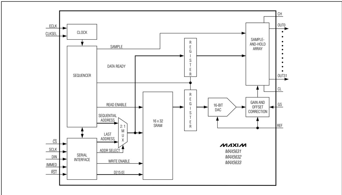
Figure 1. Functional Diagram
