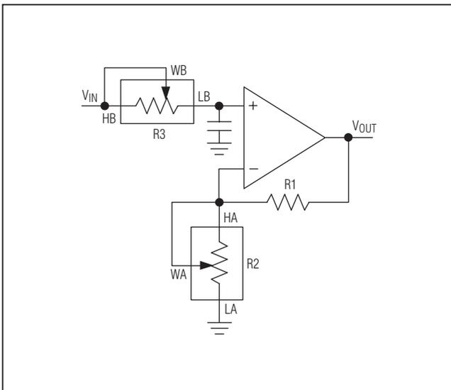
Figure 10. Programmable Filter
