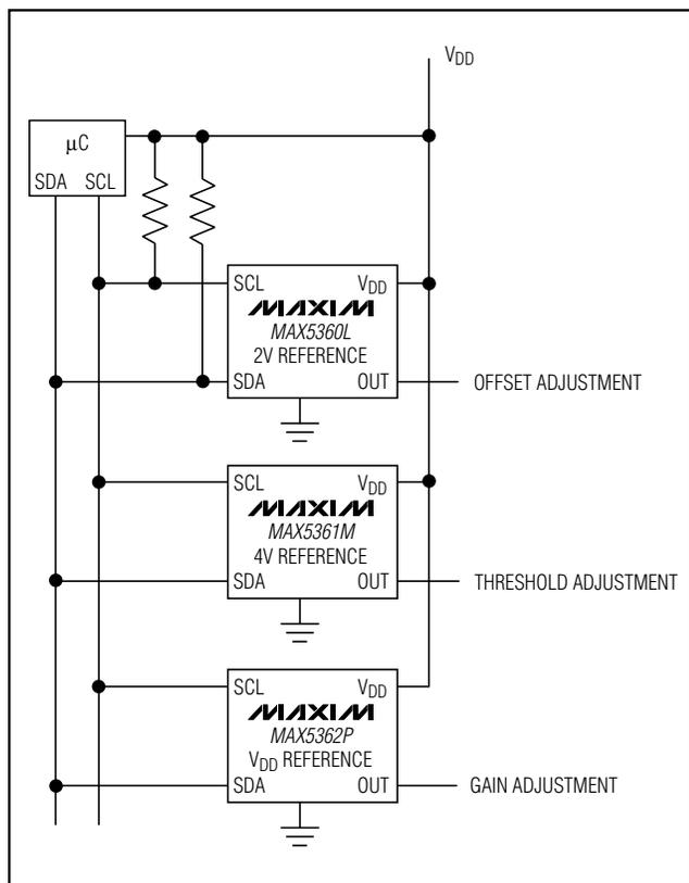
Figure 7. I<sup>2</sup>C Typical Application
