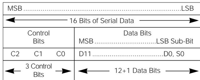
Figure 4. Serial-Data Format
