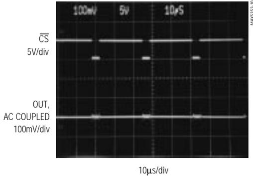
DIGITAL FEEDTHROUGH ( $f_{SCLK} = 100kHz$ )
