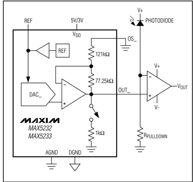
Figure 8. Digital Calibration
