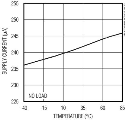
**ONE-DAC SHUTDOWN SUPPLY CURRENT vs. TEMPERATURE (MAX5233)**
