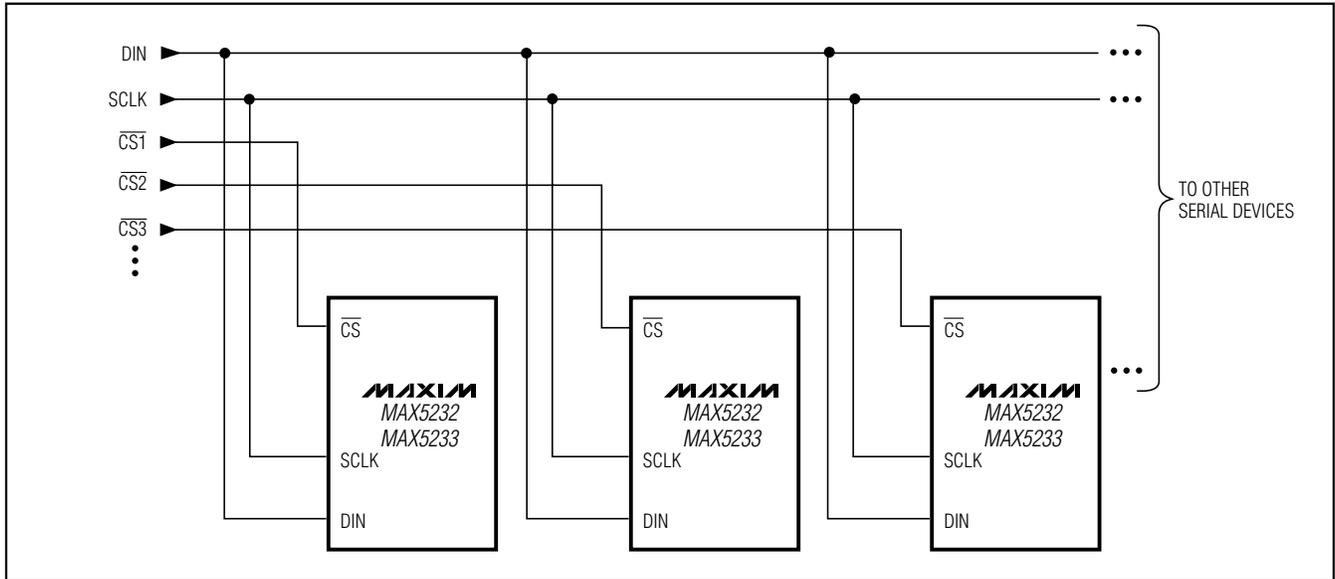
Figure 9. Multiple MAX5232/MAX5233s Sharing a Common DIN Line
