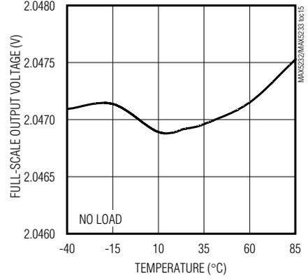
**FULL-SCALE OUTPUT VOLTAGE vs. TEMPERATURE (MAX5233)**
