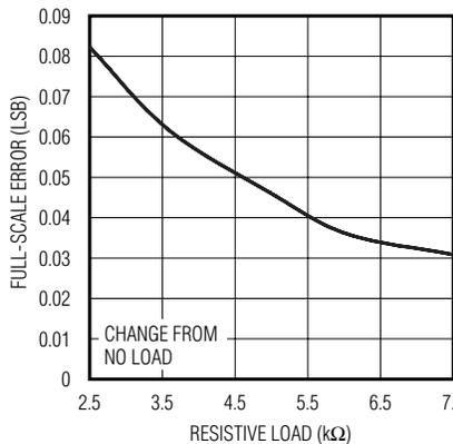
**FULL-SCALE ERROR vs. RESISTIVE LOAD (MAX5233)**
