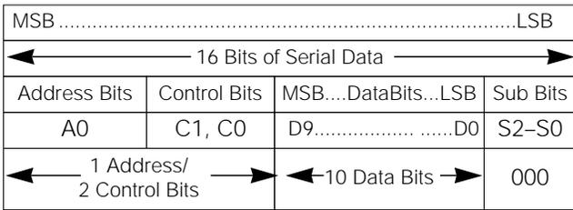
Figure 4. Serial-Data Format
