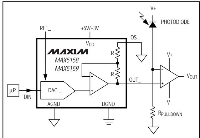
Figure 13. Digital Calibration
