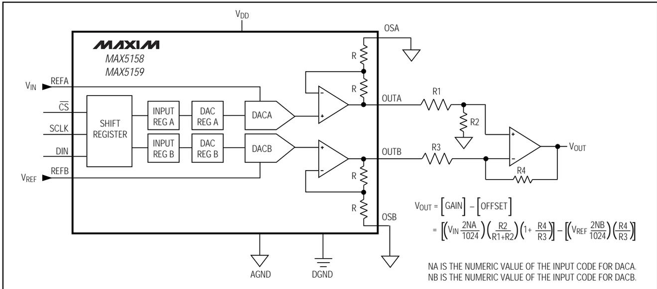
Figure 14. Digital Control of Gain and Offset
