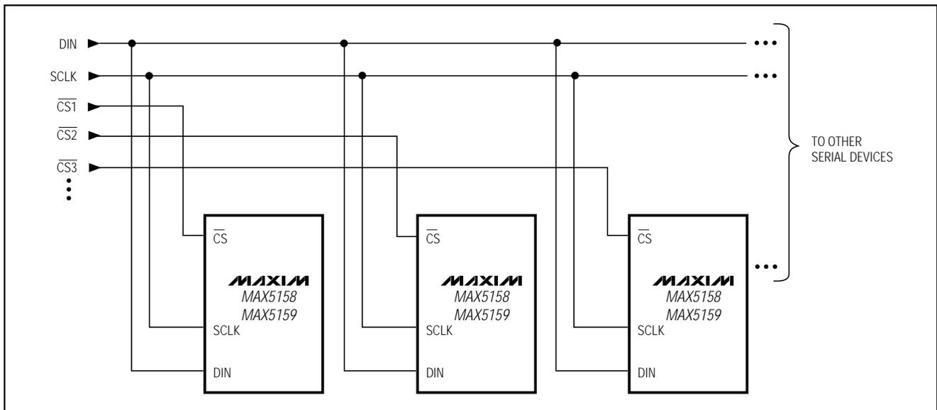
Figure 8. Multiple MAX5158/MAX5159s Sharing a Common DIN Line
