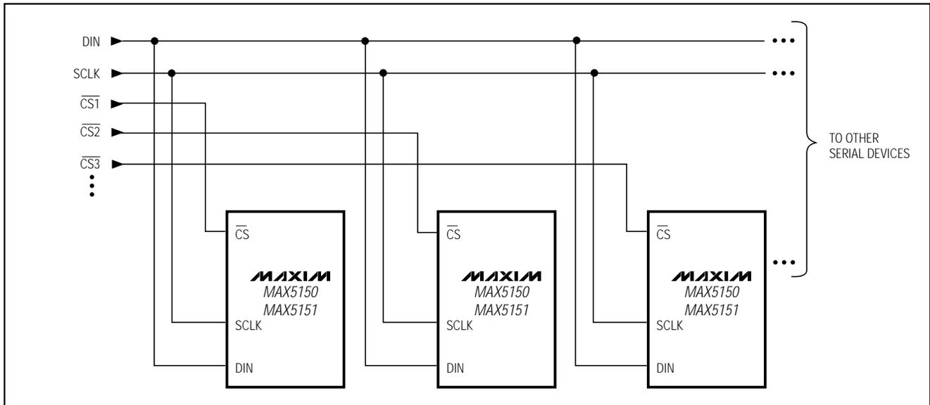
Figure 8. Multiple MAX5150/MAX5151s Sharing a Common DIN Line
