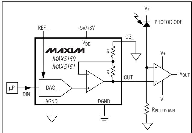
Figure 13. Digital Calibration
