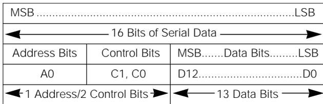
Figure 4. Serial-Data Format
