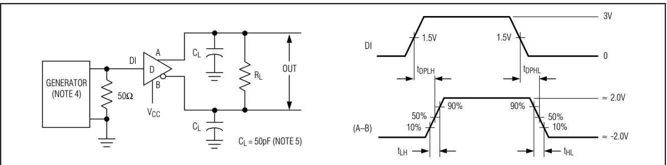
Figure 4. Driver Differential Output Delay and Transition Times
