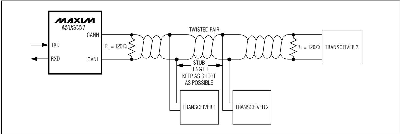
Figure 6. Multiple Receivers Connected to CAN Bus
