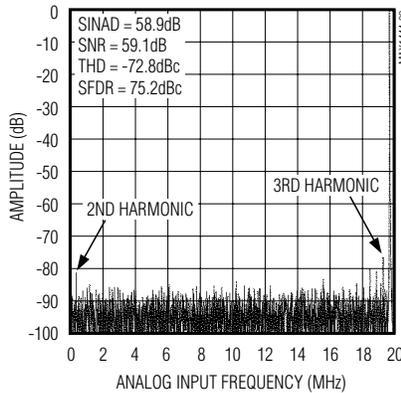
**FFT PLOT ( $f_{IN} = 47MHz$ , 8192-POINT FFT, DIFFERENTIAL INPUT)**
