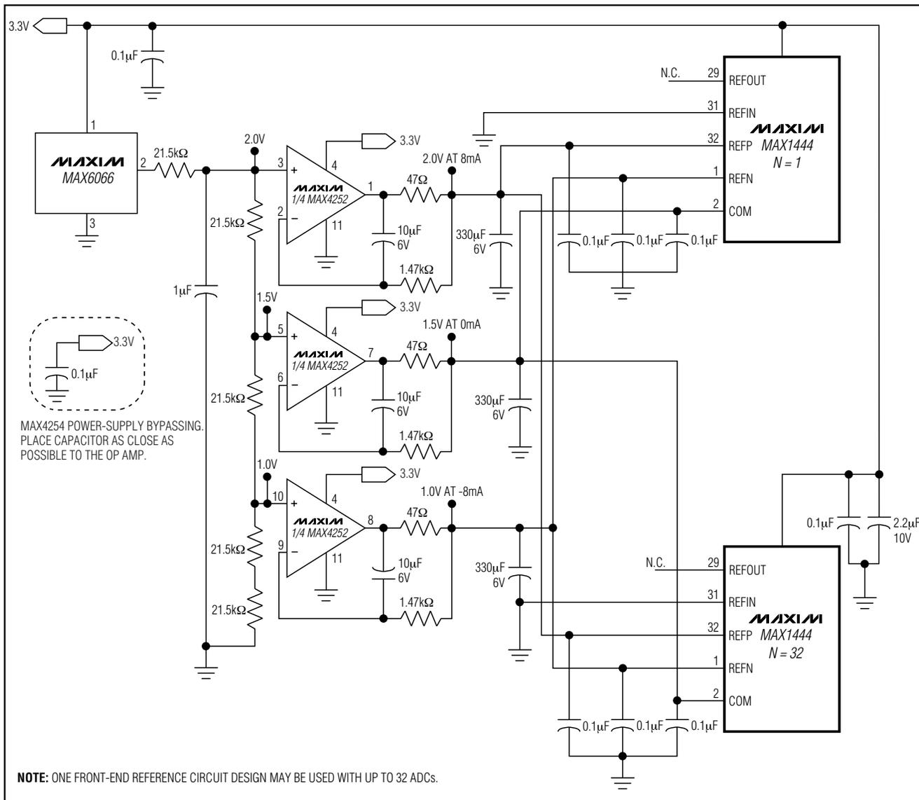
Figure 11. Unbuffered External Reference Drives Up to 32 ADCs
