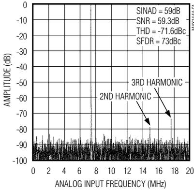
**FFT PLOT ( $f_{IN} = 19.91MHz$ , 8192-POINT FFT, DIFFERENTIAL INPUT)**
