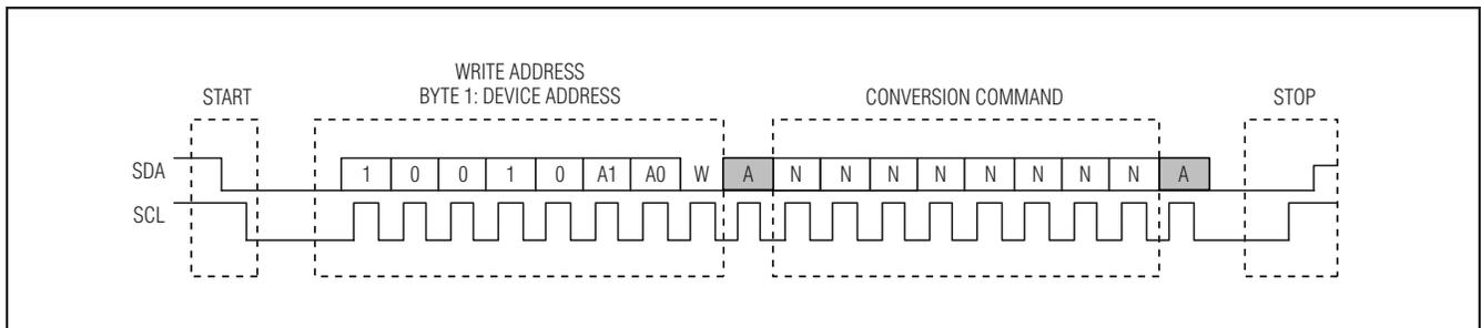
Figure 26. I<sup>2</sup>C Conversion Command
