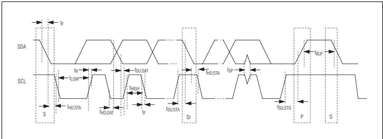
Figure 1. I<sup>2</sup>C Timing Diagram
