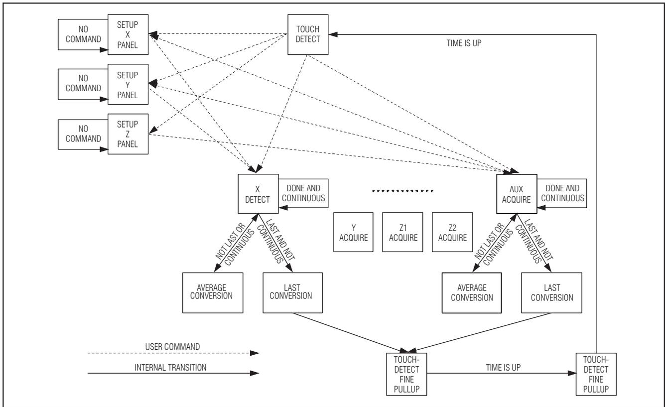
Figure 8. State Machine Transitions (Direct Conversion Mode)
