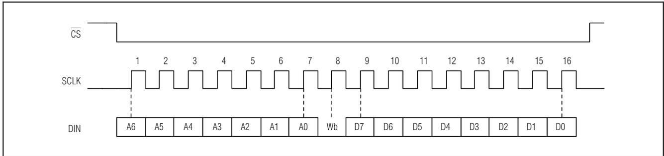
Figure 17. SPI Single Configuration Register Write Sequence
