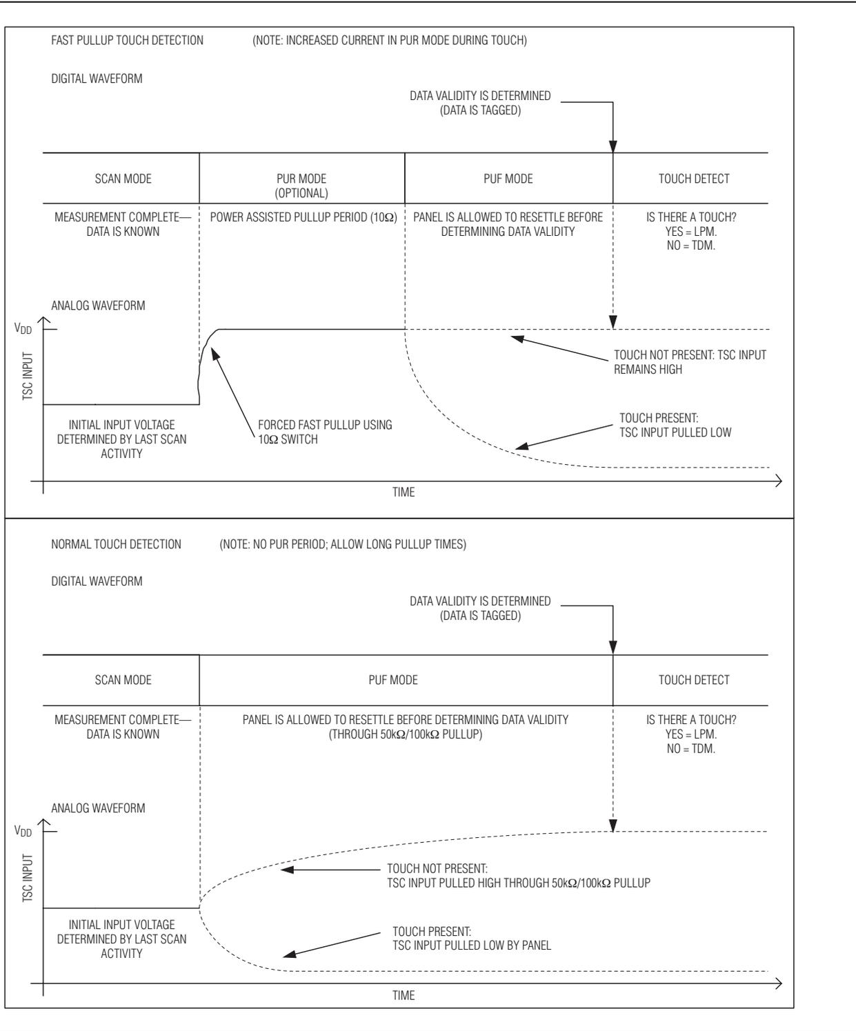
Figure 7. Touch-Detection Operations
