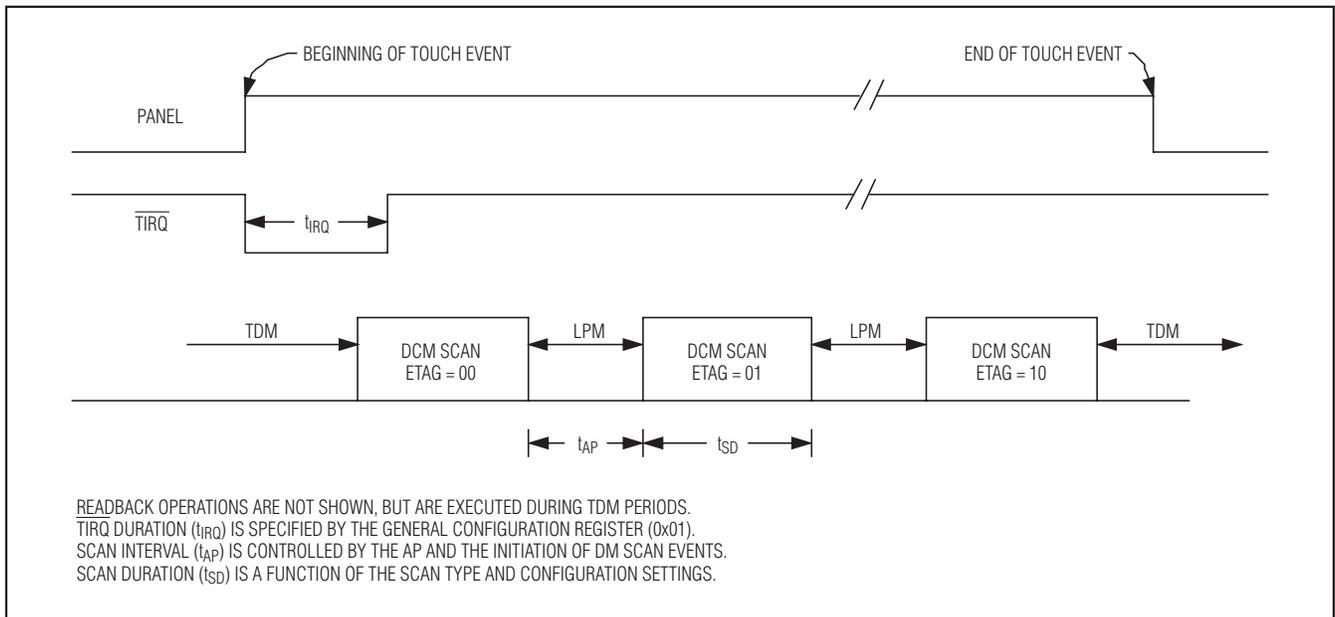
Figure 10. Edge Interrupt Mode (Direct Conversion Mode)
