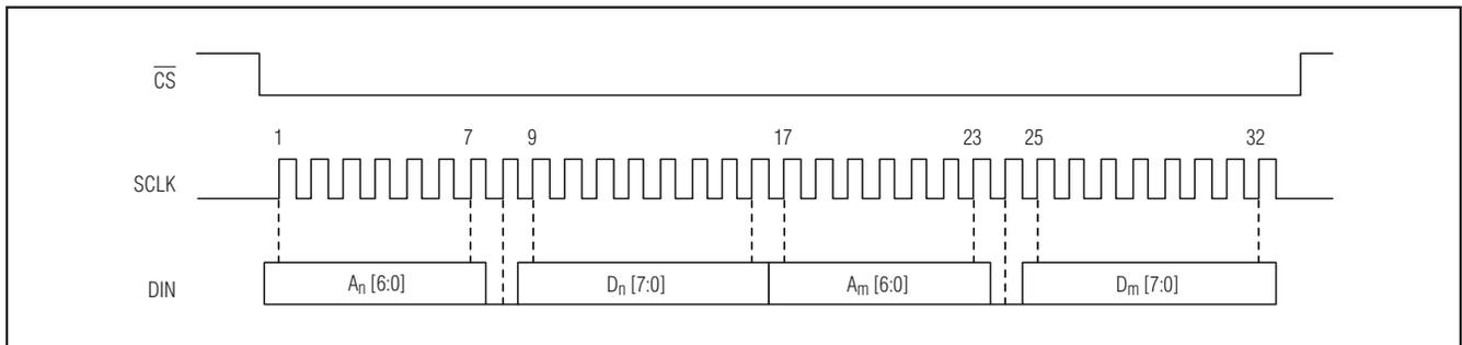
Figure 18. SPI Multiple Configuration Register Write Sequence
