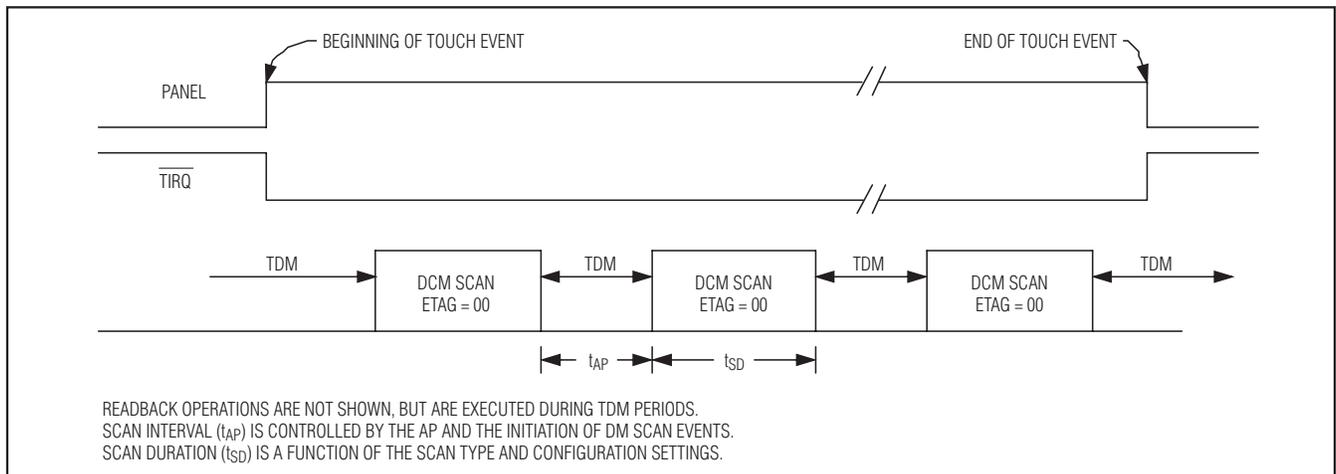
Figure 9. Continuous Interrupt Mode (Direct Conversion Mode)
