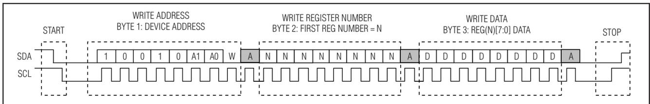
Figure 22. I<sup>2</sup>C Single Register Write Sequence
