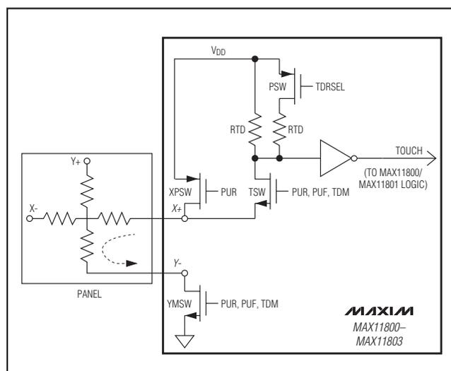
Figure 6. Touch-Detection Circuitry
