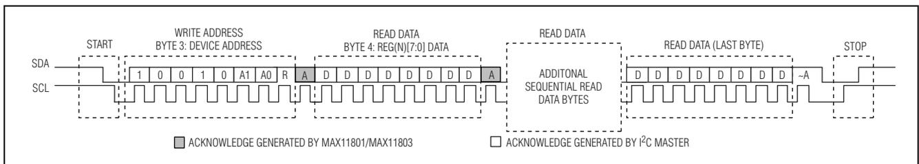
Figure 25. I<sup>2</sup>C Streamlined Register Read Sequence
