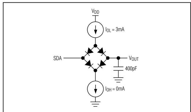
Figure 2. Load Circuit
