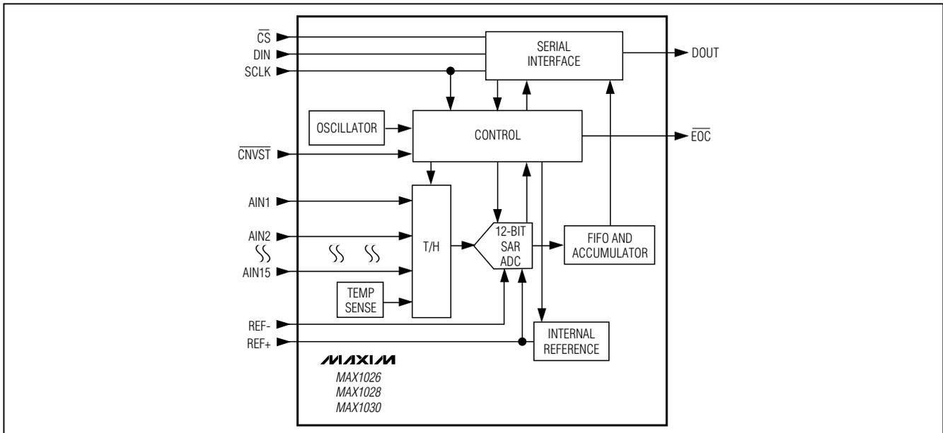
Figure 2. Functional Diagram
